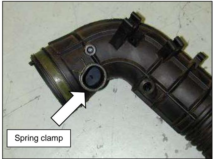
k. Remove spring clamp from stock inlet tube.
