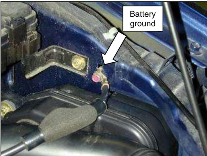
a. Remove bolt for battery ground.
