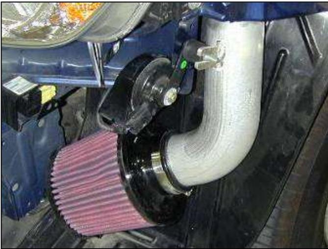
j. Install the lower pipe bracket onto the 8mm rubber mount. Install the air filter and secure with a hose clamp. Adjust the intake pipes so they do not come in contact with any part of the vehicle. Tighten the connecting clamps, 8mm washer and nylok nut. Check the fender liner and air filter and ensure there is about 1/8"-1/2" clearance.
