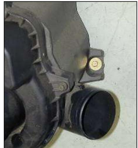
j. Loosen 1 bolt on the right side of the air box.
