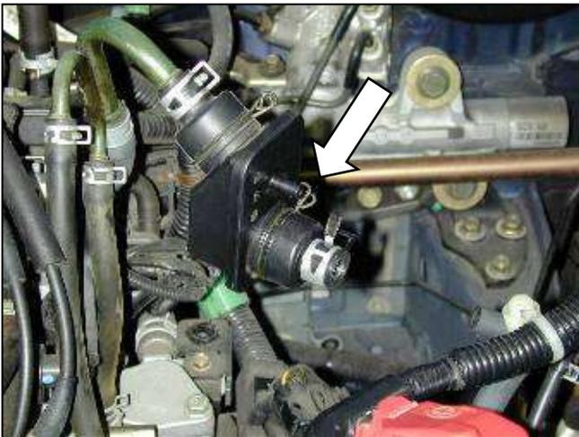
l. Attach the supplied oil trap coupler to the oil trap and secure with the clamp from step 2e.
