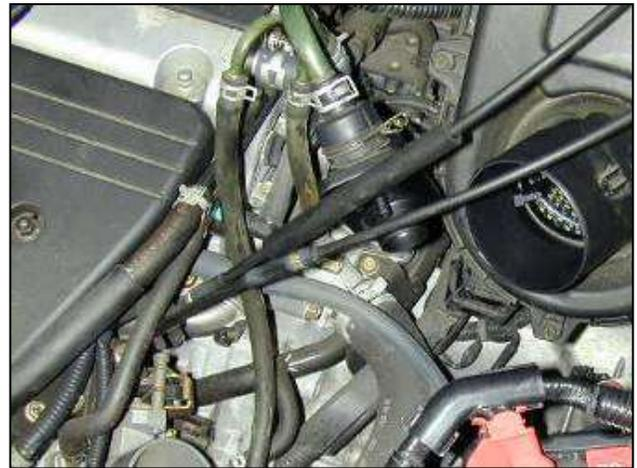
h. Remove the stock inlet tube.
