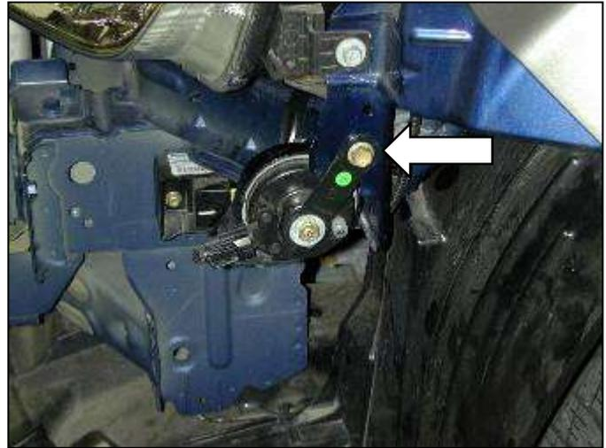
c. Remove 8mm bolt that secures the horn to the chassis.
