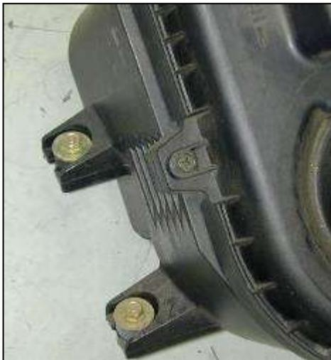
i. Loosen 2 bolts on the left side of the air box.
