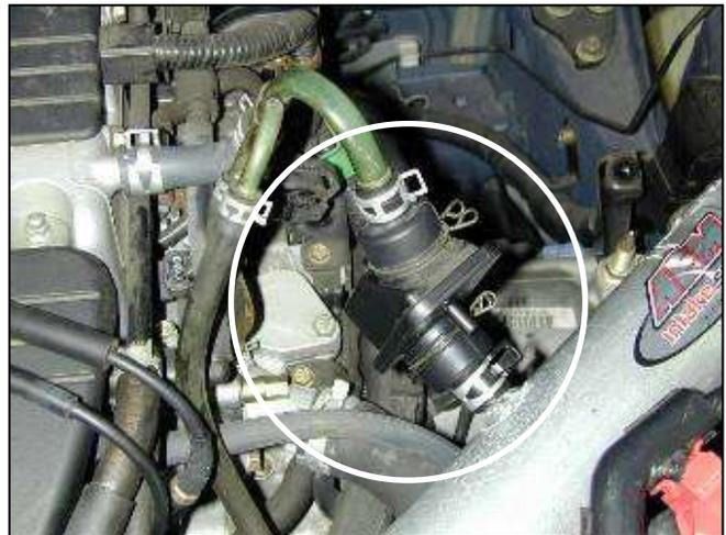
m. Secure the oil trap coupler to the nipple on the intake pipe with the provided spring clamp.
