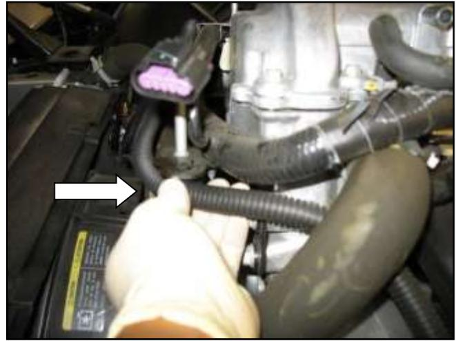
j. Remove the tree mount wire tie from the engine bracket.
