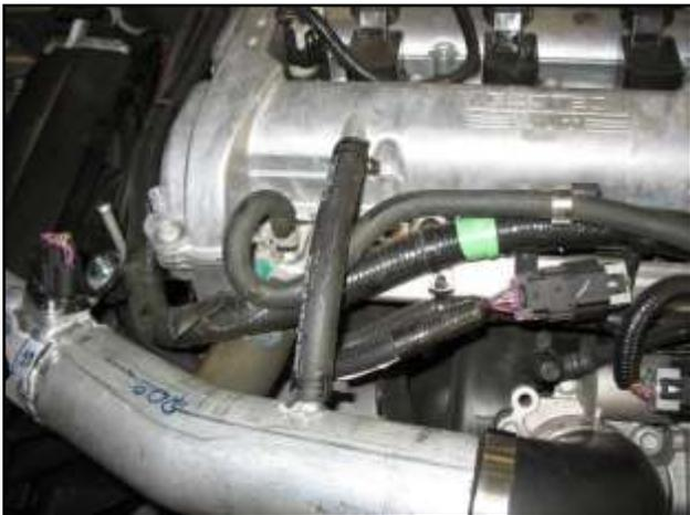
f. Insert the intake pipe into the coupler at the throttle body. Attach the supplied breather hose and secure with the factory spring clamps.
