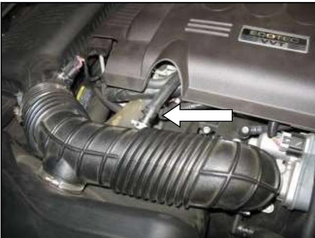
b. Unclasp the spring clamp. Remove the PCV breather hose from the inlet tube.
