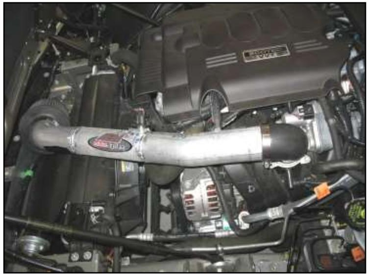
AEM® intake system installed
