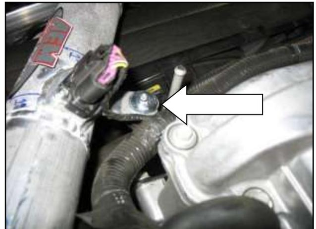
g. Align the bracket with the rubber mount. Secure with the M6 washer and M6 serrated nut. Reconnect the MAF sensor wire harness connector.
