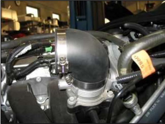
d. Attach the coupler at the throttle body as shown. Secure with the #44 hose clamps.
