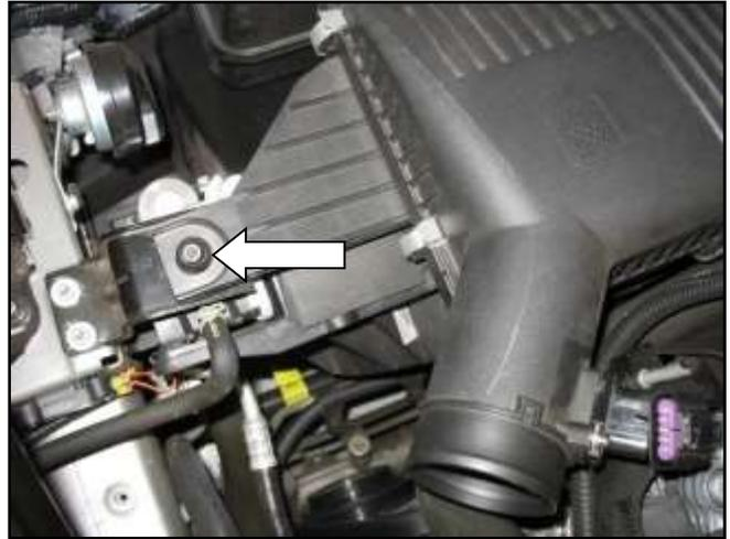
f. Loosen the air box mounting bolt.
