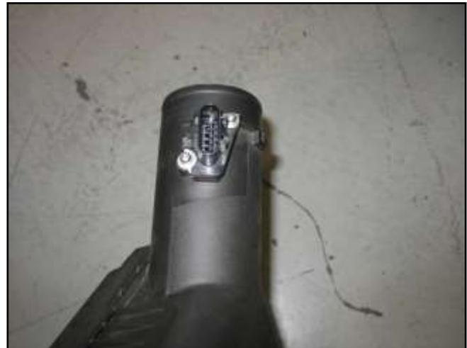
c. Remove the MAF sensor from the stock air box. The mounting screws will be reused.
