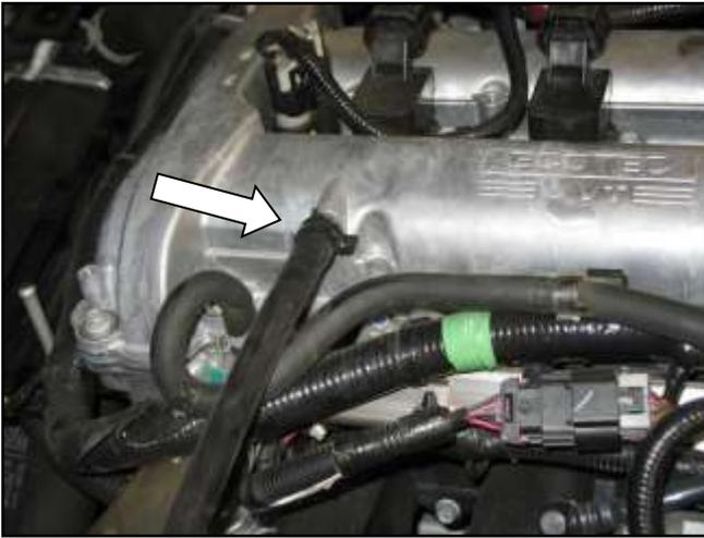
i. Remove the breather hose by unclamping the spring clamp. Both clamps will be reused.
