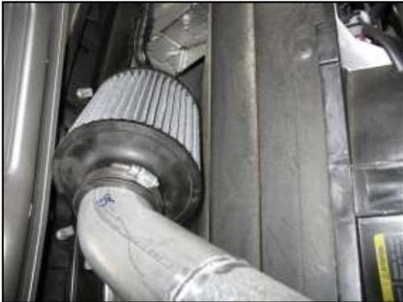
h. Attach the air filter element as shown and secure with the #48 hose clamp. Check for clearance against the radiator shroud. Attach filter sock to protect against the elements.
