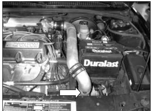
g. Make sure the intake pipes clear the battery and the clutch master cylinder before tightening the hardware. Install the supplied grommet in the hole on the lower inlet pipe. Install the IAT sensor in the inlet pipe, then reconnect the IAT wire harness connector to the IAT sensor.
