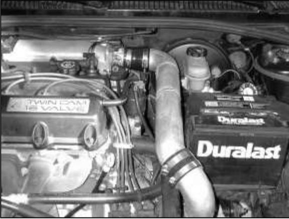
AEM<sup>®</sup> intake system installed
