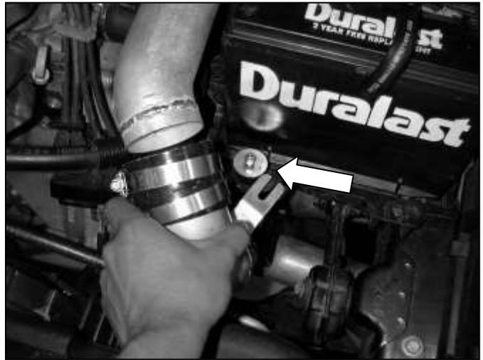
b. Insert the upper inlet pipe with the provided stepped coupler and hose clamps.
