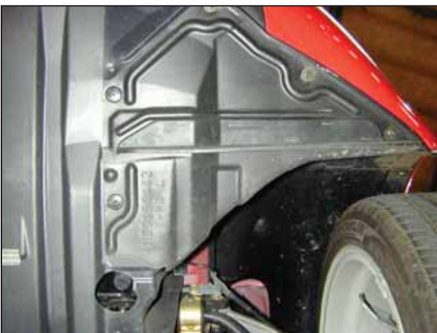
i. Remove the retaining clips and bolts securing the passenger side splash shield to the bumper and chassis. Remove the splash shield.
