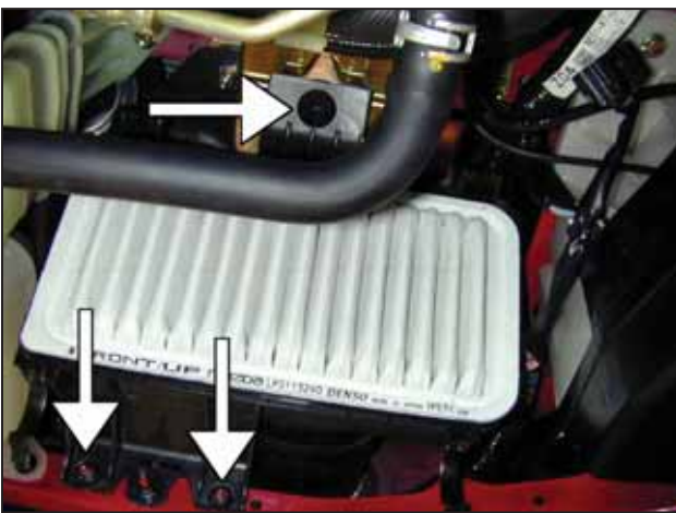
g. Remove the lower air filter housing and filter by removing the two nuts securing the housing to the chassis. Next, lift up on the back side of the housing and remove it from the vehicle.
