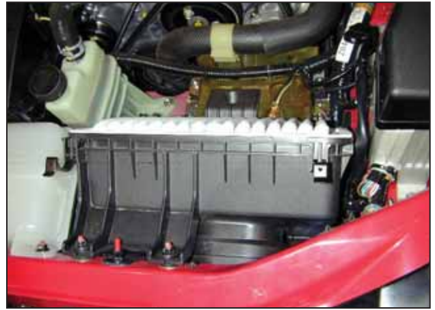
f. Remove the air filter housing lid by unhooking the metal retaining clips and sliding the lid out.
