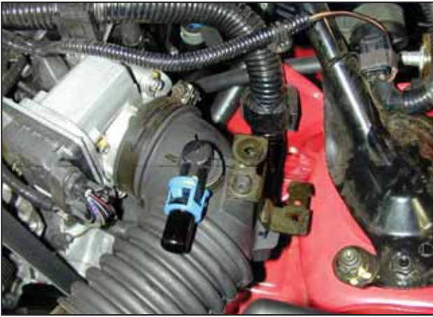
e. Unscrew the inlet tube from the throttle body and the air filter housing. Remove the inlet tube.
