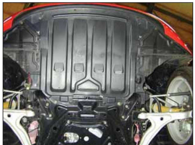
j. Remove the clips and bolts securing the center splash shield to the front bumper.
