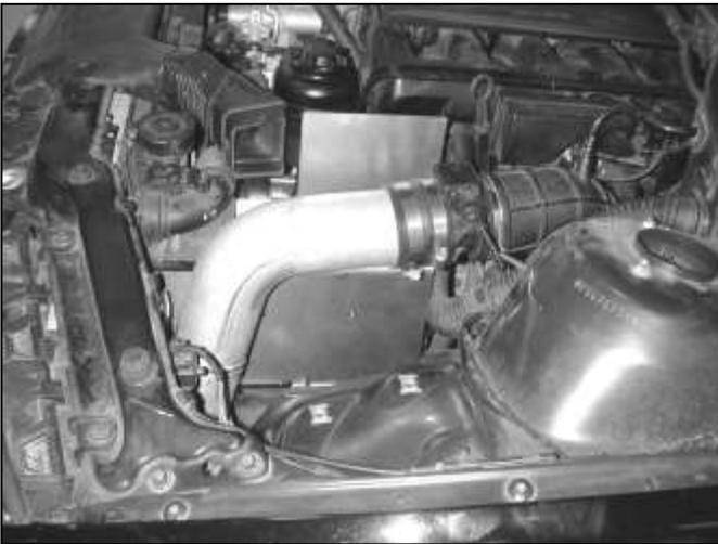
f. Insert inlet pipe into the silicon coupler
