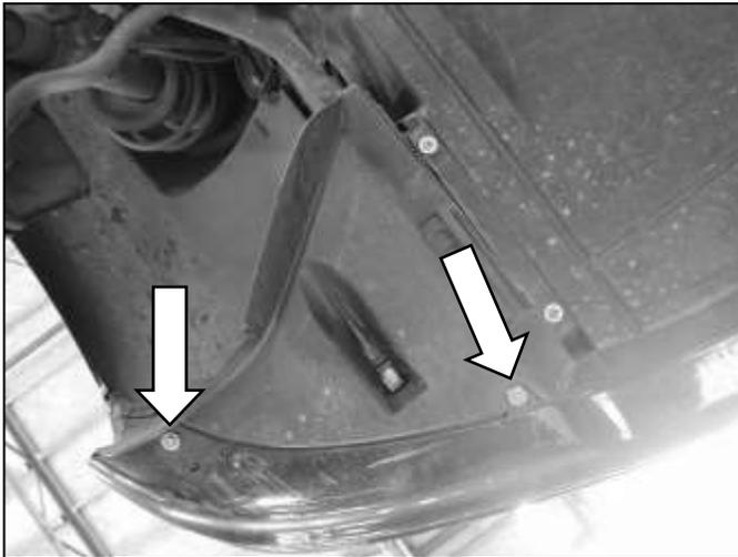
g. Loosen and remove the 2 bolts on the edge of the bumper.
