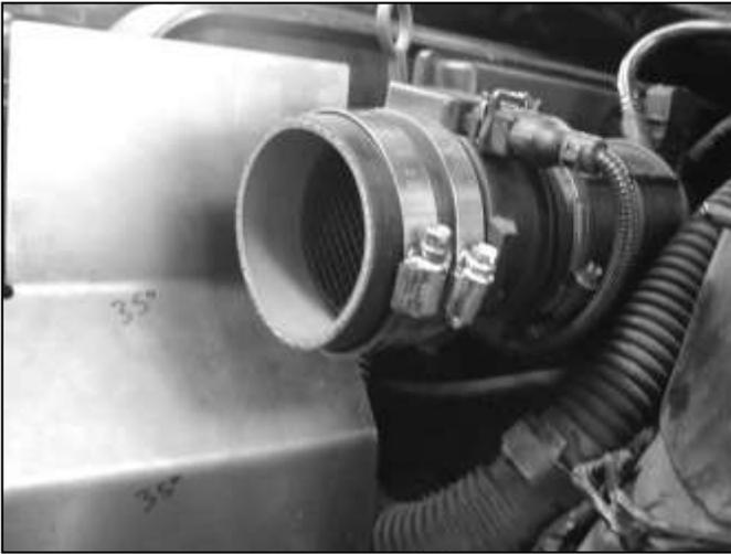
d. Attach coupler with supplied hose clamps.
