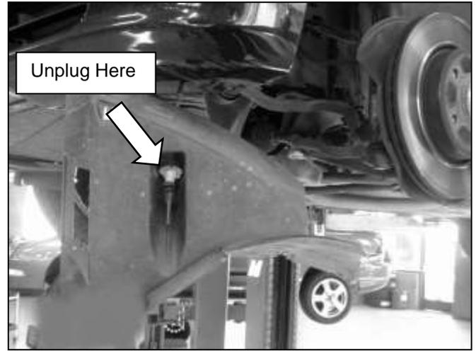
h. Gently pull down the lower splashguard. Unplug the outside temperature sensor. Remove the sensor and splashguard.
