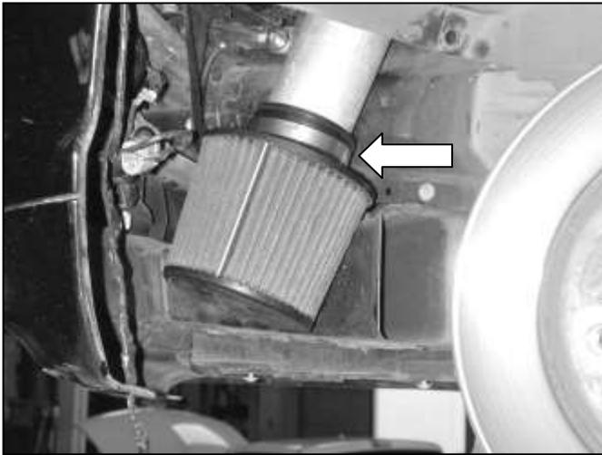
h. Attach the air filter. Secure with provided hose clamp.
