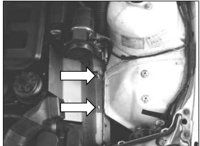
c. Insert the heat shield. Secure with washers and nylok nuts.
