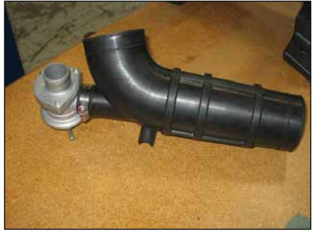
i. Install the air bypass valve into the rubber inlet hose and secure with the OE hose clamp.
