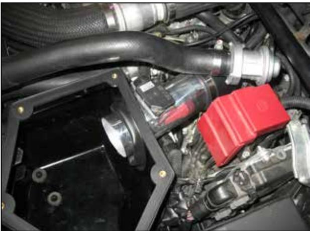
p. Reconnect the bypass hose to the bypass valve and secure it using the OE hose clamp.
