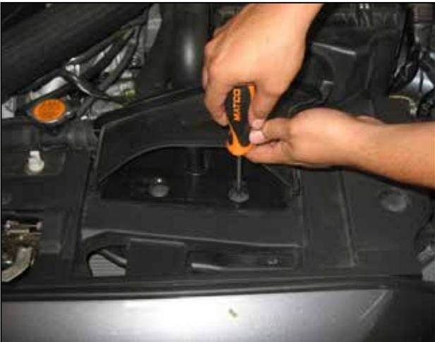
g. Remove the two plastic rivets securing the air inlet duct.
