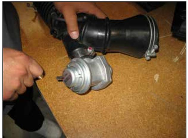
p. Remove the air bypass valve from the inlet hose by loosening the hose clamp on the inlet tube.
