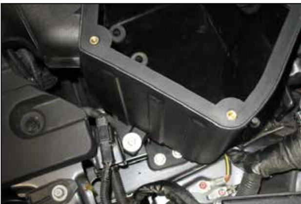
f. Align the air box tab with the mount the OE air box mounted to. Secure the air box to the mounting tab with the bolt removed in step 2d. Do not over torque the bolt, 15 ft-lbs.
