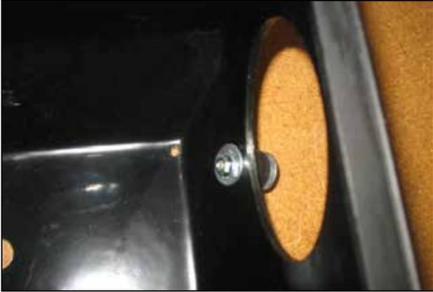
b. Install the supplied rubber mount onto the air box and secure it with a washer and lock nut.
