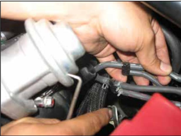
m. Disconnect the two vacuum lines that connect to the wastegate solenoid, they connect to the inlet tube.
