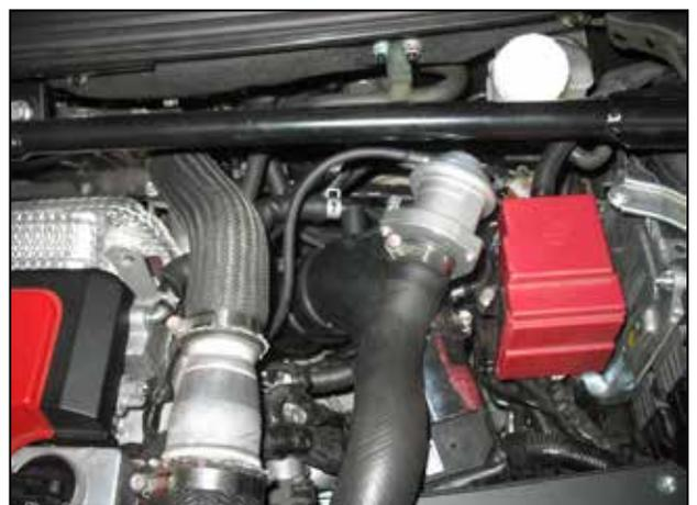
s. Using the 1/4" hose and the hose clamps (4093-3), secure the hose to the bypass valve nipple and the vacuum tube (exposed in step 2o).
