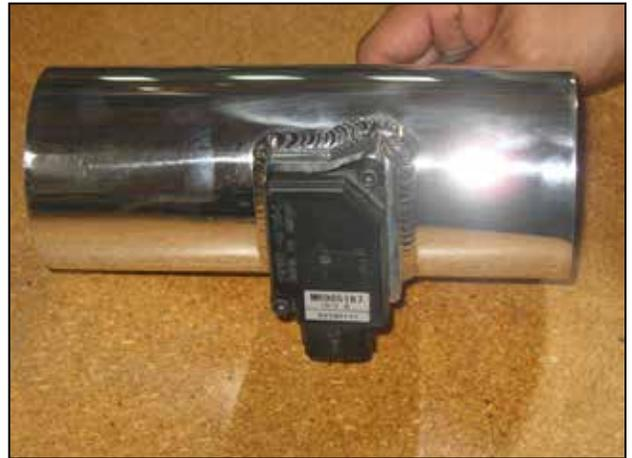
k. Install the MAF sensor to the intake pipe and secure with the supplied socket bolts.
