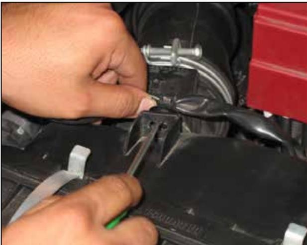
c. Using a small screwdriver remove the two tree mount zip ties from the air box housing tabs.
