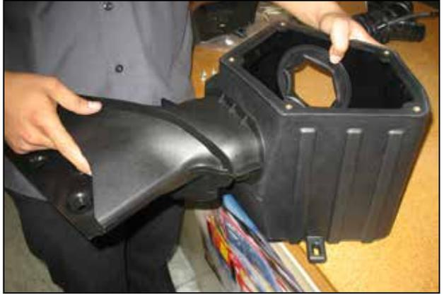
c. The inlet duct should snap into place in the oval opening of the air box. Also, install the edge trim around the inlet hole on the rear side of the air box.
