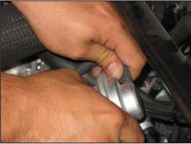
k. Disconnect the vacuum line from the air bypass valve.
