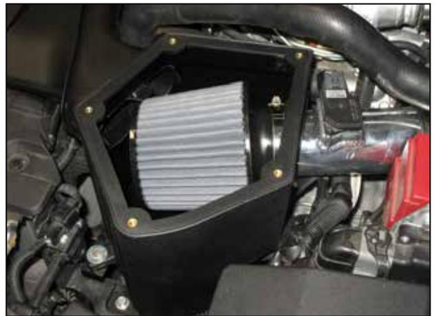
q. Install the AEM® air filter onto the end of the intake pipe and secure it with hose clamp (9452). Reconnect the MAF sensor harness connector to the MAF sensor.
