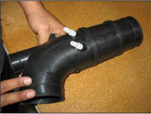
h. Insert the two white connectors into the rubber inlet hose.
