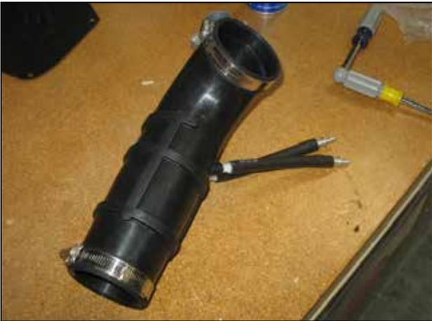
j. Insert the two aluminum connectors into each of the 5/16" hoses. Connect the 5/16" hose to the white connectors attached to the rubber inlet as shown.
