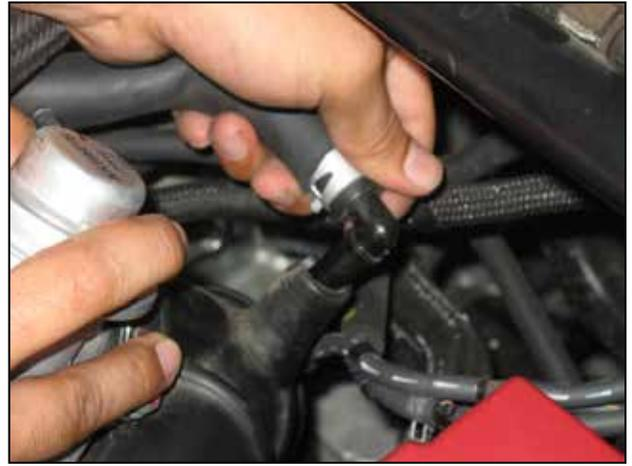
l. Disconnect the PCV hose from the OEM inlet tube.
