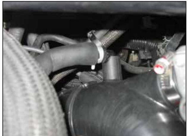
m. Install the PCV hose into the rubber inlet hose.
