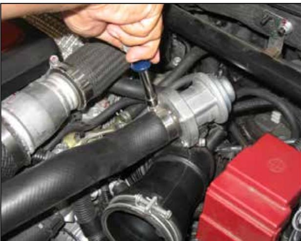
i. Disconnect the air bypass valve hose from the air bypass valve.
