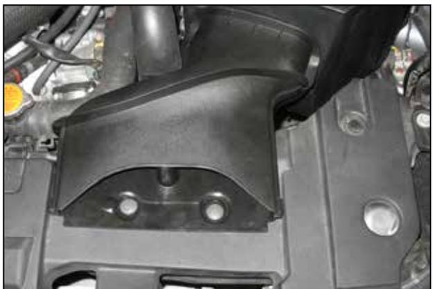
g. Secure the inlet duct using the plastic rivets removed in step 2g.
