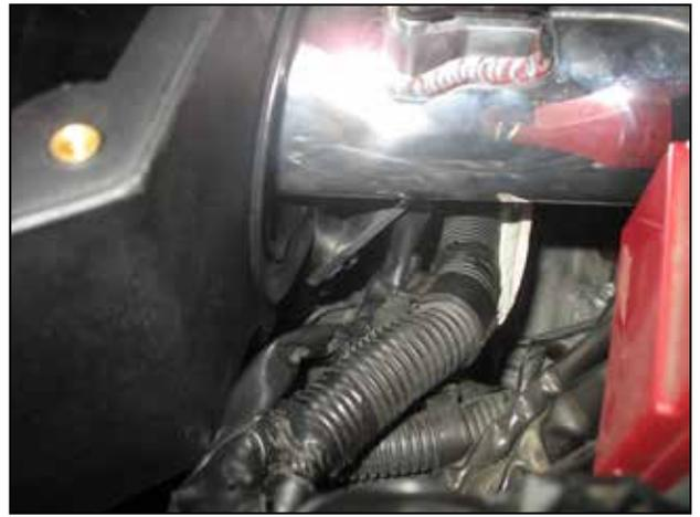
o. Install the aluminum intake pipe into the rubber inlet hose. Align the intake pipe's bracket to the rubber mount, then secure the intake pipe to the rubber inlet hose with hose clamp (9448).
