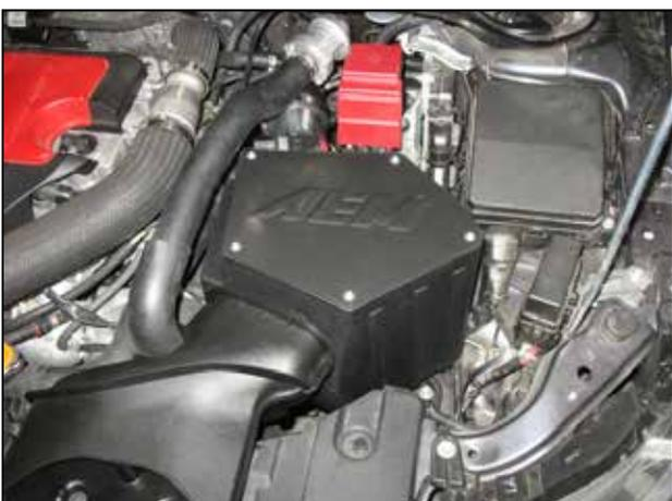
r. Align the holes of the aluminum air box lid with the threaded holes of the air box. Install 5 button head screws and plastic washers to secure the lid to the air box.
