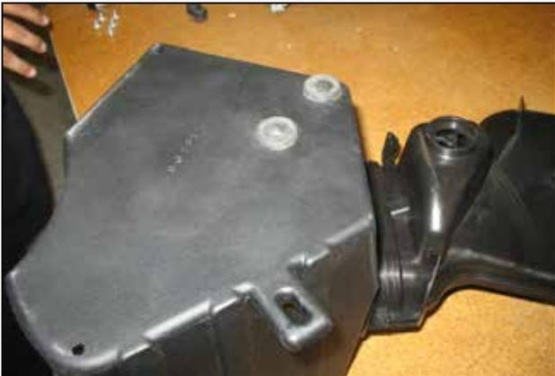
d. Install the two OE rubber grommets onto the bottom of the AEM® air box. The grommets were removed from the stock air box in step 2u.
