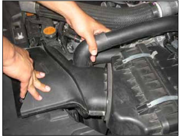
f. Remove the air bypass valve hose from the OE inlet by pulling it toward the passenger side of the vehicle.
