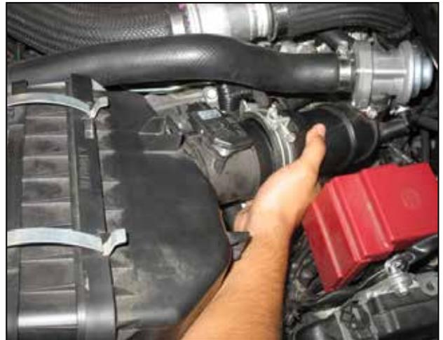
h. Disconnect the OE inlet tube from the air box, then remove the air box from the engine bay by pulling straight up.
