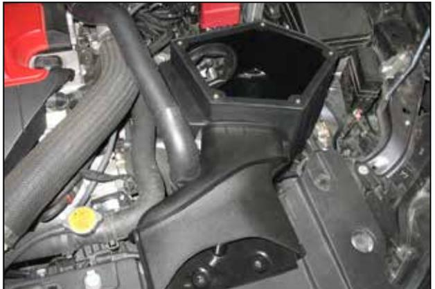
e. Place the AEM® air box in the engine bay, aligning the two rubber grommets of the air box with the two dowels protruding from the mounting location. Install bypass hose back into the clip.
