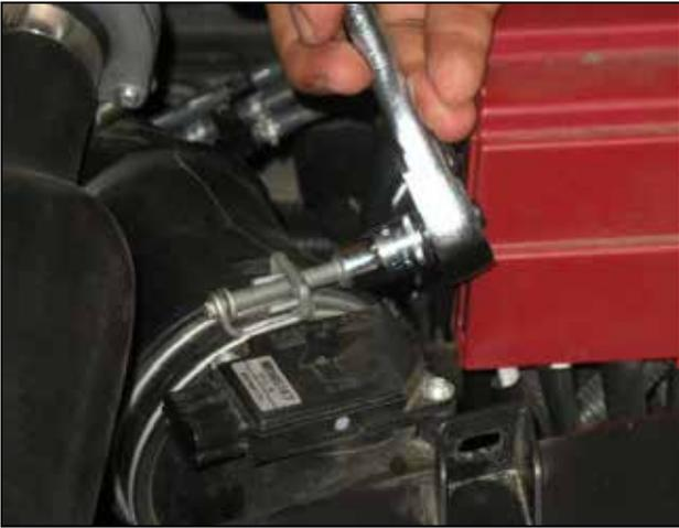
e. Loosen the hose clamp securing the rubber inlet tube to the stock air box assembly.
