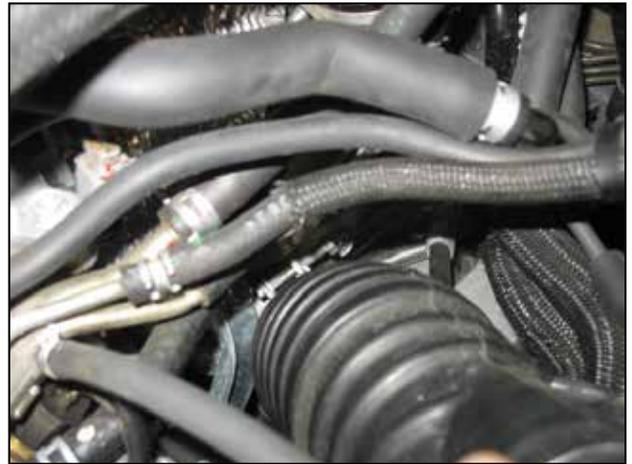
n. Loosen the hose clamp securing the inlet tube to the turbo inlet. Remove the inlet tube.
