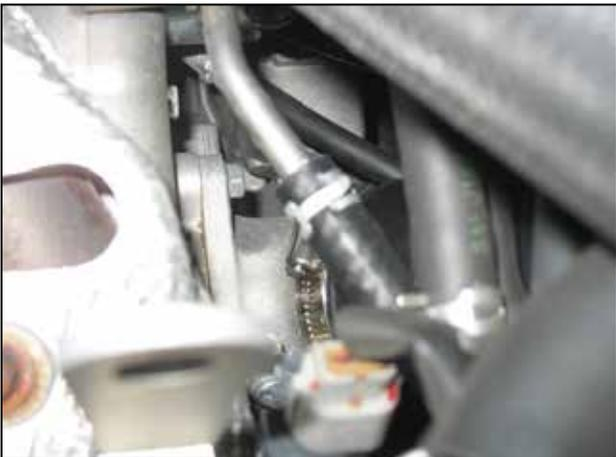
l. Install the rubber inlet into the vehicle, positioning the air bypass valve toward the top of the engine. Loosely secure the inlet to the turbo inlet with a hose clamp (9444).
