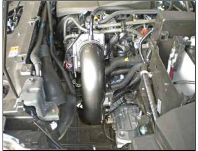
e. Install the upper intake pipe into the coupler installed earlier in step 3b. Reattach the MAF harness connector to the MAF sensor.
