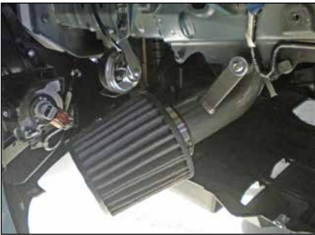
h. Attach the AEM® air filter onto the lower intake pipe. Once proper fitment is achieved, secure the air filter to the intake pipe with the provided hose clamp (# 9444).
