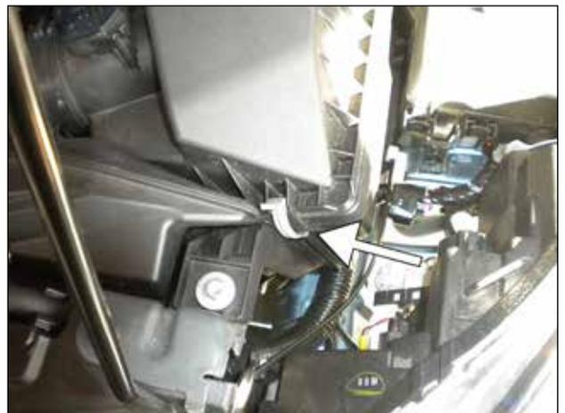
l. Unlatch the 2 metal retaining clips securing the air box lid.
