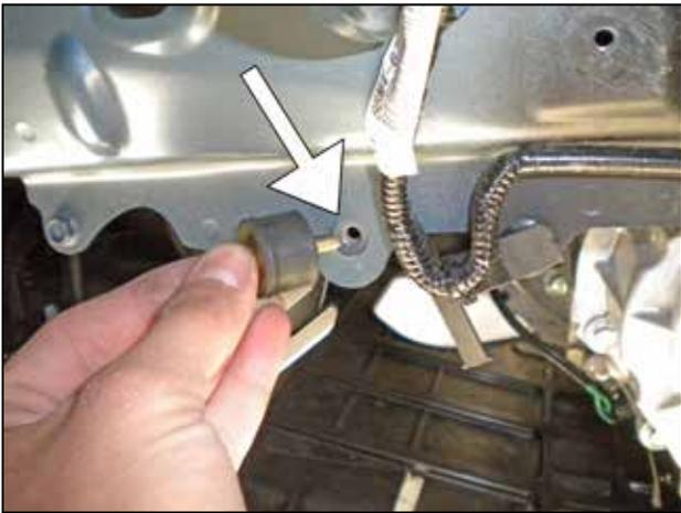
f. Install the threaded soft mount into the location shown.
