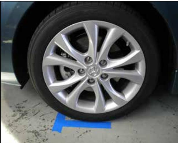
a. Remove the front driver side wheel from the vehicle.
