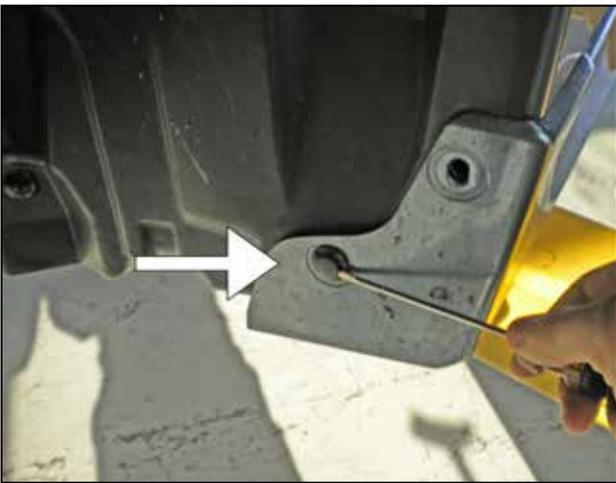
e. Remove the plastic wheel liner. This liner is held in by 16 plastic clips as shown. To remove the plastic clips use a Phillips end screw driver to remove the plastic screw in the center, then pull out the clip. A pick or flat blade screw driver can be used for popping out the two clips used in the bottom corner toward the rear of the wheel well.
