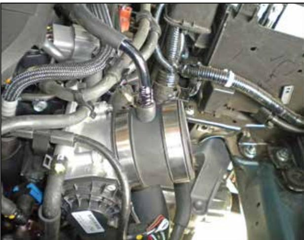
b. Install the coupler with the nipple onto the throttle body using the provided hose clamps (#9448).
