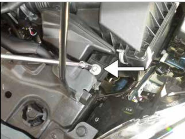
k. Remove the 10mm bolt securing the airbox to the core support.
