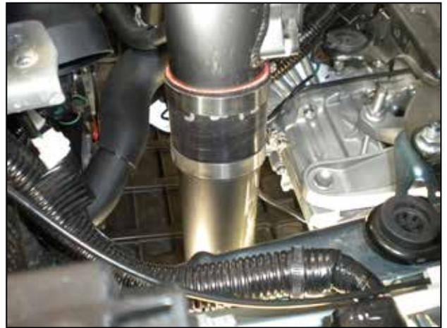
g. Use the 2.75"x3" coupler to attach the lower pipe to the upper pipe, using the supplied (#9448) hose clamps. Fasten the intake pipe bracket to the threaded soft mount with the supplied nut and bolt.
