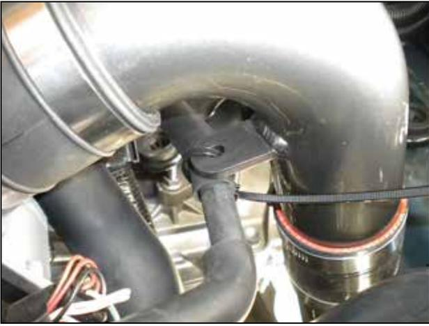
j. Coolant hose secured to the upper intake pipe's bracket.
