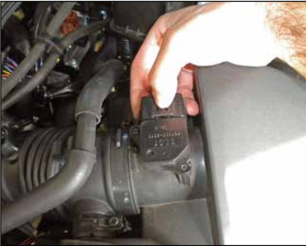
i. Remove the Mass Air Flow sensor harness by pressing down on the tab and pulling it off.
