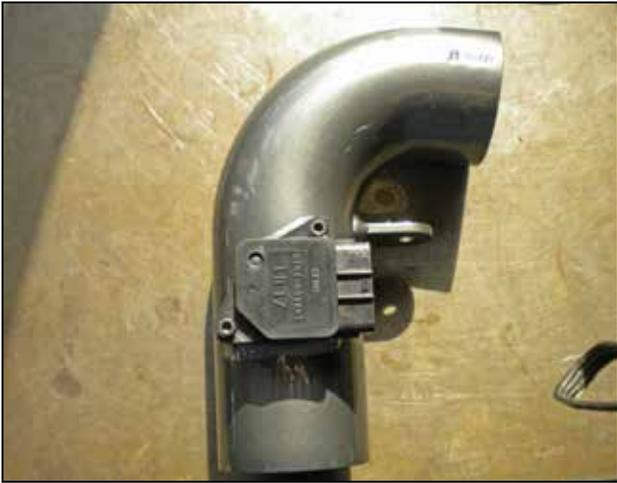
d. Install the MAF sensor into the upper intake pipe using the supplied bolts.
