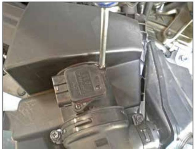
c. Remove the MAF sensor from the stock airbox assembly.
