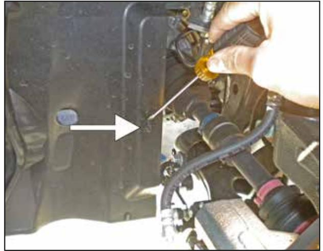
d. Undo the harness clip attached to the back side of the plastic cover.
