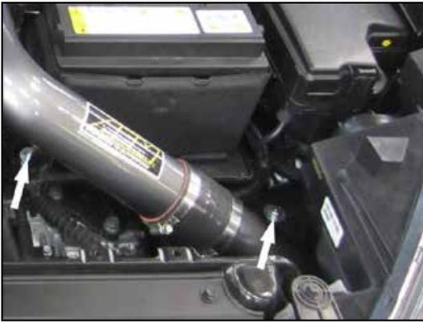
f. Use the provided hex nuts(H) and washers(G) to loosely fasten upper and lower tubes to the rubber mounts previously installed.
