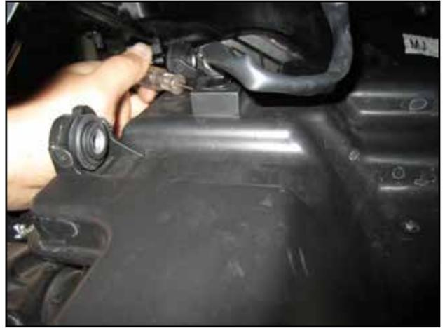
l. Carefully lower the intake resonator and disconnect the tree mount clip to detach the foglight harness. Set aside resonator chamber.
