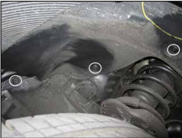
g. With the vehicle raised, remove the three plastic clips in the driver side front wheel well as indicated above.
