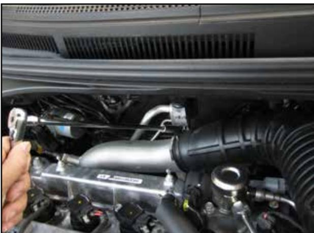
c. Loosen the stock hose clamp on turbo inlet using a 10mm socket and ratchet.
