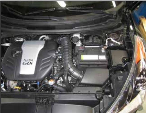
a. Stock intake system. Remove the engine cover by grasping firmly on lower end and carefully lifting up.
