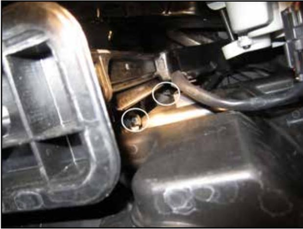
k. From underneath vehicle, remove the remaining two M6 bolts securing the lower intake resonator.
