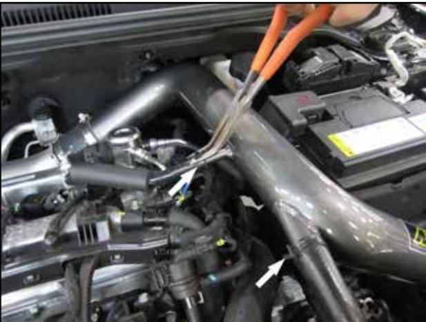
h. Reconnect crank case breather hose and recirculation valve hose to upper tube(A) and fasten using stock spring clamps as shown.
