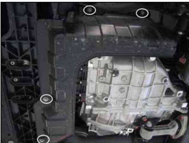
i. Remove four silver M6 bolts securing lower plastic belly pan cover.
