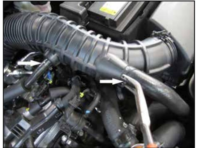
b. Loosen spring clamps to detach crank case breather hose and recirculating valve hose from intake tube.
