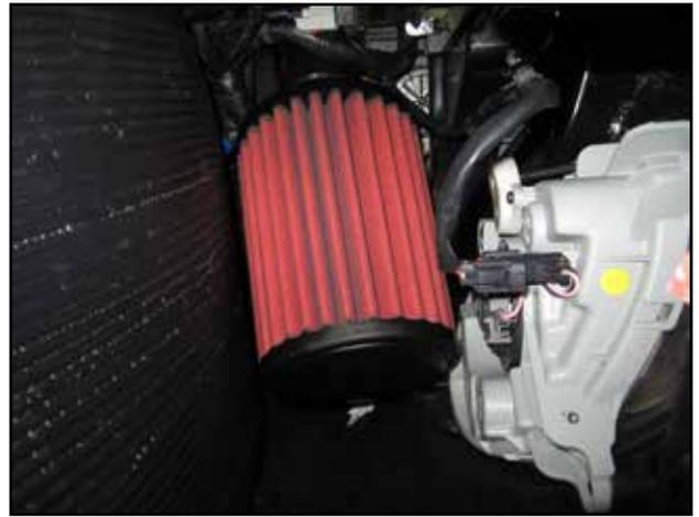
g. Check for clearance around filter between fog light housing and also plastic liner. Adjust the position of the lower tube if necessary. Tighten hex nuts(H) and hose clamps(C) once filter is properly positioned. Reinstall lower belly pan cover and plastic well liner.
