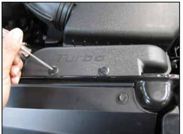
d. Remove the two plastic clips shown above and pull up on the air inlet snorkel to remove.
