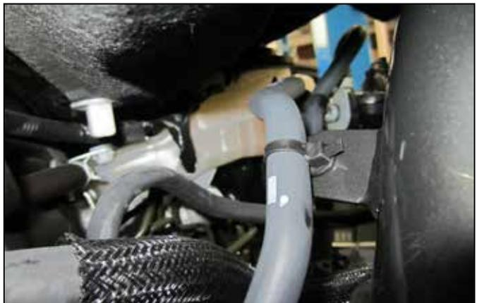
m. Fasten the VSV hose to the upper intake pipe using the provided tree mount zip tie, trim off excess.
