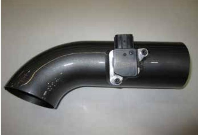
b. Install the MAF sensor onto the lower intake tube (K) using the provided M4 bolts (M), Tighten with an allen wrench.
