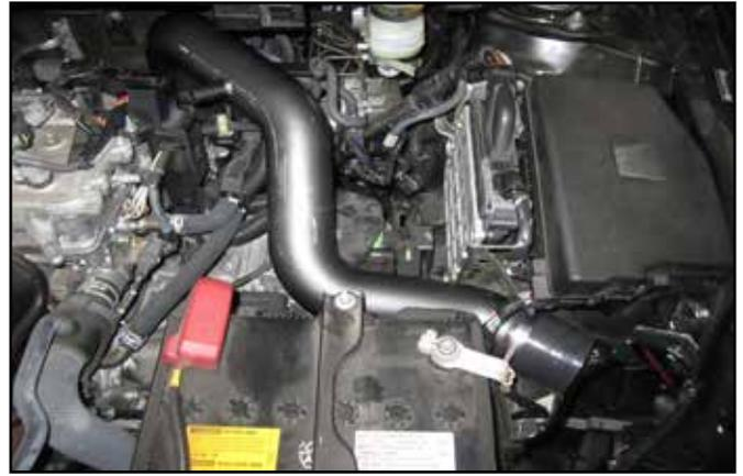
i. Maneuver the inlet side of the upper intake tube through the channel near the battery and under the wire harness. Pull back the plastic cover panel slightly and carefully slide the outlet side of tube towards throttle body. Insert the #48 hose clamp (I) over the coupler/ throttle body.
