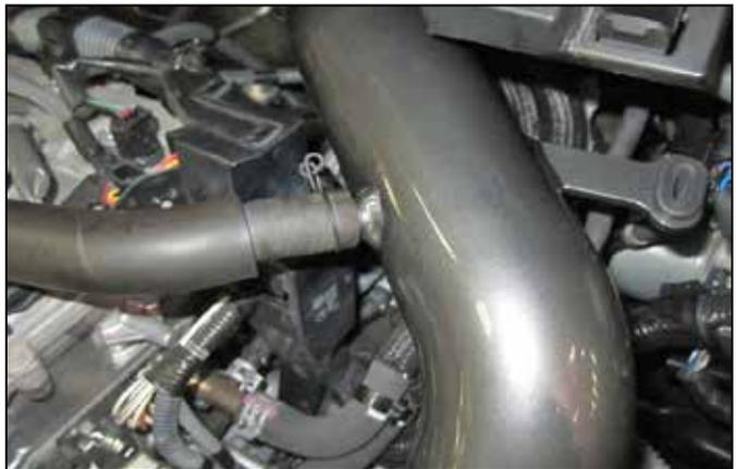
k. Connect the valve cover hose to the intake tube and secure with the stock spring clamp.
