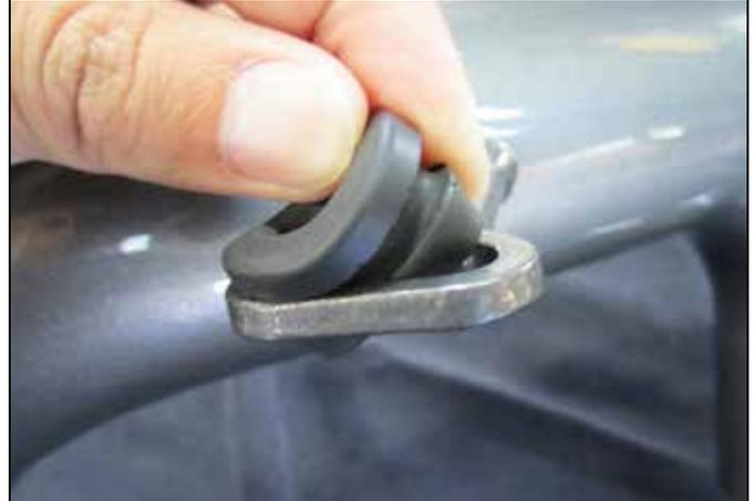
c. Insert the rubber grommet (D) into the VSV bracket as shown.
