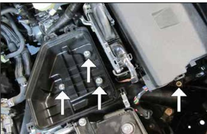
i. Remove the stock air filter. Loosen and remove the 3 bolts securing the lower airbox using a 10mm socket. Also loosen and remove the bolt securing the inlet air tube in place using a 10mm socket.
