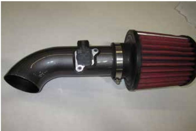
p. Install the DryFlow™ air filter (J) onto the lower intake pipe (K) using a #52 (N) hose clamp and tighten securely.
