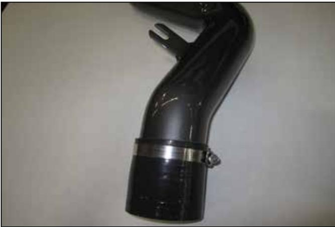
h. Install coupler (L) and hose clamp (H) on the upper intake tube.
