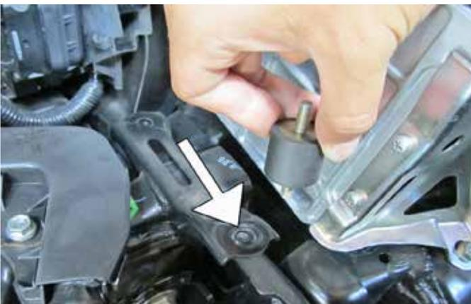
f. Install the set screw in the female side of the rubber mount with 3/8" left out. Then thread it into the location shown in the picture.
