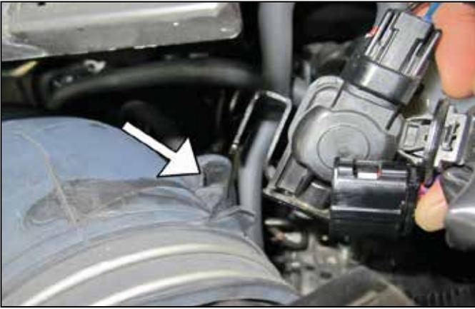
e. Unhook the vacuum switching valve (VSV) from the rubber inlet tube bracket.
