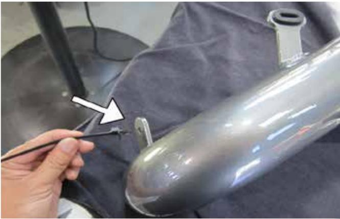
d. Insert the tree mount zip tie (C) into the bracket of the upper intake tube as shown.
