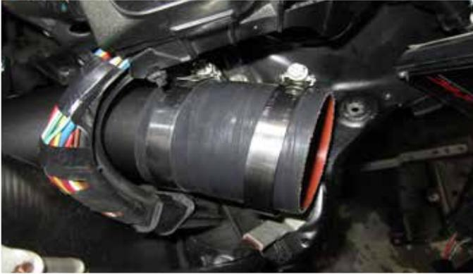
n. slide the additional #48 hose clamp (I) onto the coupler (L) .
