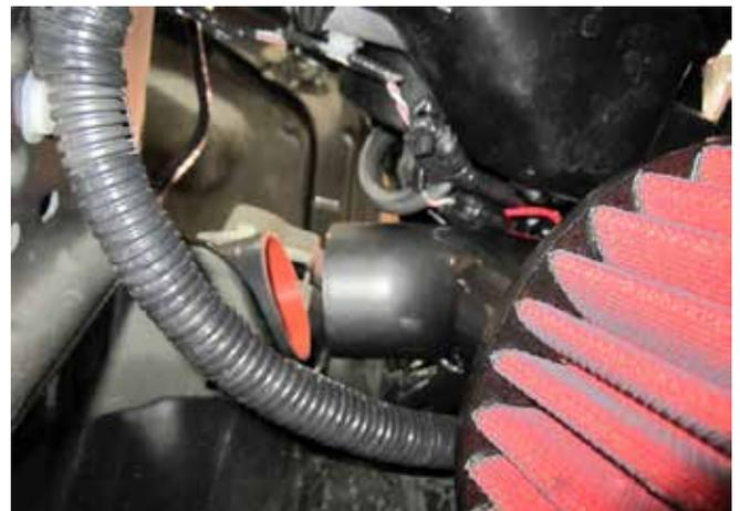
q. Pull the belly pan edge down and carefully slide the lower intake pipe through the opening. Slide the lower intake pipe into position to mount to the coupler attached to the upper intake pipe. Reinstall the 10mm bolt and plastic clip onto the belly pan, then lower the vehicle.
