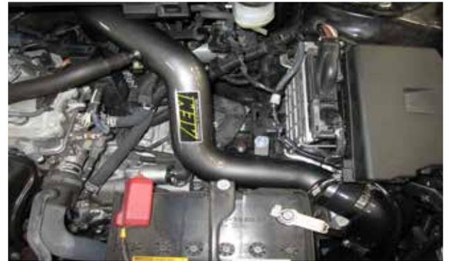
u. AEM® intake system installed.
