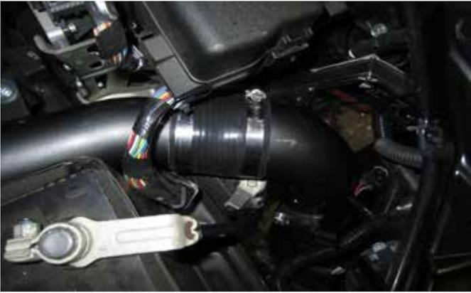
r. Attach the lower intake pipe (K) to the coupler and maneuver the intake pipe so the bracket slides into place. Check for clearance on the headlight housing and fog light housing (if applicable). Tighten all clamps and nuts once proper clearance is obtained.
