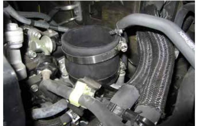
g. Install the reducer coupler (b) on to the throttle body using hose clamps (h) and (l).
