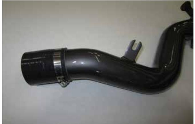
e. Slide coupler (L) onto the upper tube about 1-1/8th inch and fasten with #44 hose clamp (H)
