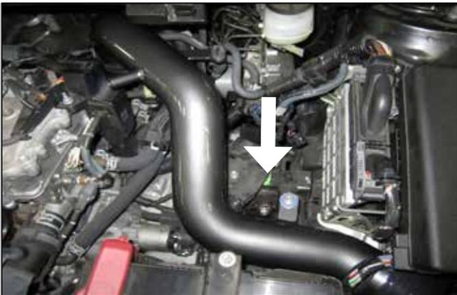
j. Position intake pipe (A) so the mounting bracket slides into position over the rubber mount, then loosely fasten with the provided washer (F) and M6 nut (G). Tighten the hose clamp to secure the intake tube to the throttle body.
