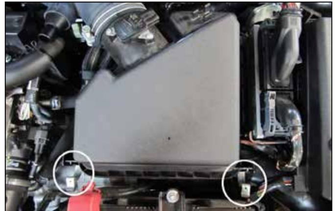
h. Locate the two clips securing the airbox lid next to the battery. Unhook the clips and slowly remove the airbox lid and tube assembly, ensuring the MAF wire harness, VSV, and VSV hose are not snagged during removal.
