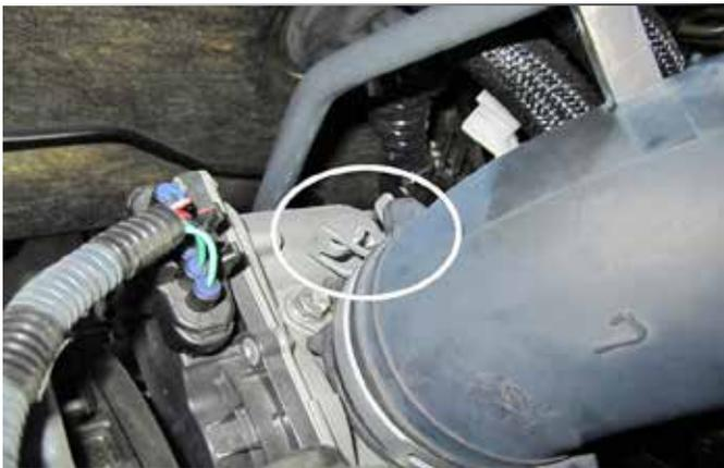
g. Use needle nose pliers to lock open the tube clamp securing the inlet tube to the throttle body. Carefully disconnect the inlet tube from the throttle body, ensuring the tube clamp does not snap back into the unlocked position.
