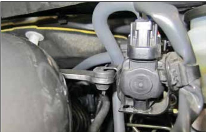
l. Slide the VSV bracket into the rubber grommet as shown.
