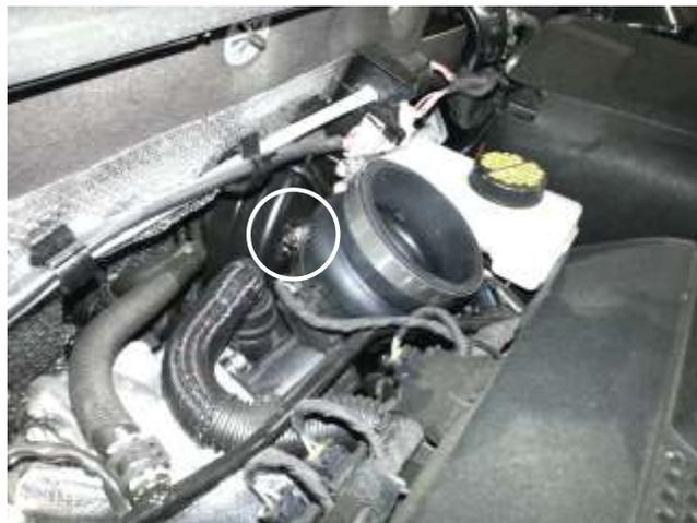
b. Install the hump hose and two hose clamps onto the compressor inlet and tighten the hose clamp circled.
