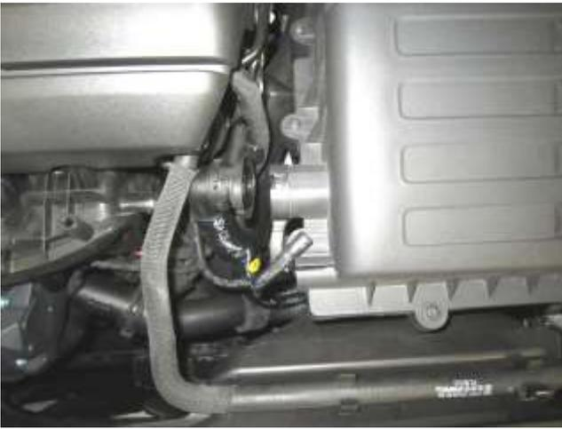
a. Remove the two hoses from the air box. The smaller hose will just slide off. The big hose will need to be squeezed to unlatch it. Note: Some models do not have this large hose.
