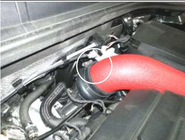
g. Install the AEM intake tube into the hump hose. Do not tighten the hose clamp yet.
