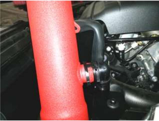
e. With warm water and soap, lubricate the O-ring on the factory connector. Then slide it onto the AEM intake tube making sure it latches into place. Note: Due to factory tolerances, rotating the fitting may be necessary.
