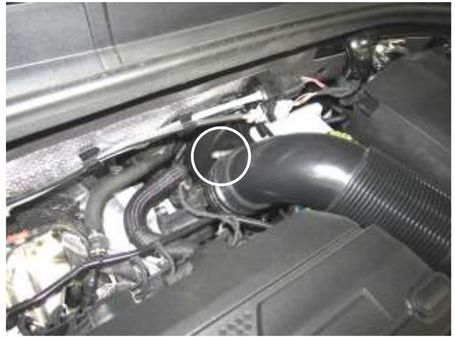
b. Loosen the hose clamp at the turbo compressor inlet and disconnect the intake tube.
