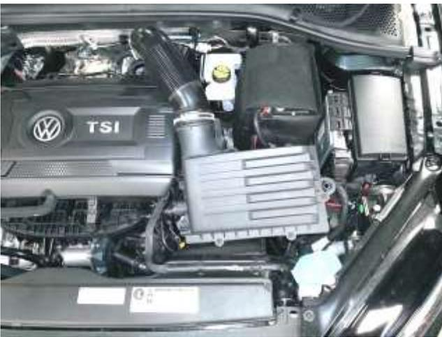
c. There are 3 rubber push on grommets securing the air box to the vehicle. Lift up on the air box and remove it from the vehicle.
