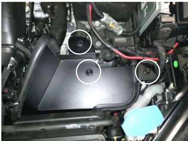
c. Using warm water and soap, lubricate the three dowel locators circled and align the grommets with them. Push down on the heat shield to secure.
