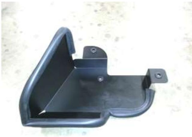
a. Install the 3 grommets into the heat shield, then install the edge trim onto the shield as shown.
