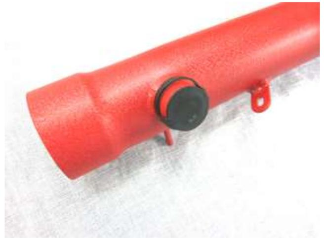
f. Certain models lack the large air injection hose. Use the included plug to block off this port as shown if your model is one that does not have this connector.
