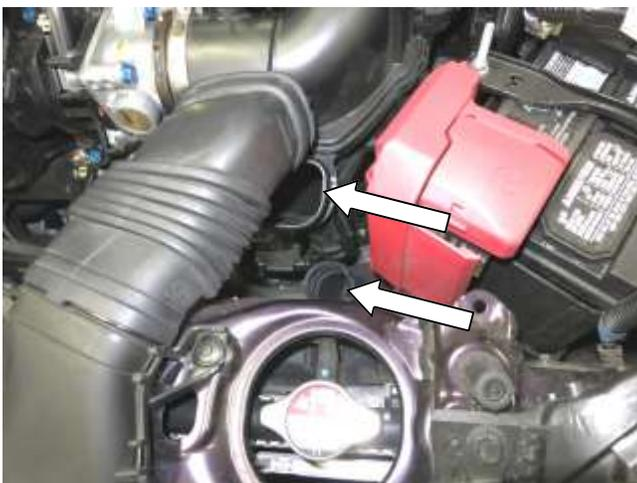
a. Disconnect the upper and lower air inlet ducts from the lower intake box.
