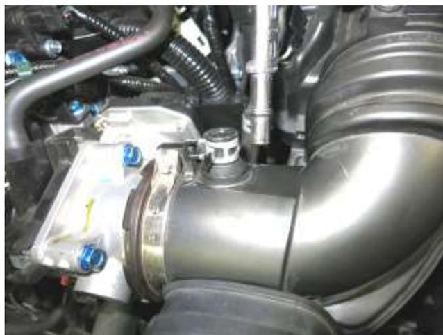
b. Depress the spring clamp on the intake tube to disconnect the hard breather line as shown.
