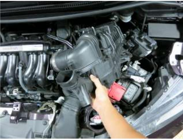
e. Carefully remove the stock intake assembly from the engine bay.
