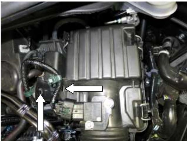
c. Disconnect the MAF harness from the connector. Unclip the two green tree-mount ties from upper airbox.
