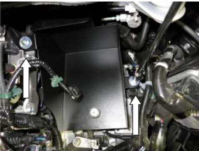
e. Install the heat shield and align locating tabs over the rubber mounts. Fasten tabs down with the provided nuts(AEM-444.460.04) and washers(08160).
