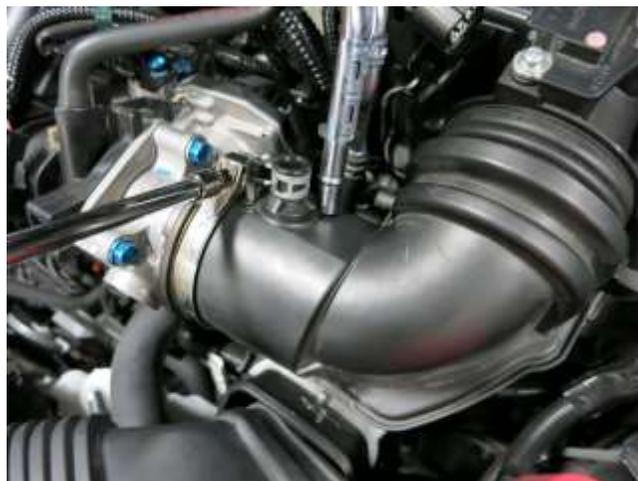
d. Loosen the hose clamp securing the intake tube to the throttle using a 8mm socket.
