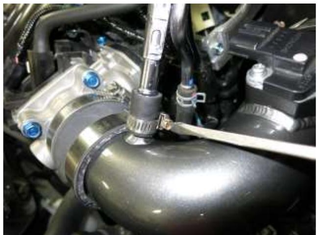
h. Connect the breather line to the intake tube using the hose(AEM-5-1002) and fasten hose clamp(AEM-4093-5). The hose may need to be trimmed for proper fitment.
