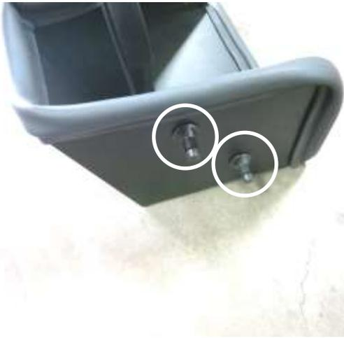
e. Install the plastic mounts with the provided hardware as shown.
