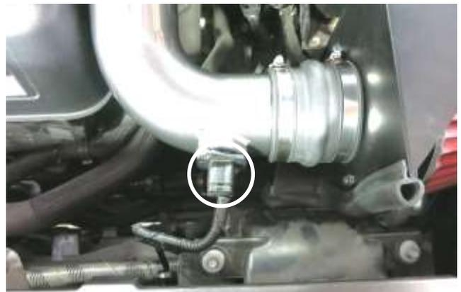
l. Re-attach the sensor connector to the sensor on the AEM intake tube and secure with the red locking tab.
