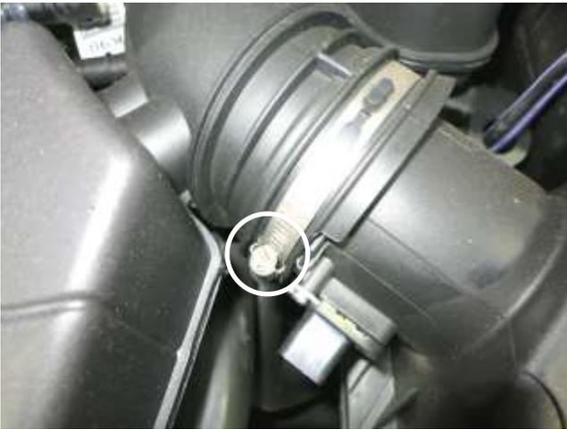
g. Loosen the hose clamp at the air box, and remove the stock intake tube from the vehicle.
