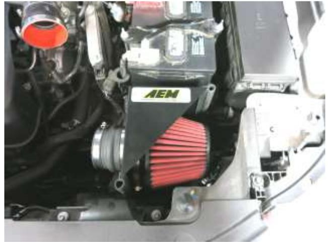
j. Install the complete heat shield assembly into the vehicle sliding the lower portion of the heat shield under the scoop and aligning the plastic mounts in the stock grommets.
