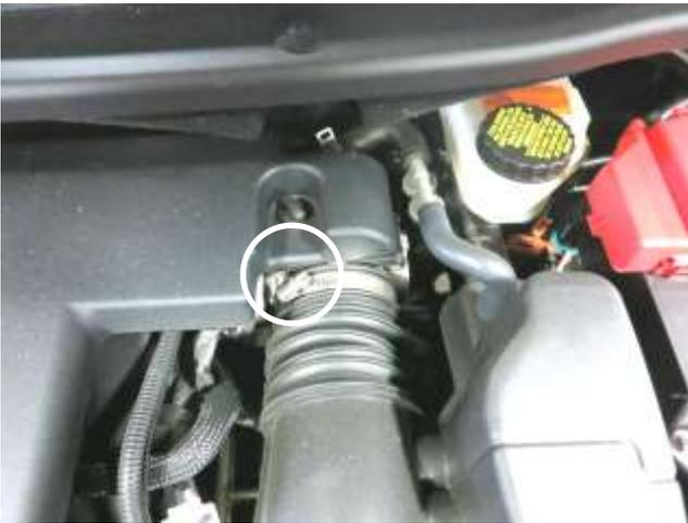
a. Loosen the hose clamp at the throttle body and disconnect the stock intake tube from the throttle body.
