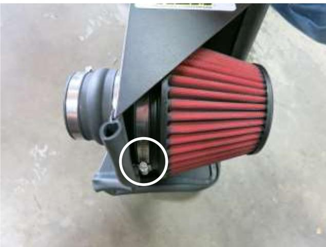
g. Insert the AEM air filter onto the filter adapter and secure with the hose clamp at this time.
