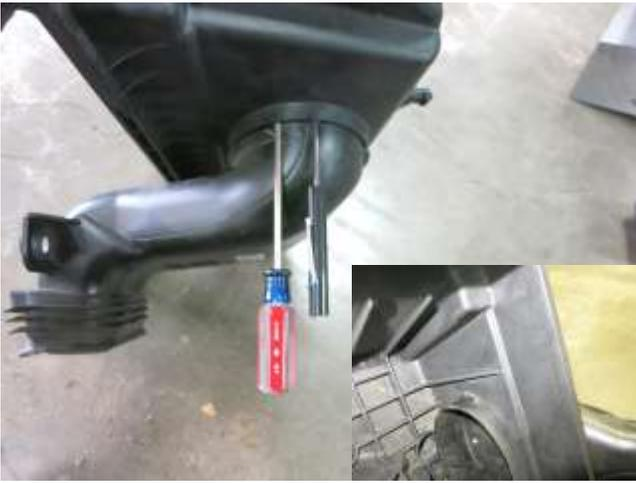
k. Insert two small flat head screwdrivers as shown into the scoop and lightly put pressure to release the clip securing the scoop to the lower air box. **NOTE:** The picture in the lower right hand corner shows the screwdrivers inserted on both side of the clip.
