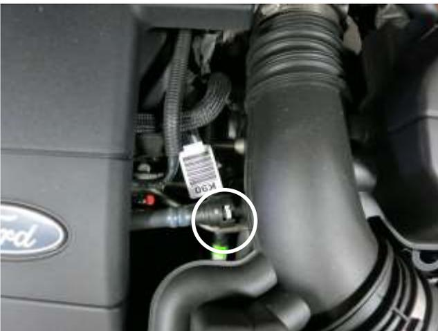
c. slide the gray tab on the vent line and disconnect it from the stock intake tube.
