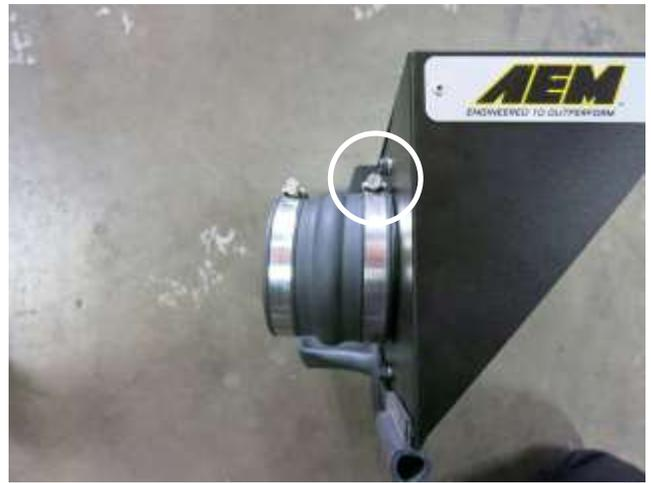
f. Install the provided coupler onto the air filter adapter. Tighten the hose clamp closest to the heat shield at this time.
