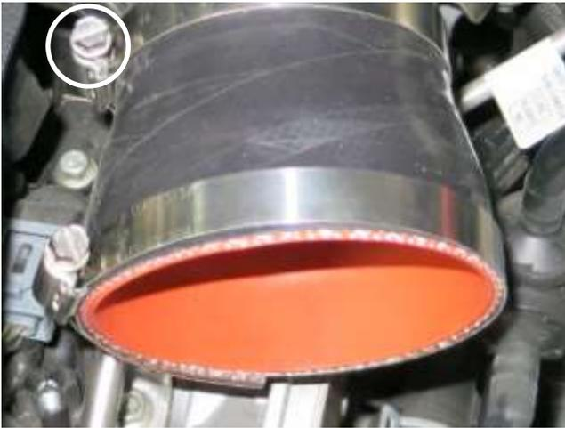
i. Install the provided coupler and hose clamps onto the throttle body. Tighten the hose clamp closest to the throttle body at this time.
