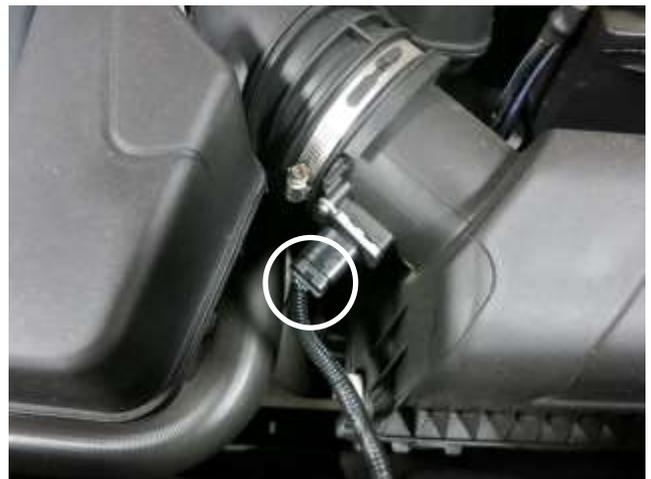
d. Slide the red locking tab back and depress the clip on the sensor connector to disconnect it from the sensor.
