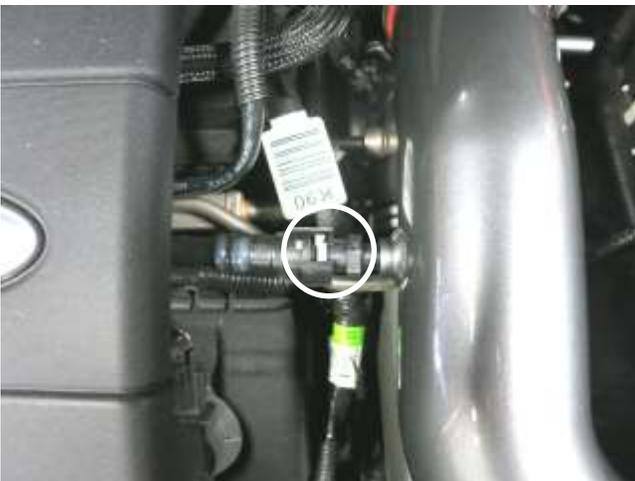
m. Reconnect the vent line onto the AEM intake tube.
