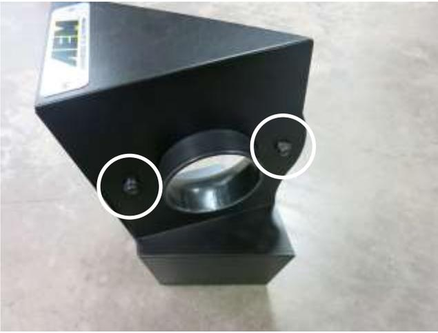
c. Install the filter adapter onto the heat shield with the provided hardware.
