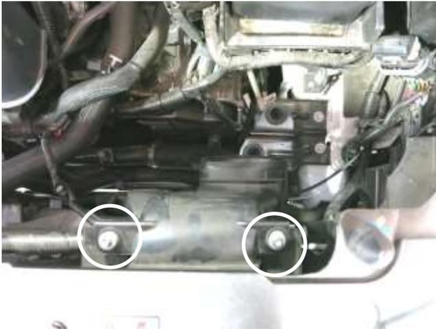
a. Install the scoop back into the vehicle and secure with the bolts that were removed in step 2f.
