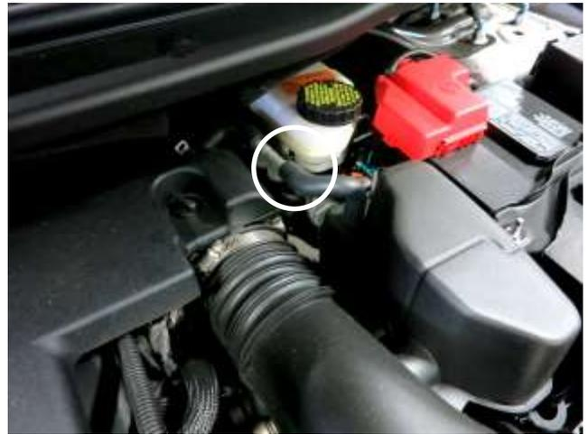
b. Remove the vent hose from the "T" circled.
