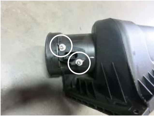
l. Remove the two T15 Torx. bolts that secure the sensor to the upper air box. Note: the sensor will be reused in step 3b. **Note: Some models do not have this sensor. See step 3b.**
