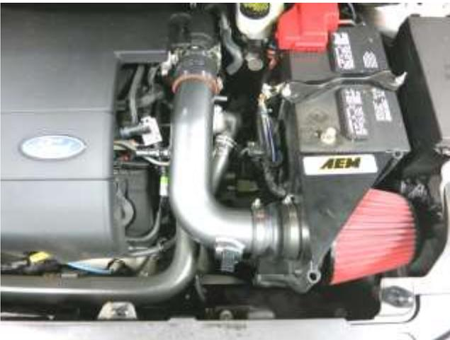
k. Slide the AEM intake tube into the coupler via the filter adapter side, then slide it into the coupler at the throttle body side.
