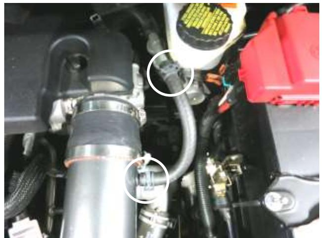
n. Connect the provided vent line onto the "T" and AEM tube and secure with the provided spring clamps.
