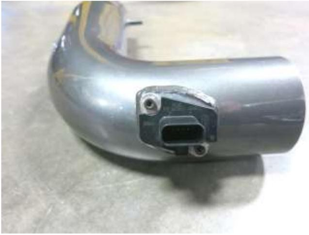
b. Install the sensor that was removed in step 2l and secure in the AEM intake tube with the provided hardware. **Note: Some models do not have this sensor. Use included block-off plate and gasket in place of sensor in these applications.**
