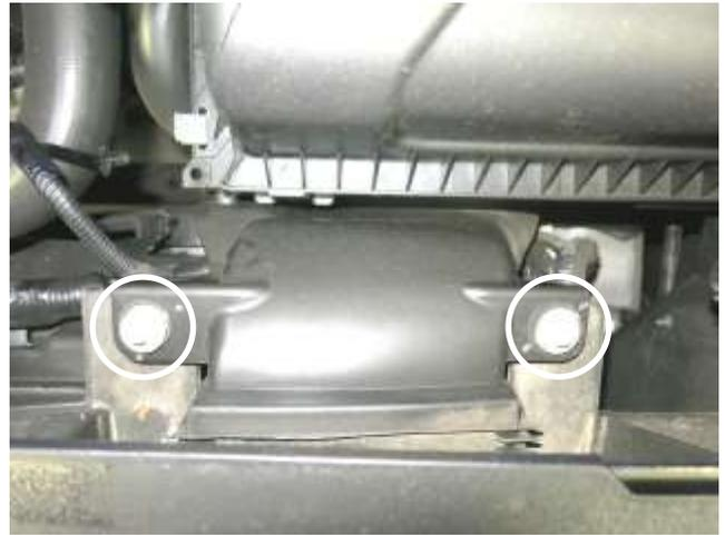
f. Remove the two bolts securing the stock air scoop to the vehicle. This and the bolts will be reused in step 3a.
