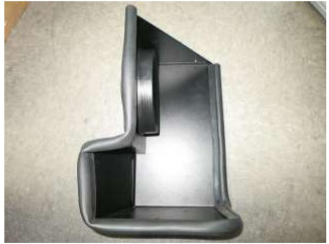
d. Install the provided edge trim onto the heat shield, cutting to fit as shown.
