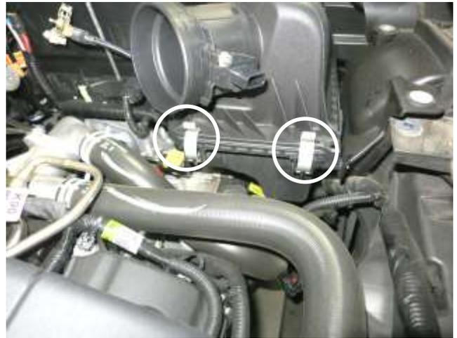
h. Unlatch the clips that secure the upper air box to the lower air box.
