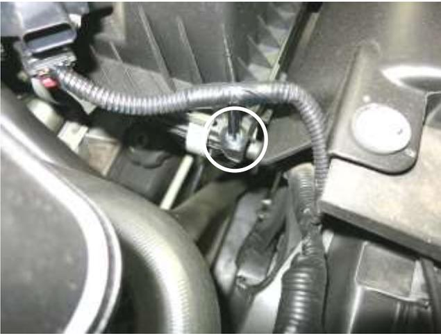
e. Pull the push in plastic connector from the upper air box.
