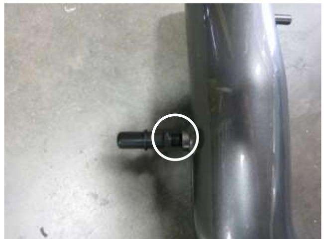
h. Install the provided fitting into the AEM intake tube by hand tightening and then torque a quarter turn with a wrench.
