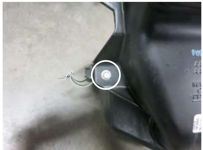
j. Remove the bolt that helps secure the stock air scoop to the lower air box.
