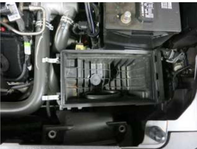
i. Remove the stock air filter and the lower air box from the vehicle. Note: Do not discard any of your stock equipment.
