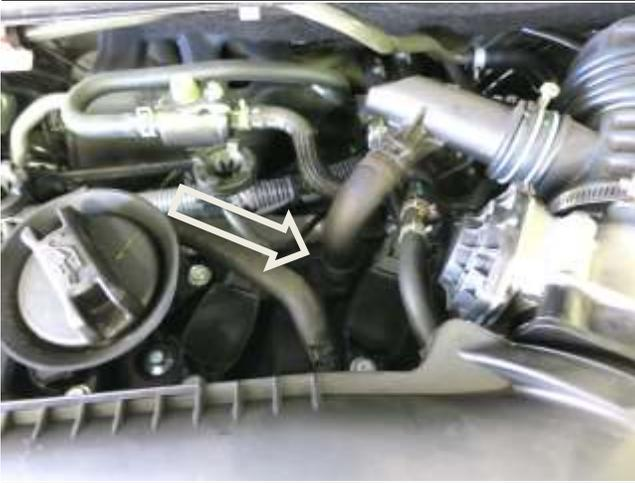
g. Using pliers, release the pressure on the spring clamp holding the vent hose to the engine and disconnect the vent hose from the engine. The two spring clamps will be reused in step 3m.
