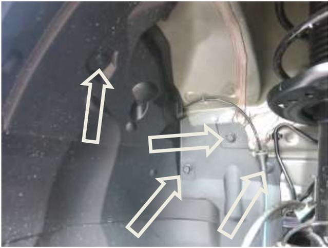
l. Remove the four pop outs shown in the inner fender well area.
