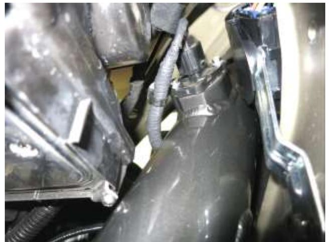
l. Route the MAF harness down to the MAF sensor and connect it as shown.
