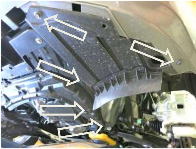
m. Remove the two bolts and three pop outs under the driver's side front corner of the bumper in the locations shown.
