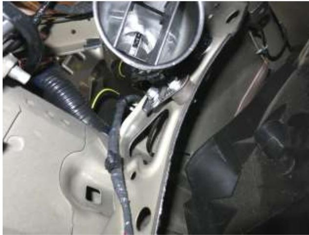
j. 2016 and newer models will require the use of the stainless steel offset bracket as shown. On all models secure the Intake tube bracket with the bolt and washer to the isolator. Note: the wiring harness that runs beneath the tube may need to be loosened and adjusted to fit properly.
