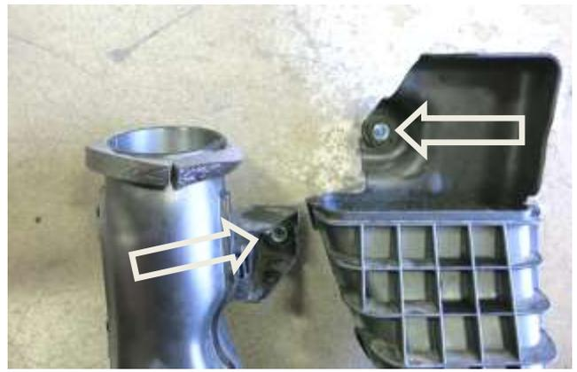
j. Loosen the two bolts holding the resonator in the front fender well area where the plastic duct was removed. These bolts are difficult to see but relatively easy to access from the engine bay.
