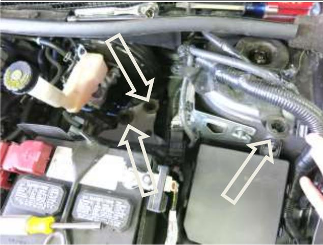
i. Remove the 3 rubber grommets that secured the air box and ducting and place them on the stock components for storage as they will not be reused.
