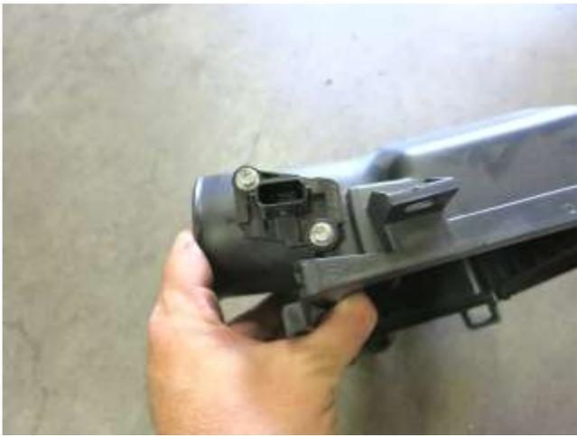
p. Remove the MAF sensor from the stock air box. Note: These screws will be reused in step 3a.
