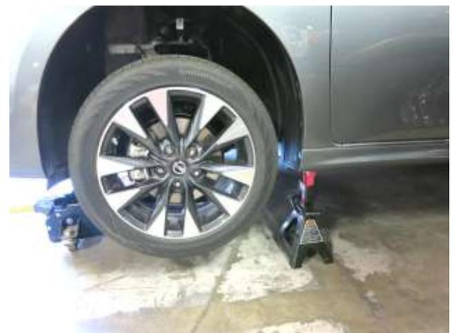
n. Torque all remaining hose clamps to 30 in-lbs, reinstall the engine cover, reassemble the fender liner, install wheel and torque lug nuts, and lower the vehicle.
