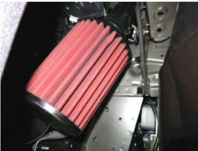
k. Install the AEM filter and torque the provided hose clamp to 30 in-lbs.
