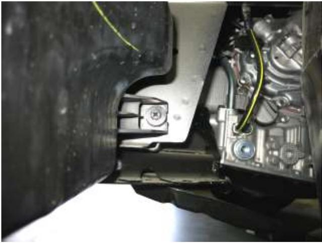
n. Lower the plastic fender liner to access the lower bolt securing the resonator and remove it.
