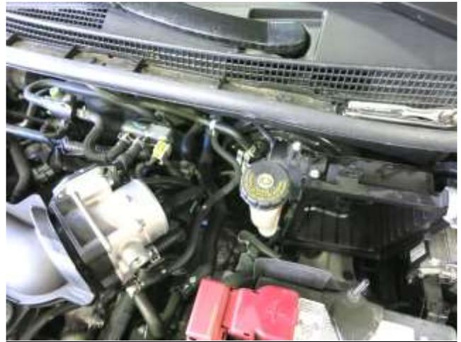
h. Remove the stock rubber air duct first, then remove the remaining section of air box by pulling it up and out of the engine bay.
