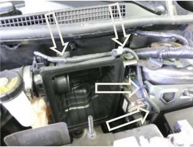
e. Unplug the Mass Air Flow (MAF) sensor harness and unclip the wire looms using a small flathead screwdriver to depress the tabs on the wire ties to release them from the air box.
