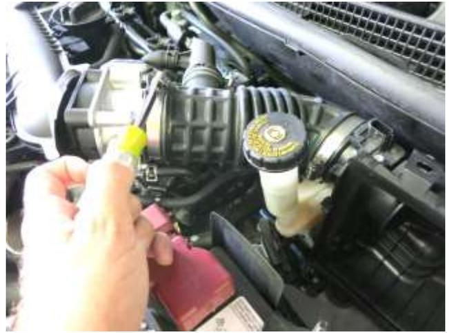
f. Loosen the hose clamps on the throttle body and air box.
