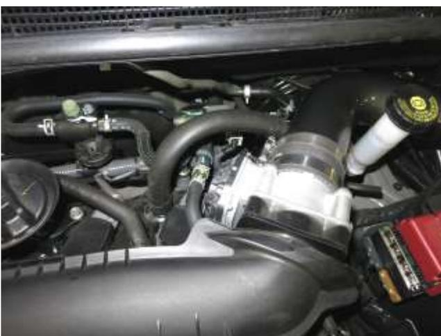
m. Using the spring clamps removed in step 2g, attach the provided vent hose from the engine to the AEM intake tube.
