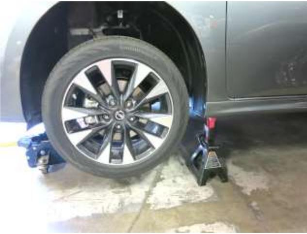
k. Break loose the lug nuts on the driver's side front wheel. Then, jack up the front of the vehicle and support it with jack stands. Then, completely loosen the lug nuts and remove the wheel.
