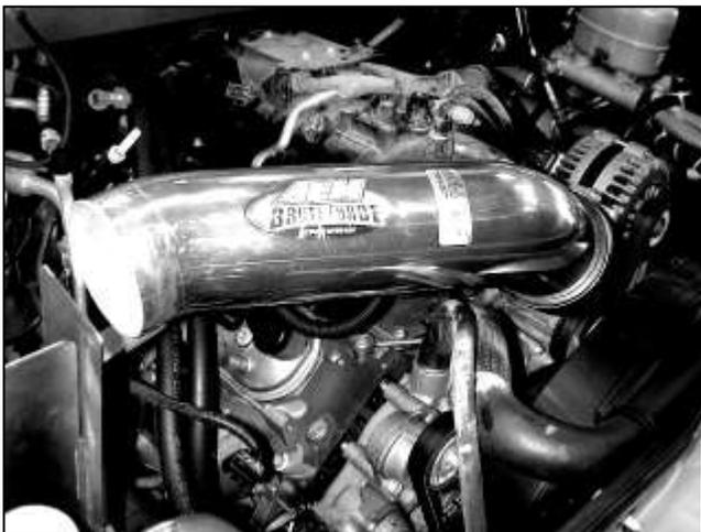
h. Insert the inlet pipe into the 90-degree coupler. Secure with provided hose clamps.
