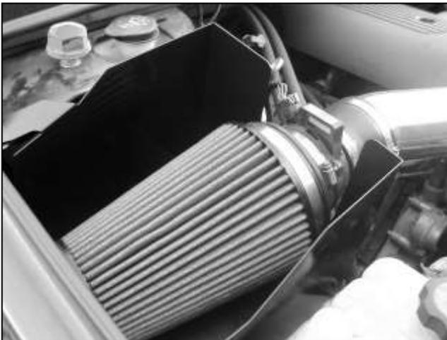
l. Attach the air filter assembly to the intake pipe and secure. Plug in MAF sensor.
