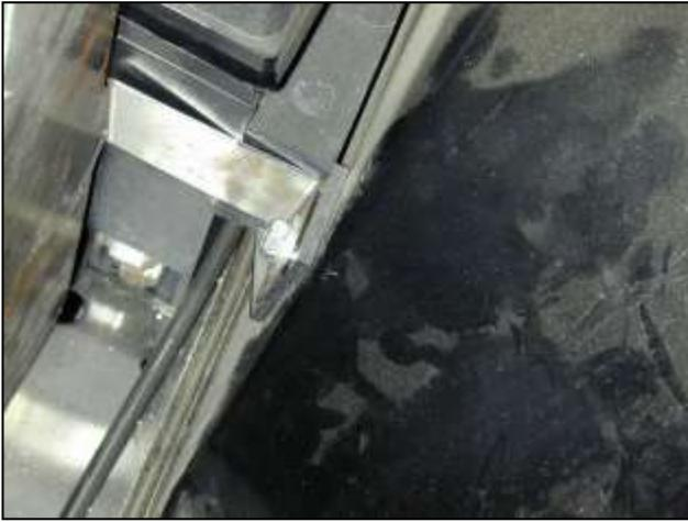
h. Reinstall the bolt that was removed in step 2j through the hole in the U shaped tab on the heat shield. Once secured, fully tighten the 2 ¼" bolts from step 3g. This will load the heat shield in order to fully secure it.
