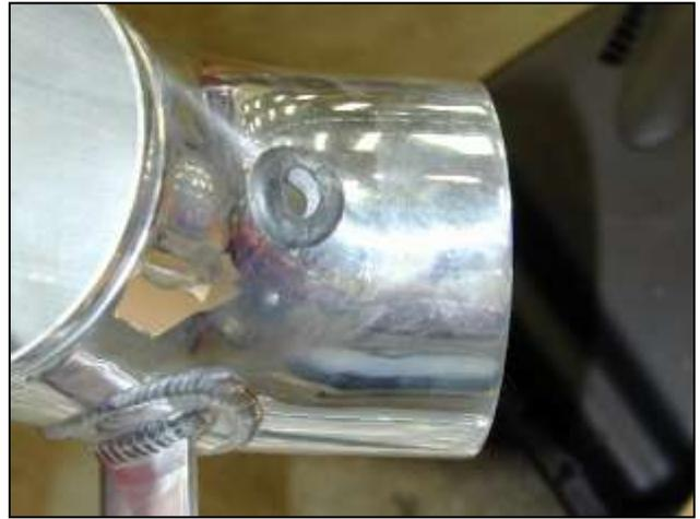
m. Insert the rubber grommet into the hole on the lower intake pipe as shown.
