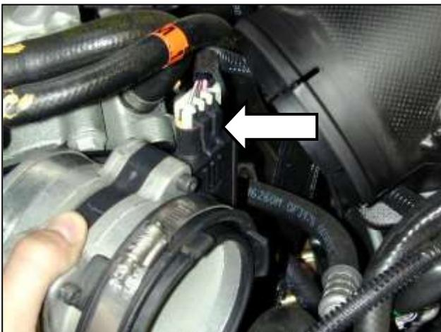
c. Loosen the hose clamp securing the MAF adapter to the air filter housing. Unplug the wiring harness from the MAF sensor and remove sensor.
