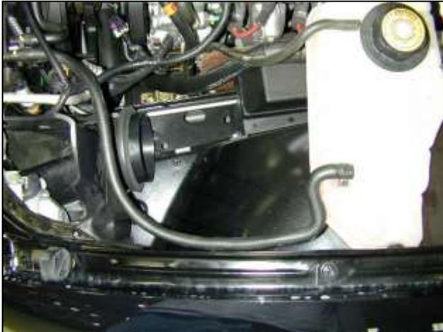
g. With the coolant reservoir out of the way, remove the lower half of the air filter housing by gently lifting it up. This is held in place with grommets similar to the coolant reservoir.
