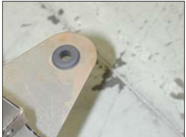
c. Install the rubber grommet into the hole in the heat shield as shown.
