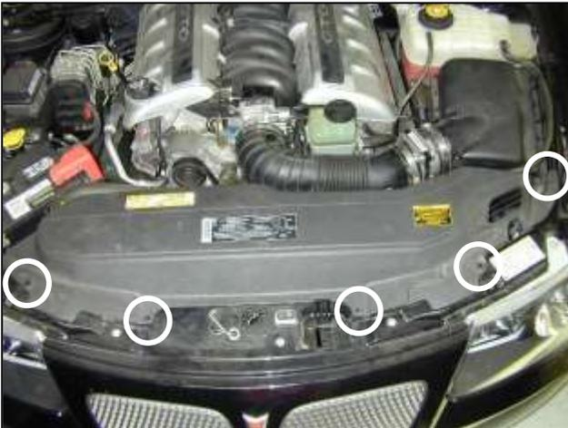
a. Remove the radiator shroud from the front of the car by removing the 5 plastic connectors.
