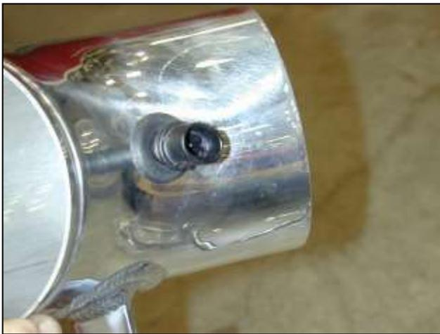
n. Insert the IAT sensor into the grommet. This may be eased with the use of some lubrication on the rubber grommet. Be careful not to damage the IAT sensor.
