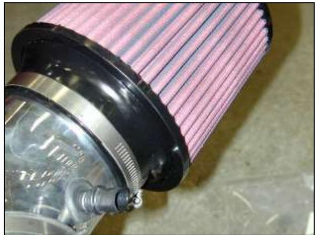
o. Install the AEM<sup>®</sup> air filter on to the end of the inlet tube. Push the air filter over the inlet pipe until the stop in the filter is reached. Then install one hose clamp to secure the filter onto the inlet pipe.
