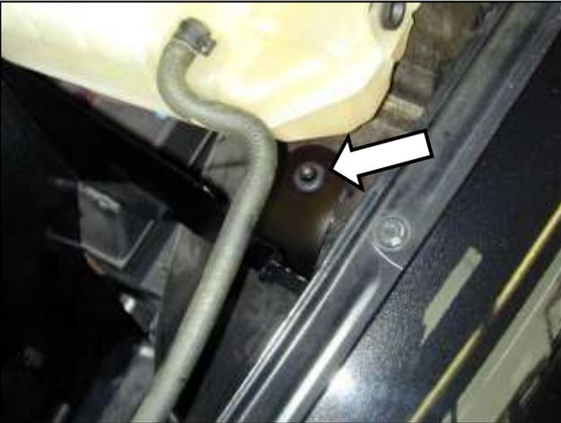
f. Carefully slide heat shield into engine bay. Push rubber grommet installed in previous step over the stud on the strut tower.
