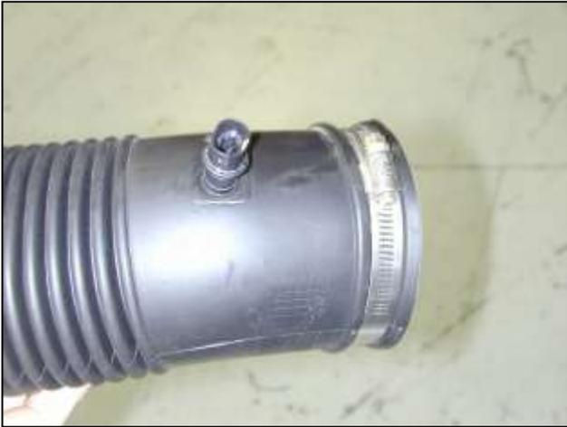
i. Unplug the IAT sensor from the stock intake tube. The best way to do this is to pull straight back while twisting gently.
