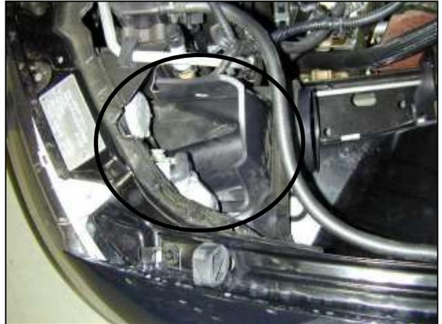
h. Remove the air shield by bending it slightly and pulling it towards the shock tower.
