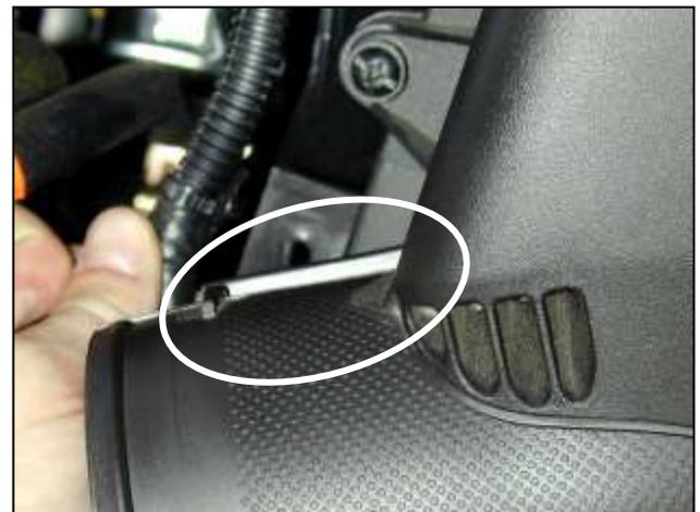
d. Detach the wiring harness air filter housing as shown.
