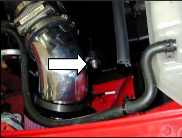
p. Insert the lower intake pipe and tubing spacer into the stock rubber coupler on the MAF sensor. Align the mount with the bracket on the pipe. Install the washer and Nylok nut onto the rubber mount.
