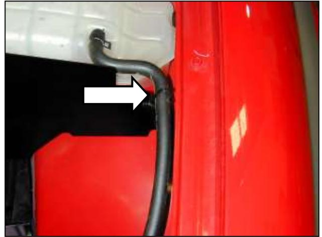
q. Install the supplied heat shield zip-tie into the on the tab for the coolant reservoir hose.
