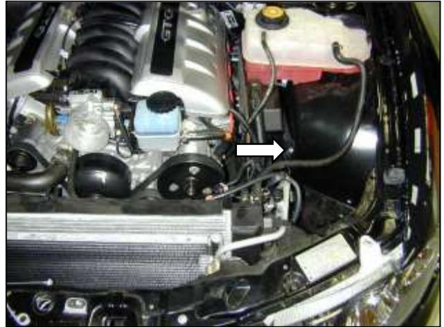
j. Remove the bolt shown on the inner fender. This bolt will be reinstalled later.
