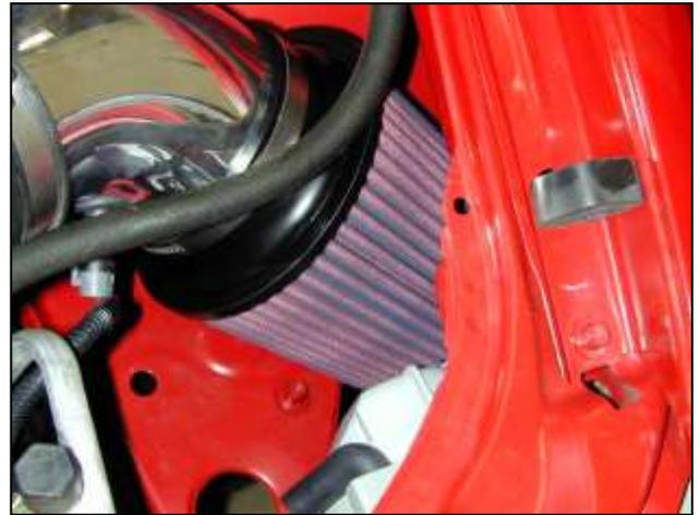
s. Ensure the air filter is not touching any part of the vehicle. Position the intake system for best fitment. Be sure that the inlet pipe or any other component is not in contact with any part of the vehicle. Tighten the hose clamps at the throttle body and silicone coupling. Tighten the nut on the mounting bracket. Re-adjust the inlet pipe if necessary.
