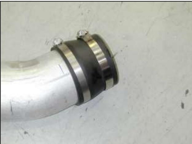
j. Install the reducer coupler onto the intake pipe using the supplied #64 hose clamp. Install the #56 hose clamp onto the 3.5" side of the coupler.
