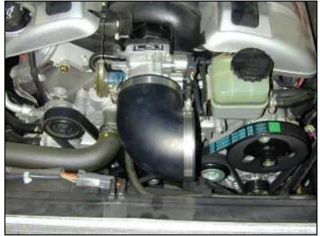
i. Install the long end of the rubber elbow over the throttle body using the supplied #64 hose clamps.
