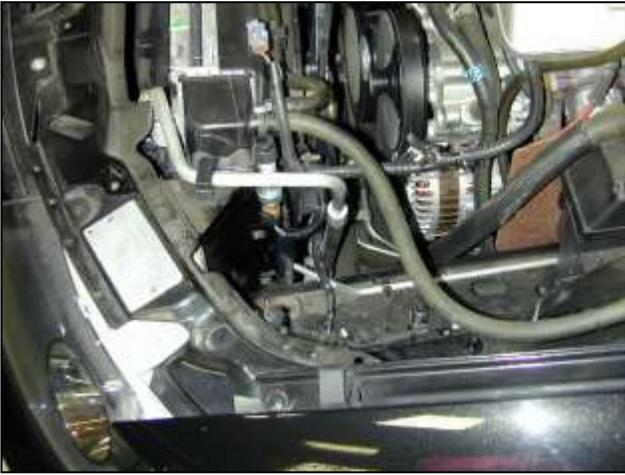
d. Route the wires for the IAT, MAF, and ACPT so they are in front of the AC line but behind the radiator support as shown.
