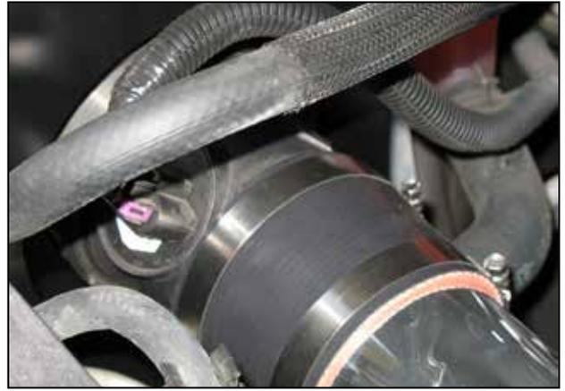
h. Then attach the assembly made in step 3f to the end of the intake pipe. Then reconnect the MAF sensor wire.
