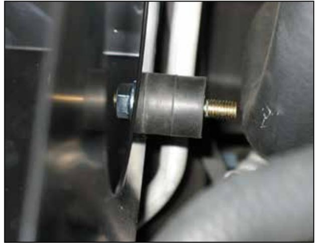
d. Install rubber mount on the heat shield using the supplied washer and nut.
