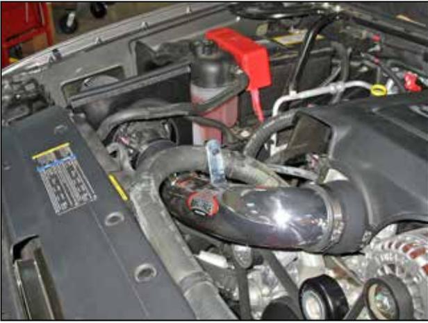
m. Install filter assembly into the stock MAF rubber coupler. Also put the rubber edge gasket along the top edge of the heat shield.
