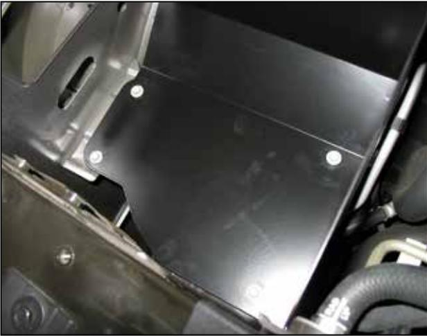
c. Install the heat shield using the four stock bolts used to secure the air filter box mounting plate.
