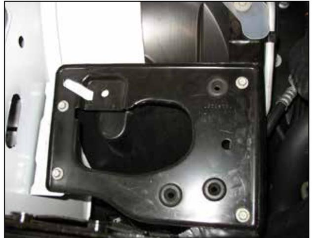
h. Remove the four bolts securing the stock airbox mounting plate.
