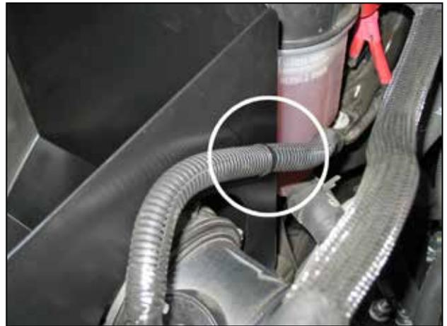
j. Use the supplied tree mount to secure the MAF sensor wire to heat shield.
