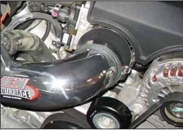
g. Insert intake pipe into reducing coupler located at the throttle body. Route the intake pipe under the upper radiator hose. Secure the bracket to the rubber mount on the heat shield.
