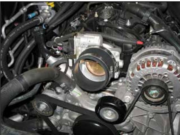
e. Install the reducing coupler on the throttle body, and loosely put the supplied hose clamps on the two ends of the coupler.
