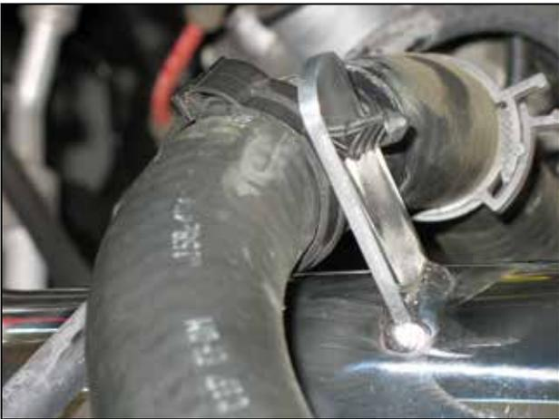
i. Use the stock plastic radiator clamp to secure the radiator hose away from the intake pipe. By inserting it into the bracket located on the pipe.
