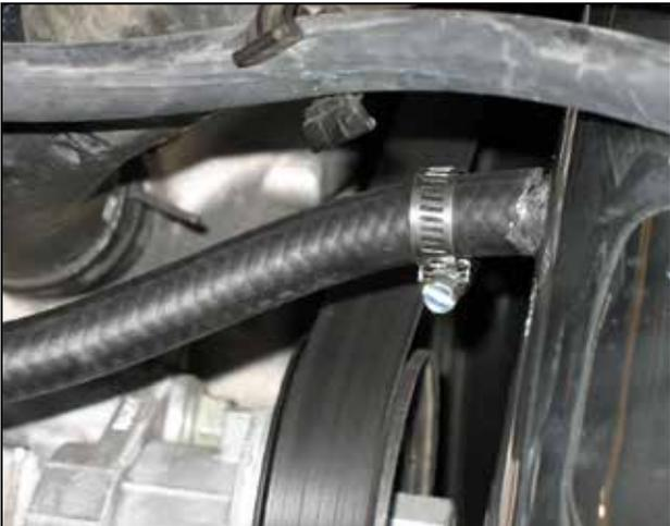
o. Finally, secure the breather hose to the nipple on the intake pipe.
