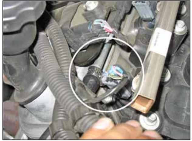
n. Secure the supplied breather hose with the supplied hose clamp.
