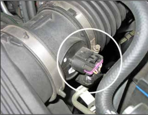
e. Disconnect the mass air flow sensor wire, and loosen the hose clamp securing the MAF housing to the stock inlet tube.
