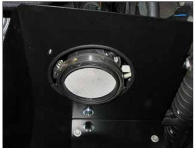
l. Install rubber edge trim on the heat shield where the intake pipe will pass through.
