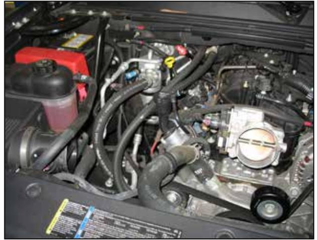
f. Pull the stock inlet tube out of the vehicle.
