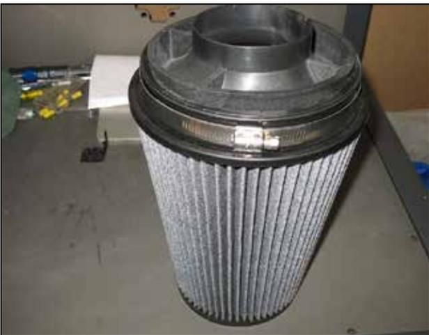
k. Create an assembly of the supplied air horn and the air filter.
