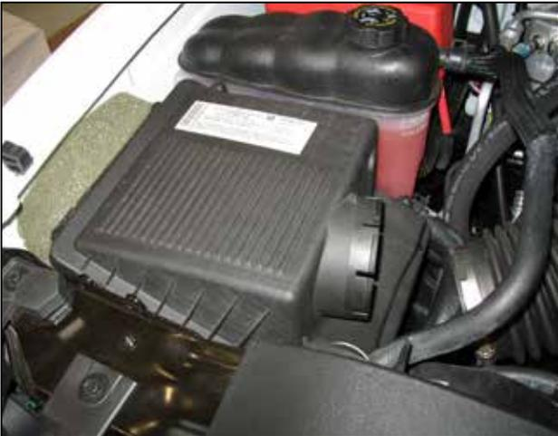
g. Pull the stock air filter housing straight up out of the vehicle.
