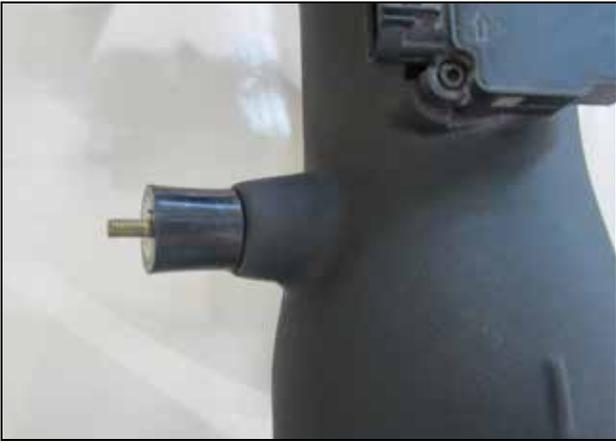
n. Attach the supplied rubber mount to the set screw supplied and install it 3/8" away from the rubber and then thread it into the AEM® intake tube (9-0402).
