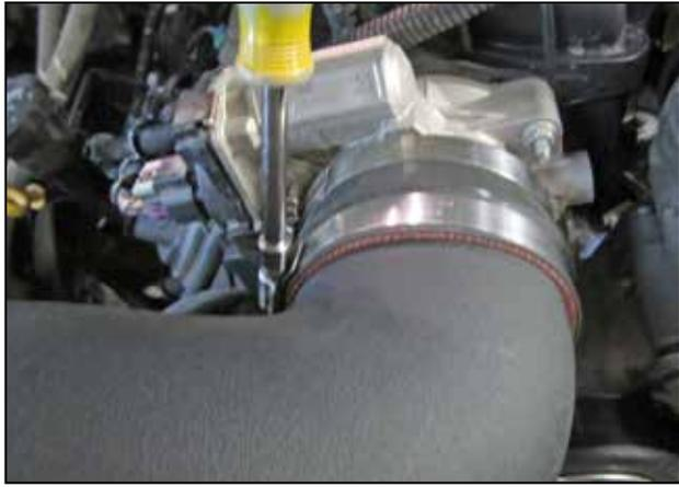
u. Tighten the hose clamp (9464) at the throttle body.
