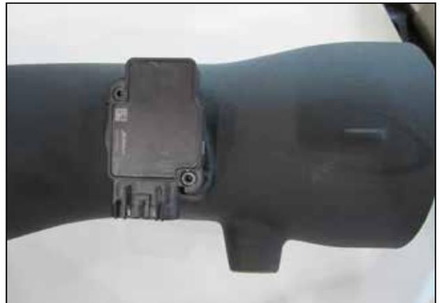
m. Install the MAF sensor in the AEM® intake tube (9-0402) with the two supplied M4 screws (1-2105).
