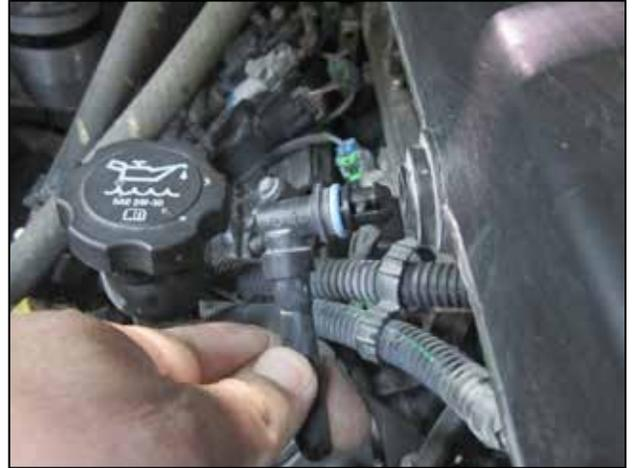
b. Disconnect the PCV line from the resonator.
