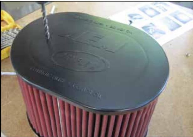
j. Drill a 1/4" hole in the filter cap of the air filter (21-2277DK), below the corner of the "A" for the filter minder grommet.
