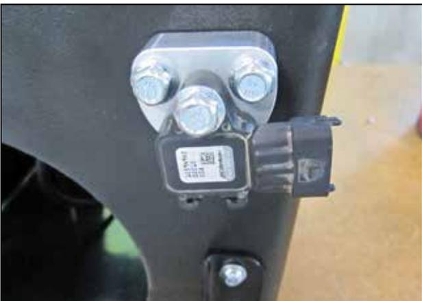
f. Install the filter minder sensor onto the adapter using 1 M6 bolt (1-2038).
