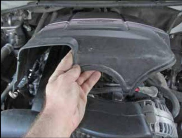
a. Remove the engine cover by lifting up on the front and pulling it forward.
