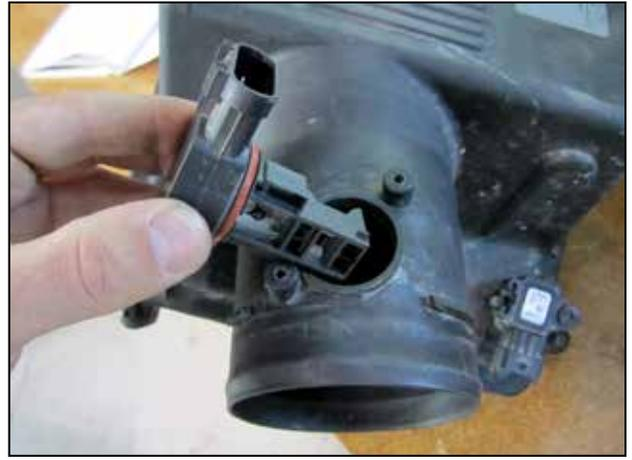
r. Remove the MAF sensor from the air box.
