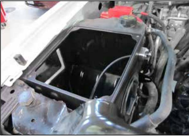
h. Install the AEM® air box (9-0390-1) into the vehicle.
