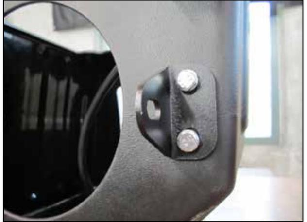
c. Install the pipe bracket (32-3079) onto the AEM® air box (9-0390-1) using the supplied M6 bolts (1-2065) and washers (1-3016).
