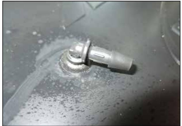
k. Install the grommet (784631) and 90 deg. fitting (8-152) into the air filter's filter cap as shown.
