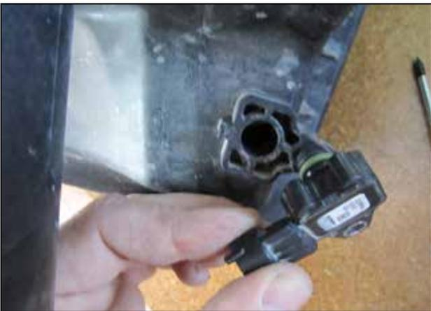
s. Remove the filter minder sensor from the air box.
