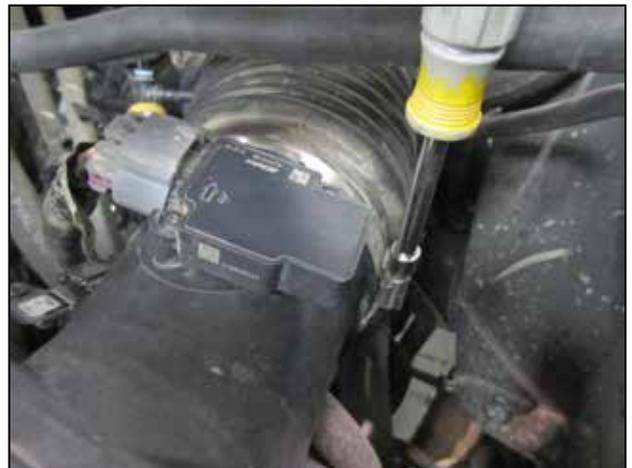
d. Loosen the hose clamp at the air box neck.
