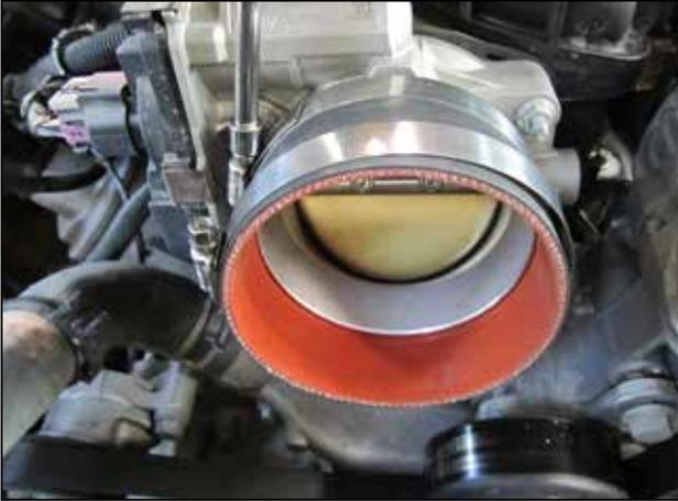
b. Install the provided coupler (5-402) and 2 #64 clamps (9464) onto the throttle body.
