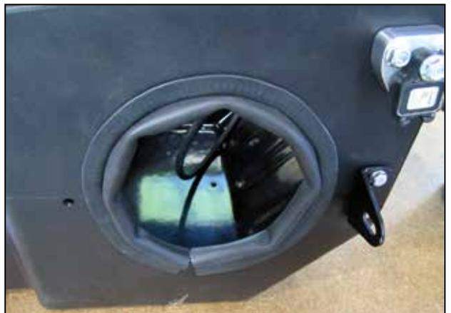
g. Install the rubber edge trim (8-4018) onto the AEM® air box (9-0390-1) as shown.
