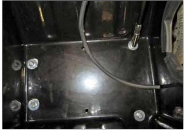
i. Secure the AEM® air box (9-0390-1) using the 4 supplied M6 bolts (1-2038) and washers (08160).
