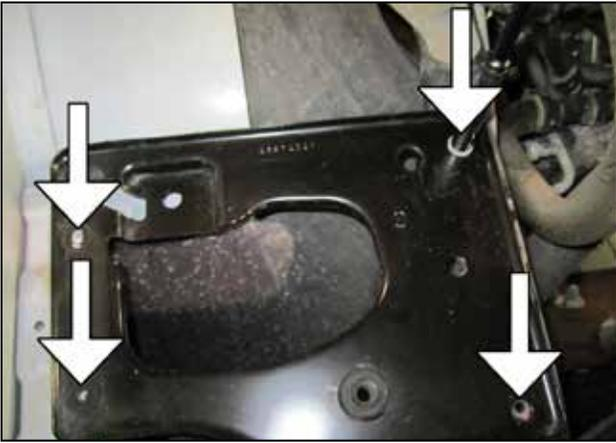
k. Remove the air box tray by removing the 4 M6 bolts.
