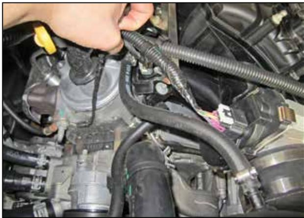
w. Push the plastic connector (8-125) into the grommet installed in the AEM® intake tube. Connect the other end of the hose (5-1012) to the PCV line on the engine, tighten both hose clamps (4093-5).
