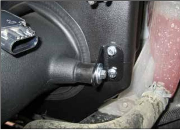
t. Install the rubber mount (1228599-1), washer (08160) and M6 nut (444.460.04) onto the bracket. Align for best fit and tighten the bracket bolts and rubber mount.
