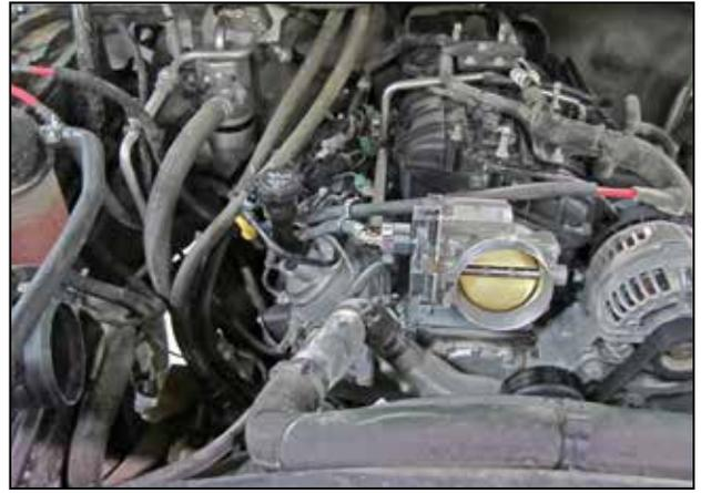
f. Remove the intake tube and resonator.
