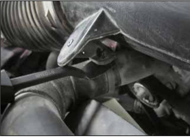
e. Unclip the radiator hose from the intake tube.
