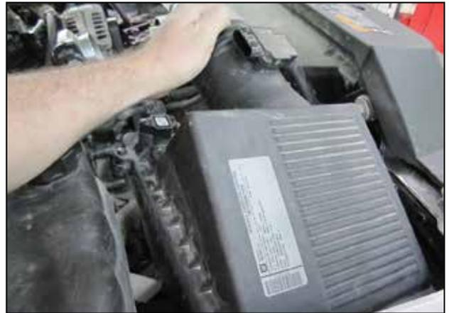
j. Remove the air box from the vehicle by firmly lifting up to disengage its clips.
