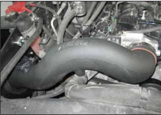
p. Install the AEM® intake tube (9-0402) as shown.
