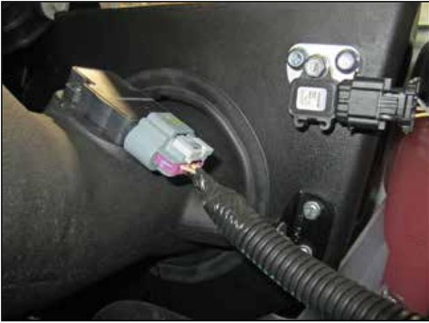
z. Reconnect the MAF air flow sensor and filter minder sensor.
