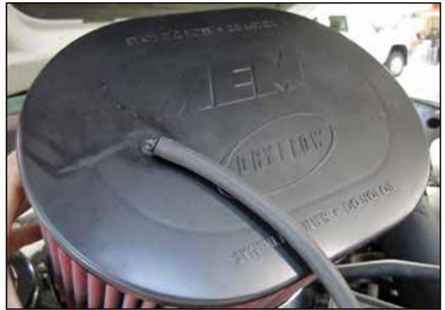
q. Attach the filter minder hose (5-3020) to the 90° fitting (8-152).
