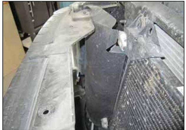
n. Locate the air deflector behind the grill on the passenger side of the radiator.
