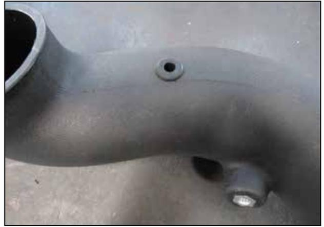
o. Install the supplied grommet (784642) into the AEM® intake tube (9-0402).
