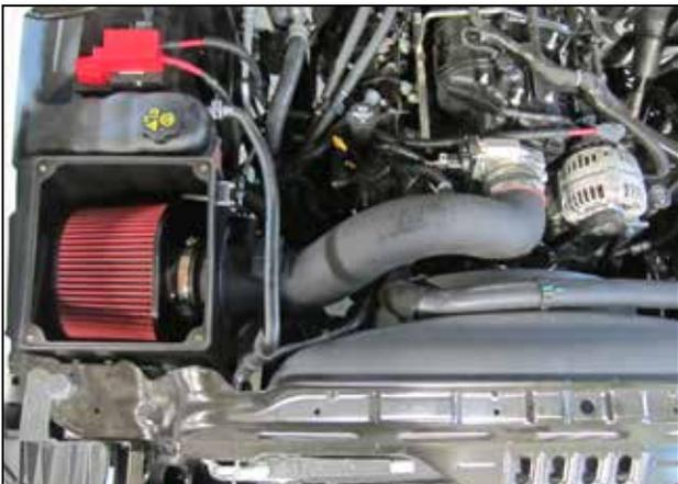
x. Align for best fit and tighten all hose clamps and hardware.
