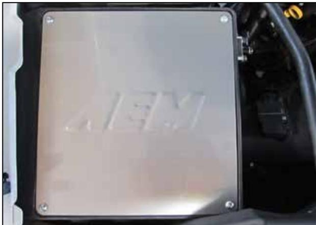
y. Install the AEM® air box lid (20-8514) using the 4 M6 bolts (1-112) and nylon washers (1-3001).
