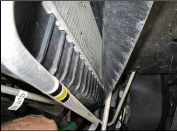
q. Remove the final clip at the bottom, then remove the air deflector.
