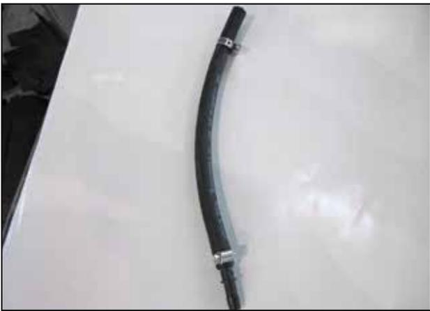
v. Assemble the 3/8" hose (5-1012), plastic connector (8-125), and two hose clamps (4093-5) as shown.
