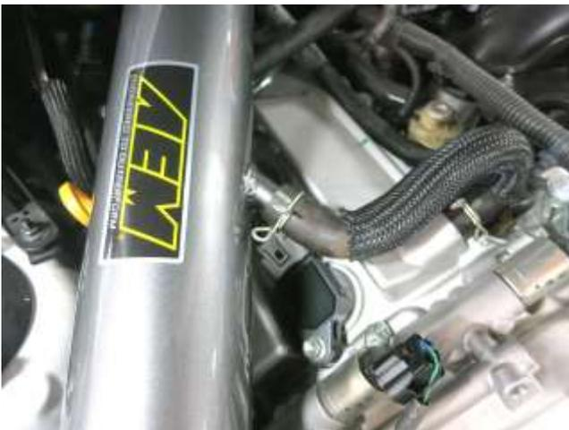
i. Connect the factory vent hose to the AEM intake tube and secure with the factory spring clamp.
