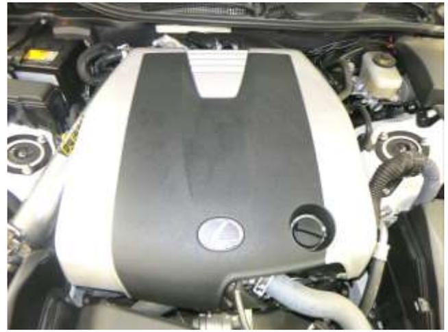
l. Replace the plastic engine cover by lining up the rubber grommets with the posts on the engine and pushing down to secure.
