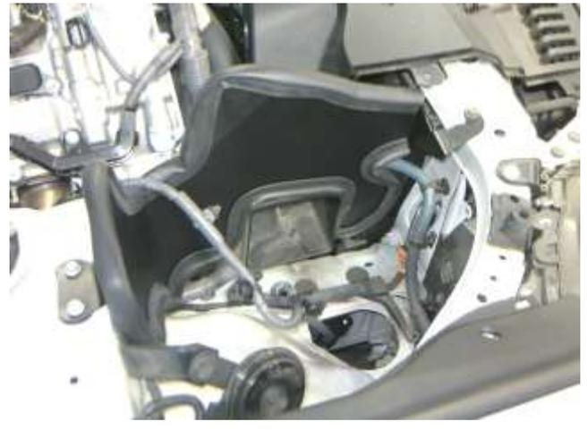
f. Install the heat shield as shown using the two provided bolts and the core support bolt removed earlier. The scoop position may need adjusting during installation.
