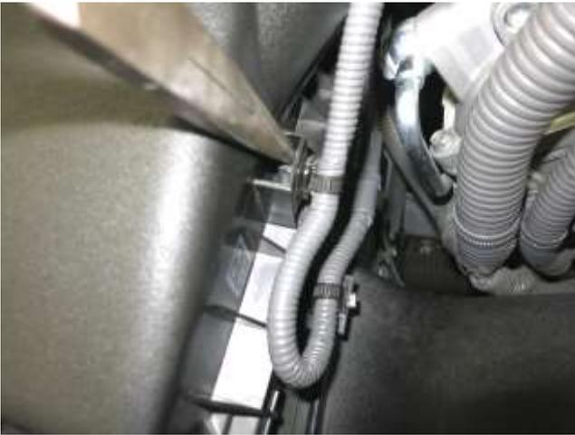
e. Use needle nose pliers to release the first wire tie clip on the factory air box.
