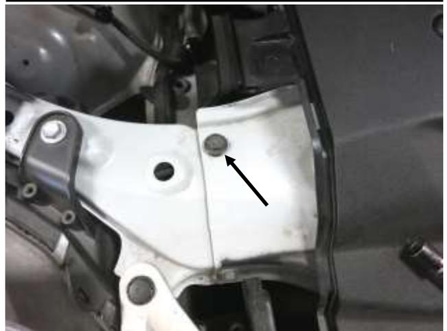
J. Remove the core support bolt. This bolt will be reused in step 3f.
