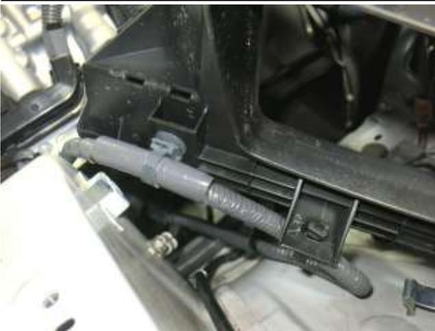
i. Pull the air box base upwards and to your left to release it from the fresh air scoop and rubber grommet. Rotate the box upside down so the last two wire clips are accessible. Disconnect them and remove the box from the engine bay.
