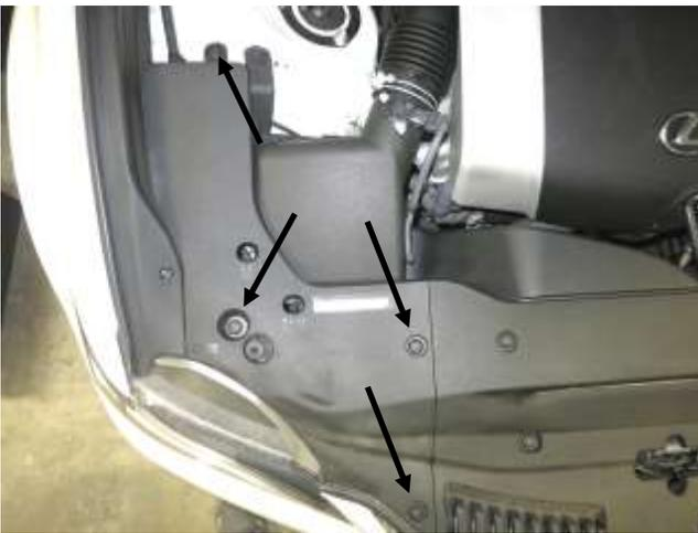
a. Remove the plastic shroud over the air box by depressing the 4 plastic rivets and removing them.
