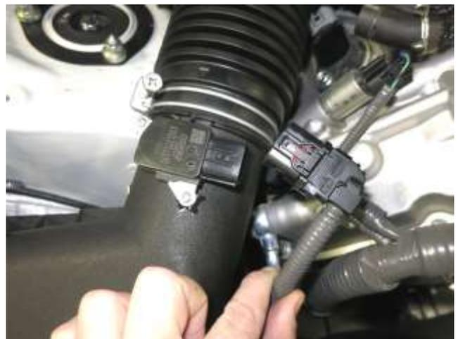
d. Disconnect the Mass Air Flow (MAF) sensor by depressing the clip.
