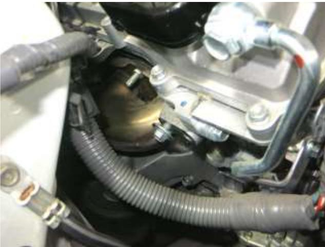
c. Thread the included large bolt and washer onto the location shown on the side of the motor. Leave roughly 1/4" of space for the intake tube bracket.
