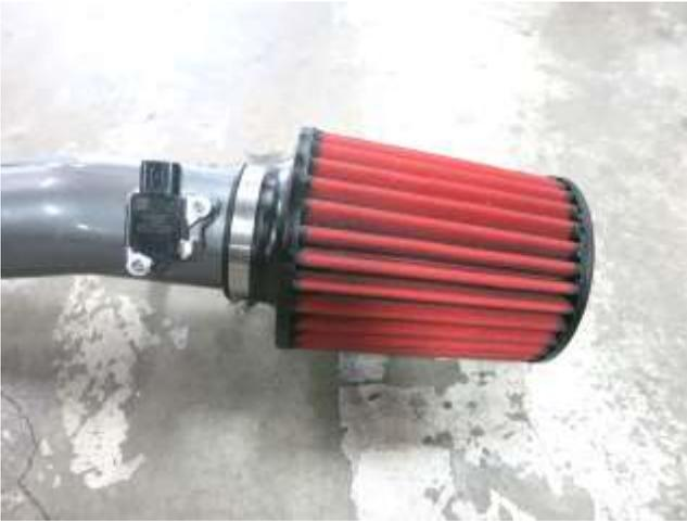
a. Install the MAF sensor using the supplied bolts, then install the AEM DryFlow filter using the supplied hose clamp.
