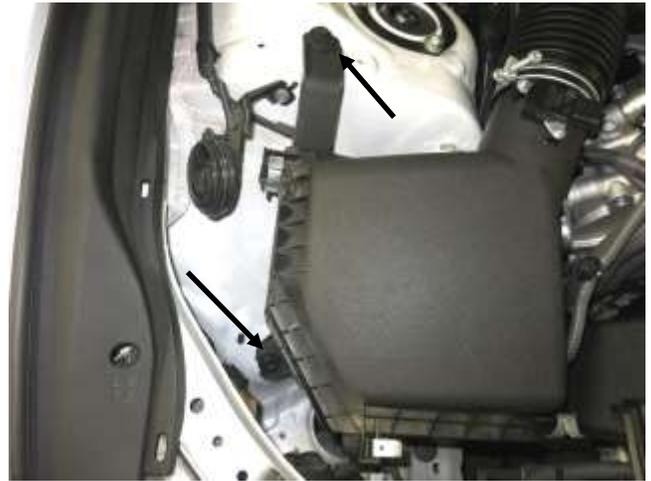
f. Remove the two bolts securing the factory air box.
