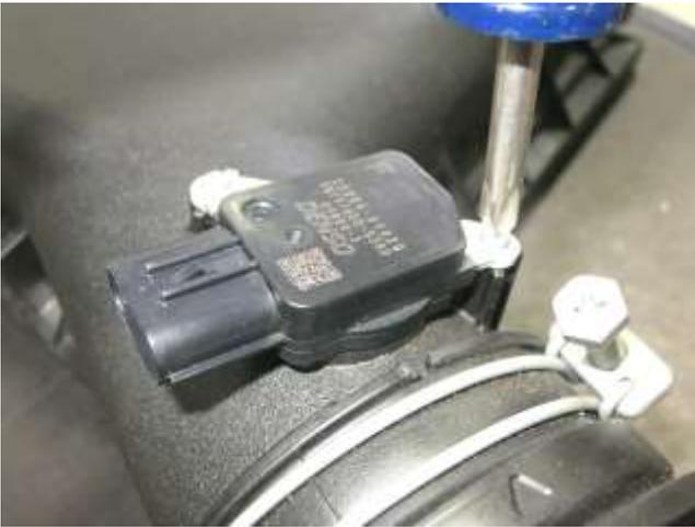
k. Remove the MAF sensor from the upper part of the factory air box. The sensor will be reused in step 3a.
