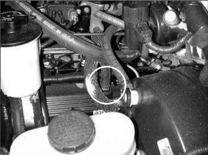
u. Attach the other end of the crankcase breather tube to the nipple of the crankcase and secure.
