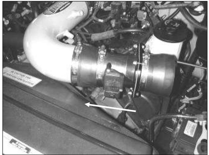
l. Attach MAF assembly to the upper inlet pipe, the flow arrow on the MAF sensor should be pointing to the upper inlet pipe.
