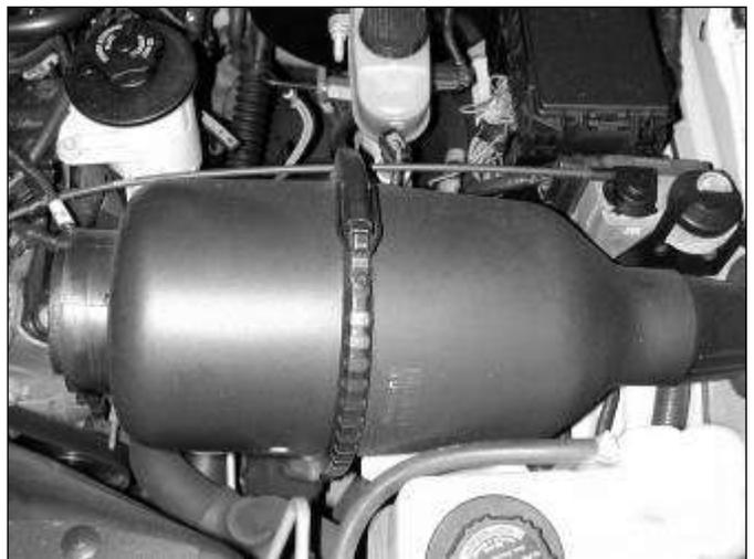
h. Unclasp the latch for the air filter and MAF sensor.
