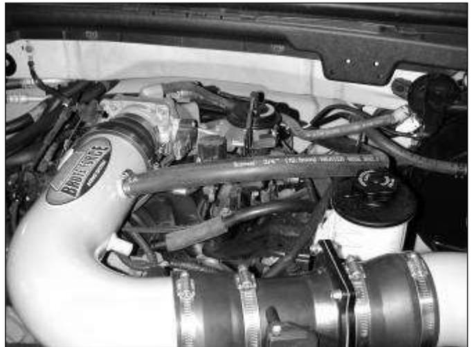
q. Attach breather hose for the IAC and secure it to the check valve.
