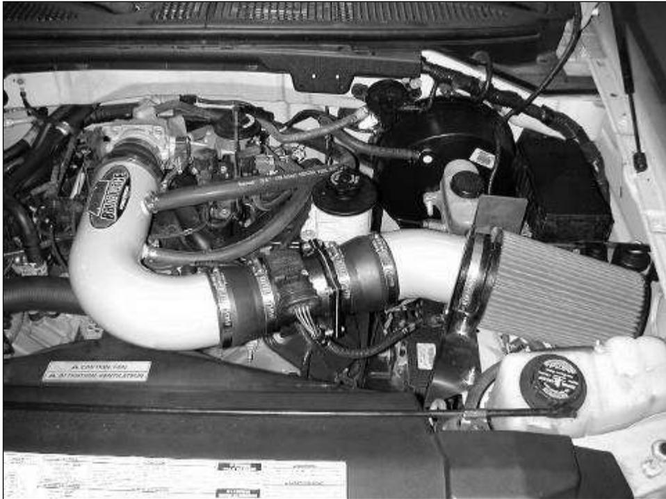
w. Plug the wire harness connector back into the MAF sensor.
