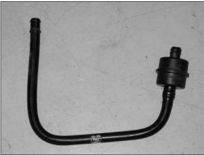
o. Remove this portion of the IAC breather tube from the vehicle. Remove the tube from the check valve, the check valve will be used with the AEM<sup>®</sup> intake system.
