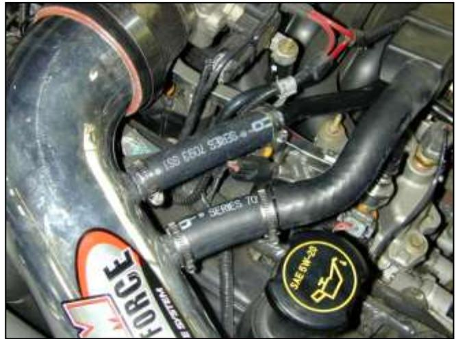
e. Attach provided 3/4" breather hose for the PCV and secure with provided hose clamps.
