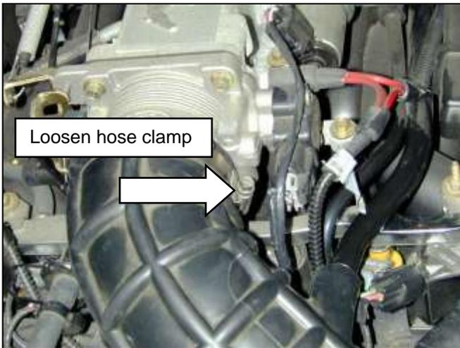
a. Loosen the hose clamp on the inlet air tube on the throttle body.
