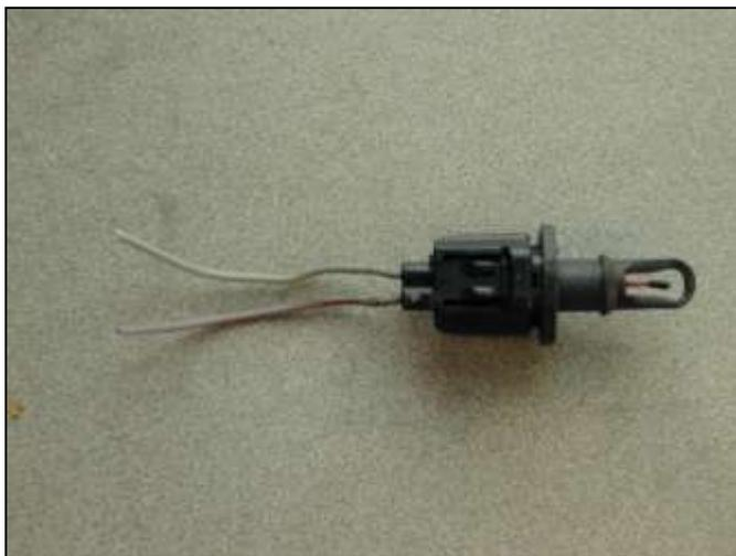
l. Strip off the wire loom from the sensor.
