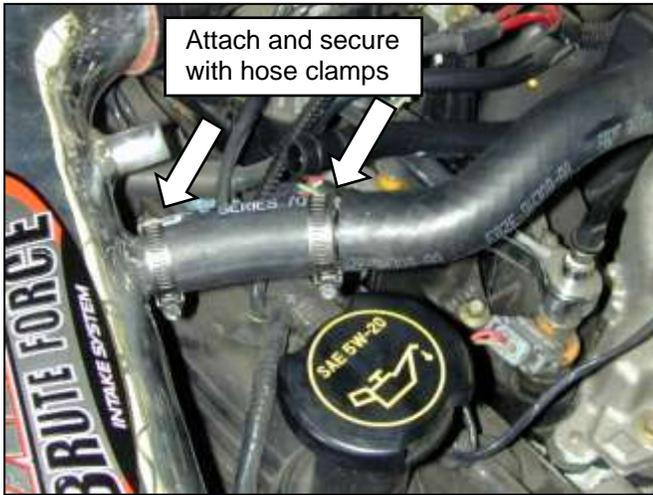
d. Attach the provided 5/8" hose for the IAC and secure with provided hose clamps.
