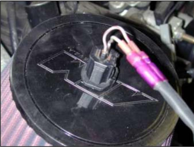
t. Insert IAT into the air filter end and attach to air horn.
