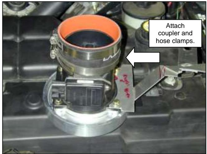
g. Attach coupler and hose clamps. Do not completely tighten.
