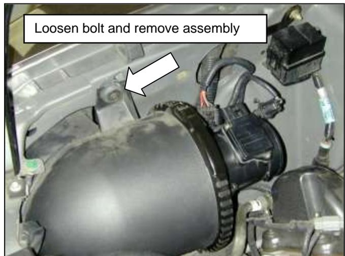
d. Loosen bolt and remove air filter assembly with MAF sensor.
