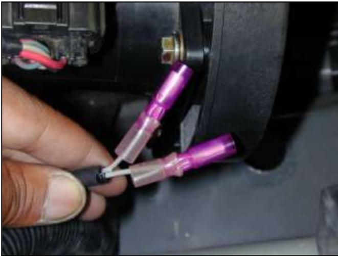
p. Strip off a ¼" section from each end and attach the 2 female end butt-connectors. Crimp and apply heat to each.
