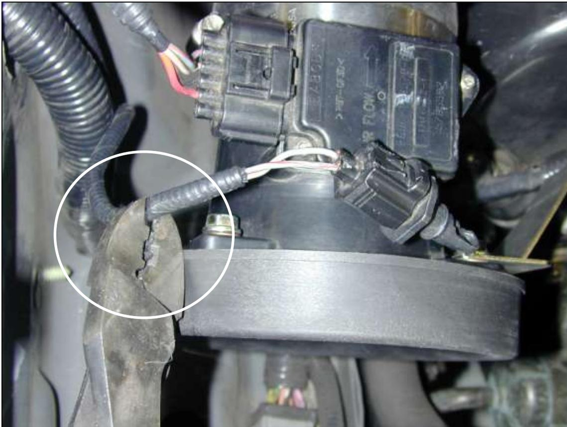
k. Locate the IAT sensor harness. Cut 3" down from the sensor to allow enough wire for crimping.
