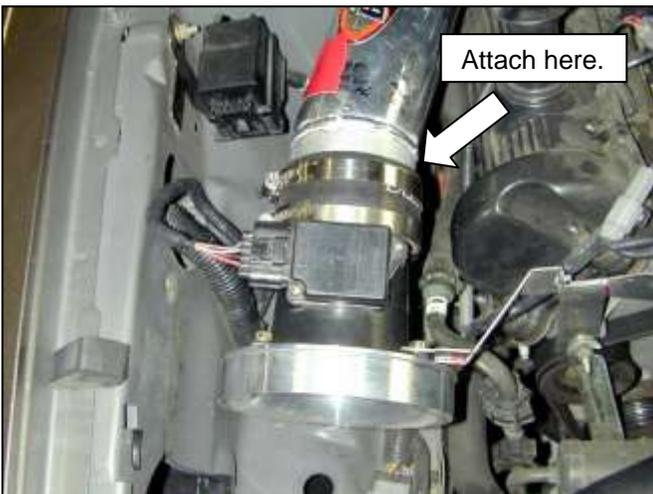
j. Attach the coupler to the inlet pipe. Plug in the MAF sensor harness.
