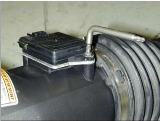
i. Use the supplied torx key to remove the MAF sensor. Save screws for later use.
