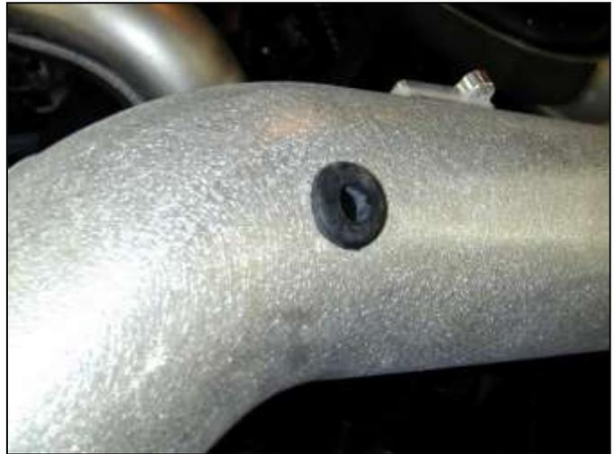
e. Install the supplied grommet in the inlet pipe.
