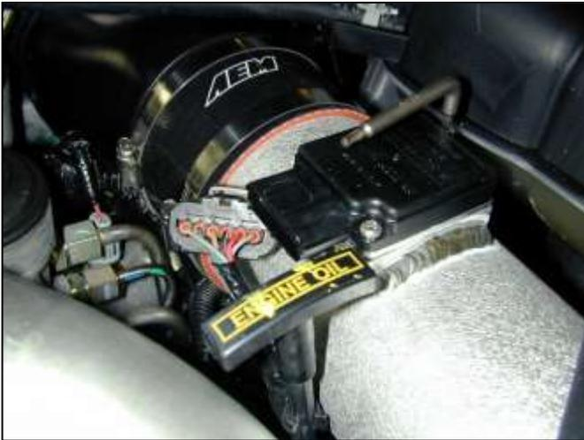
h. **Vehicle with a MAF Sensor:** Install the sensor into the intake pipe using the two factory bolts removed during step 2i. Proceed to step 3k.)
