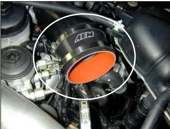
b. Install the supplied coupler as shown.
