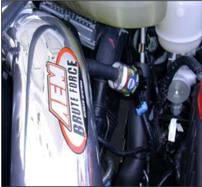
b. Install the air filter status meter assembly as shown.
