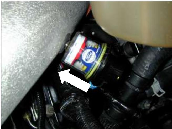
j. Install the air filter status meter into the rubber grommet on the rear of the pipe.
