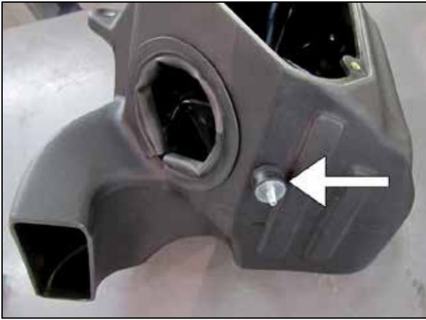
f. Install the supplied rubber mount (1228598) into the threaded insert on the front of the airbox.
