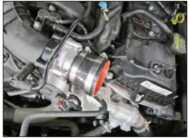
i. Install the throttle body coupler using one #48 hose clamp (9448) and one #56 hose clamp (9456).
