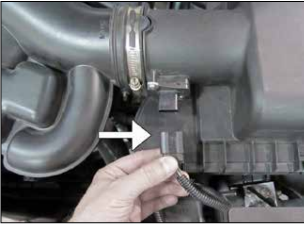
e. Unplug the MAF sensor connector.
