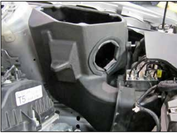
h. Ensure the inlet of the airbox engages the rubber part of the OEM inlet scoop.
