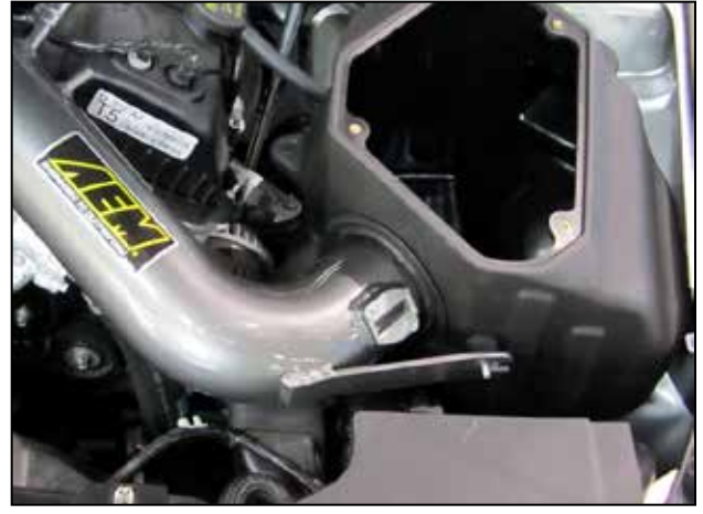
k. Insert the filter end of the intake pipe through the large hole in the airbox.
