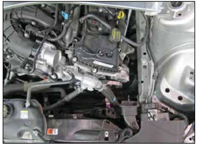
h. Lift up and remove the OEM airbox and inlet tube from the vehicle.
