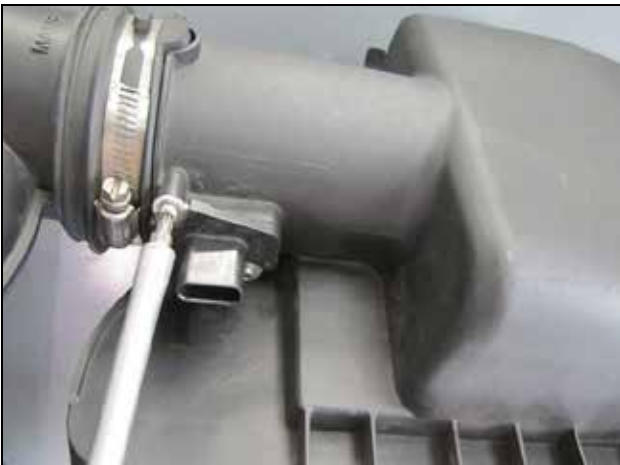
i. Remove the OEM MAF sensor from the OEM airbox and set it aside for future use.
