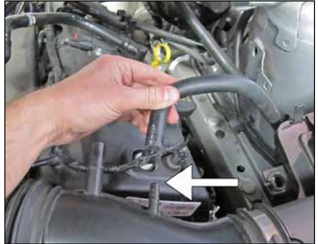
b. Disconnect the brake booster vacuum line.
