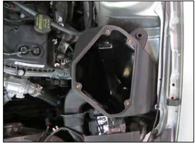
g. Lower the airbox assembly into position as shown. Ensure that the bosses on the bottom of the airbox are properly seated in the grommets that were installed in step 3b.
