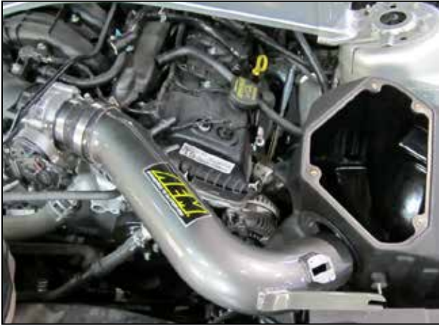
j. Position the intake pipe as shown. Insert the throttle body end of the pipe into the throttle body coupler as far as it will go.
