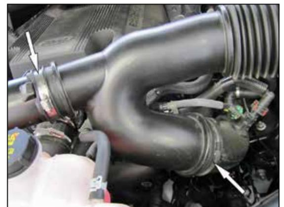
5. Loosen the two hose clamps that secure the factory intake tube to the turbo inlets and remove the factory tube from the vehicle.
