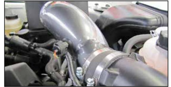
18. Reconnect the inlet air temperature sensor electrical connection.
