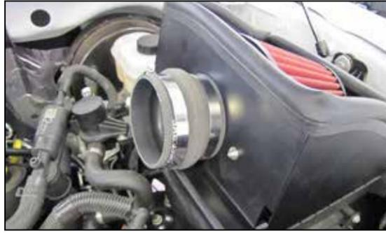
12. Install the provided hump coupler (08699) onto the filter adapter and secure with the provided hose clamp.
