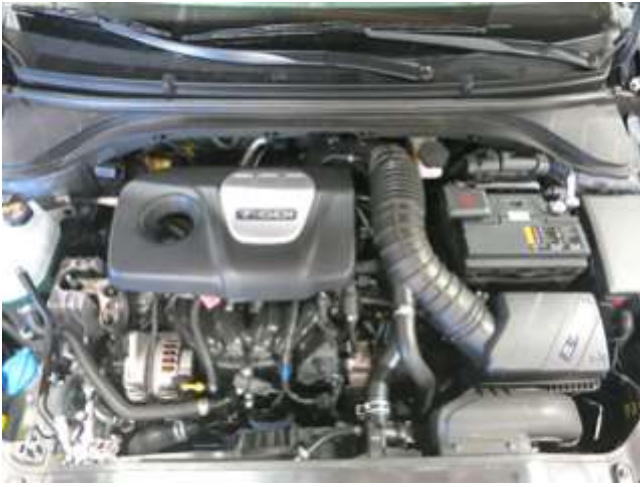
STOCK INTAKE INSTALLED
