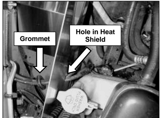
c. Pass both connectors through the supplied large grommet and then through the hole in the heat shield. Reconnect wire connectors and washer fluid hose to the washer fluid reservoir.
