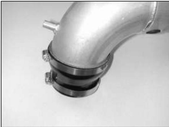
j. Loosely install the coupler and hose clamps on to the end of the AEM® inlet pipe nearest the vacuum nipple.
