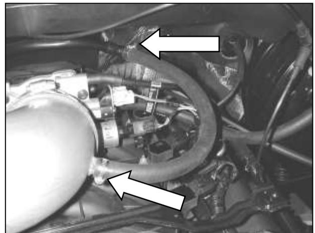
m. Install the supplied breather hose and secure with the two supplied hose clamps.
