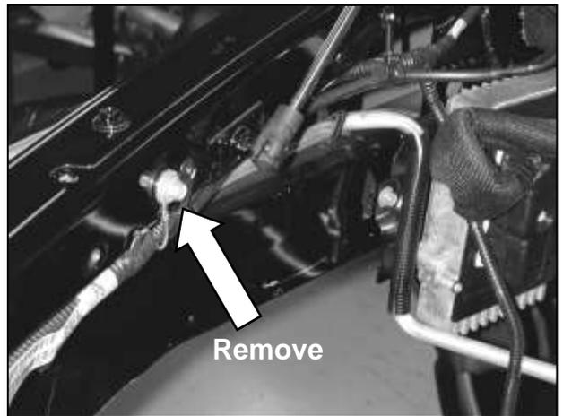
j. Remove the ground bolt located in front of the hood prop cylinder.
