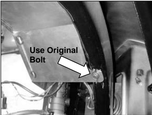
f. The lower heat shield mounting tab will line up with the lower air box mounting hole. Loosely secure the mounting tab with one of the original bolts.
