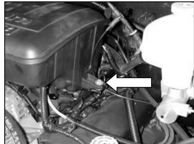
f. Remove the two bolts retaining the intake air resonator. One is located on the driver's side (pictured); the other is located near the oil dipstick.
