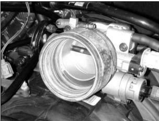
i. Remove the rubber adapter from the throttle body.
