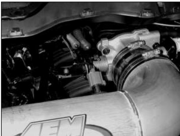
l. Reconnect the wire harness to the IAT sensor (if applicable). Do not push the grommet through into the pipe.
