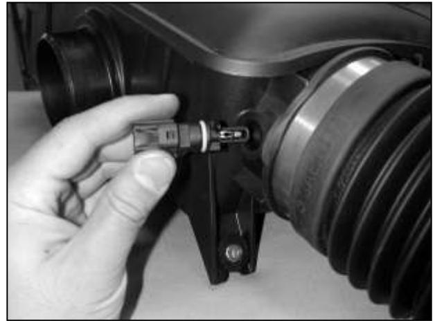
h. Remove the inlet air temperature (IAT) sensor from the intake resonator by gently twisting counter-clockwise. Remove the o-ring from the IAT sensor. Keep the o-ring for use if the vehicle ever needs to be returned to stock. (Except 2002 models)
