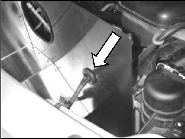
d. Install the rubber grommet in to the hole in the heat shield. Make sure the groove in the grommet is properly seated in the heat shield.
