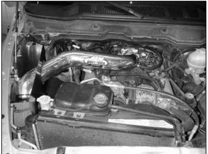
AEM<sup>®</sup> intake system installed
