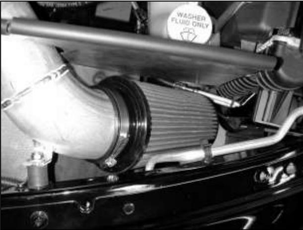
n. Install the AEM<sup>®</sup> air filter from inside the fender well. Slide the air filter on to the pipe until it stops. Secure with the supplied hose clamp. Make sure the windshield washer wires and hose do not come into contact with the air filter.
