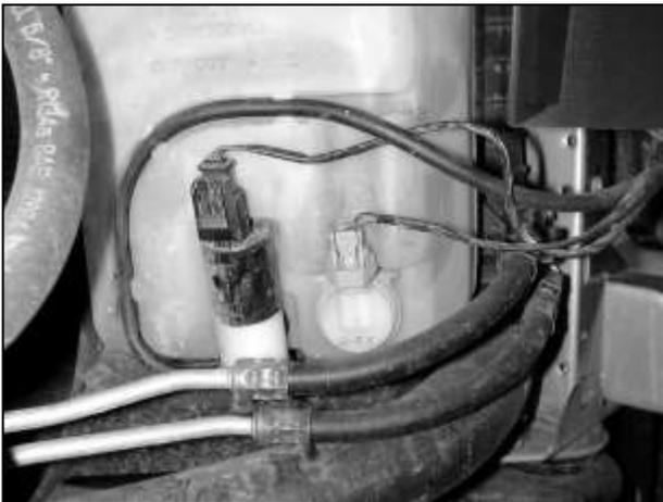
b. Unplug the wire connectors going to the windshield washer fluid pump and level indicator. Unplug the washer fluid hose. Block the nipple on the pump to prevent the washer fluid from draining.
