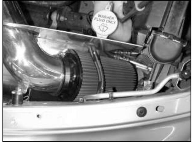
e. Reinstall the AEM<sup>®</sup> air filter. Adjust the windshield washer hose and wires so they do not rub against the AEM<sup>®</sup> air filter.
