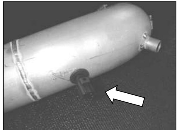
i. On models with an IAT sensor, install the supplied grommet into the AEM<sup>®</sup> inlet pipe. Insert the IAT sensor into the grommet. Use care to avoid pushing the grommet into the pipe.
