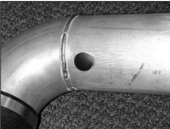
h. On 2002 models install the supplied polyethylene plug into the hole in the AEM<sup>®</sup> inlet pipe.
