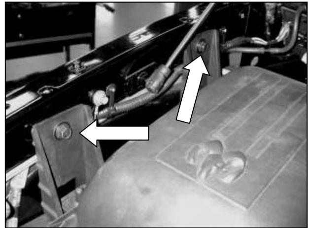
d. From inside the engine bay, remove the two remaining bolts securing the air box. Remove the air box from the engine bay.
