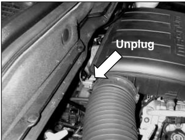
e. Unplug the inlet air temperature (IAT) sensor located on the back side of the intake air resonator (except 2002 models).
