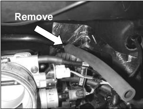
g. Disconnect the breather hose from the back of the resonator. Remove the resonator from the engine bay. Remove the breather hose from the tee near the back of the intake manifold. This hose will be replaced with one supplied with the AEM® intake kit.
