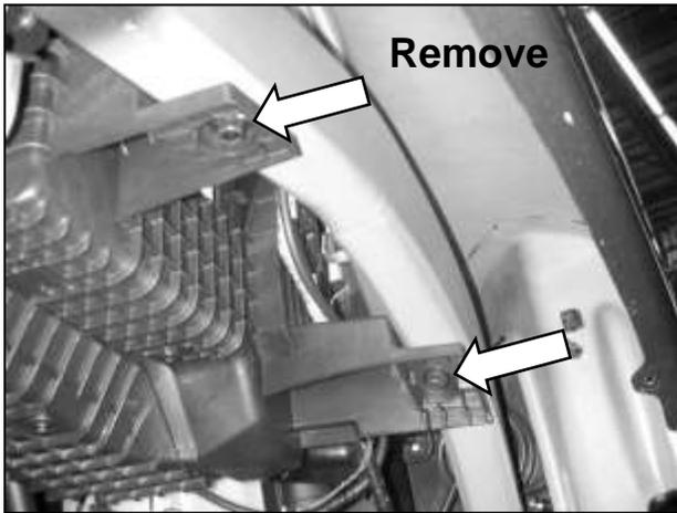
c. Remove the two bolts securing the bottom half of the air box.
