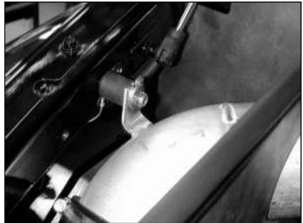
k. Install the bracket end of the AEM® inlet pipe through the cutout in the heat shield. Install the coupler on to the throttle body. The bracket will line up with the rubber mount installed in step 3b. Loosely secure the bracket with the supplied washer and locknut. Refer to the diagram below for proper rubber mount installation.
