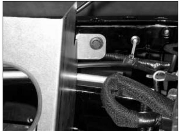
g. The rear mounting tab on the heat shield will line up with one of the lower air box mounting holes. Install one of the original bolts. Adjust the heat shield for best fitment then tighten the three mounting bolts.
