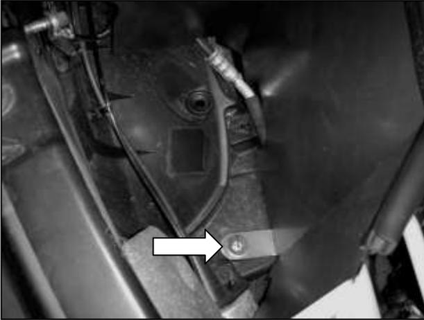
f. Place the heat shield in the engine bay. Gently push the heat shield bracket down into the rubber grommet.
