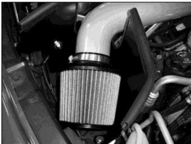
n. Insert the air filter onto the end of the intake pipe. Secure with the supplied hose clamp.
