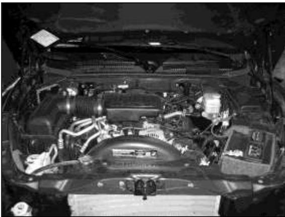
a. Stock air box system installed.
