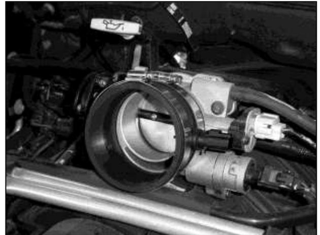
i. Place the #52 hose clamp on the smaller end of the reducer coupler. Attach the smaller end of the reducer coupler to the throttle body with the IAT sensor directed to the right of the throttle body.
