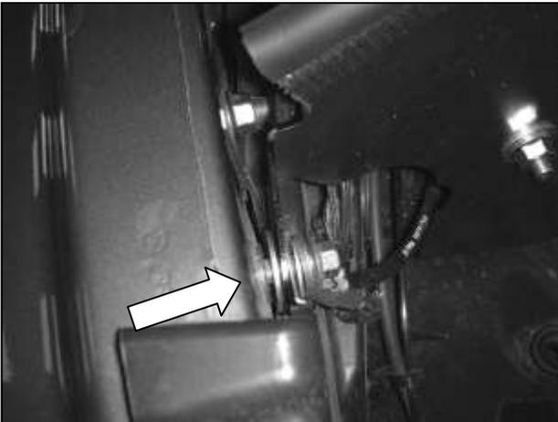
h. Place supplied spacer between the fender and the heat shield bracket. Secure with bolt.
