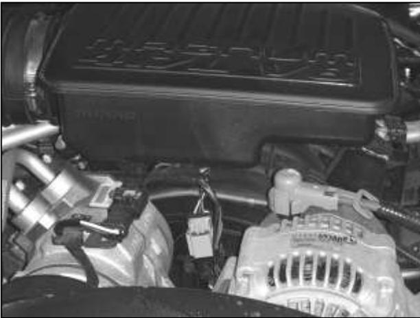
e. Remove the two resonator bolts.
