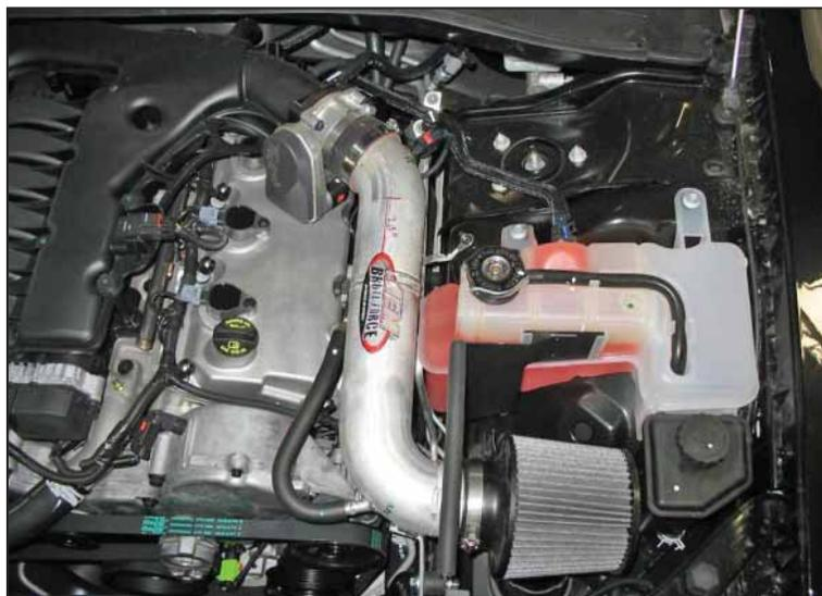
AEM® intake system installed
