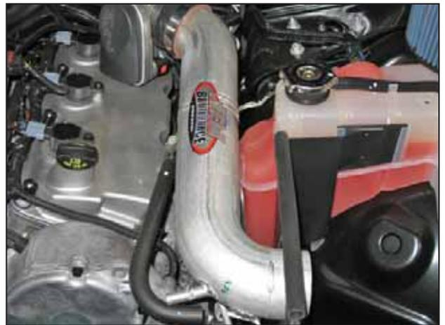
i. Insert the intake pipe as shown. Align the intake pipe bracket with the rubber mount.
