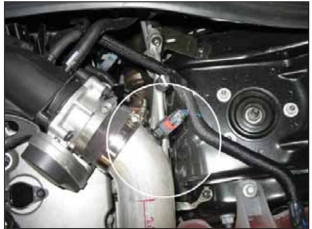
m. Insert the grommet for the IAT sensor into the intake pipe. Insert the IAT sensor and reattach the IAT sensor harness connector that was disconnected in step 2a. Secure the intake pipe to the throttle body coupler.
