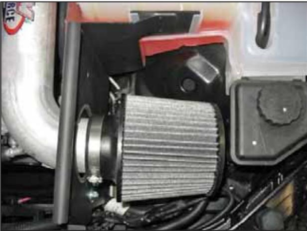
l. Attach the AEM® Dryflow™ air filter. Check for clearance around the rubber edge trim and secure.
