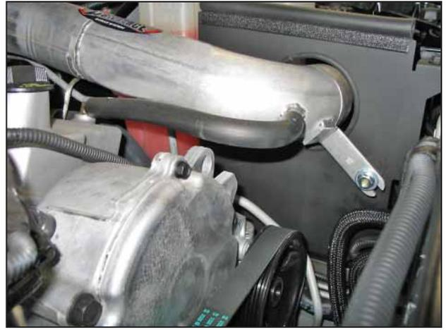
k. Reattach the PCV breather hose to the breather nipple on the intake pipe. Secure with a hose clamp.
