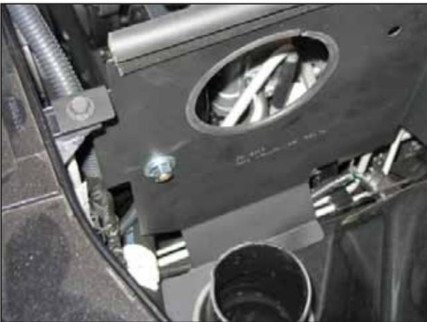
h. Secure the rubber mount with the M8 washer and nut.
