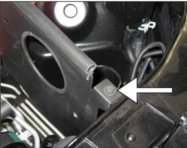
f. Secure the remaining tab with the factory screw.
