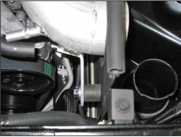
j. Once the bracket is aligned, check the intake pipe for clearance around the rubber edge trim. Secure the bracket with a M8 washer and nut.
