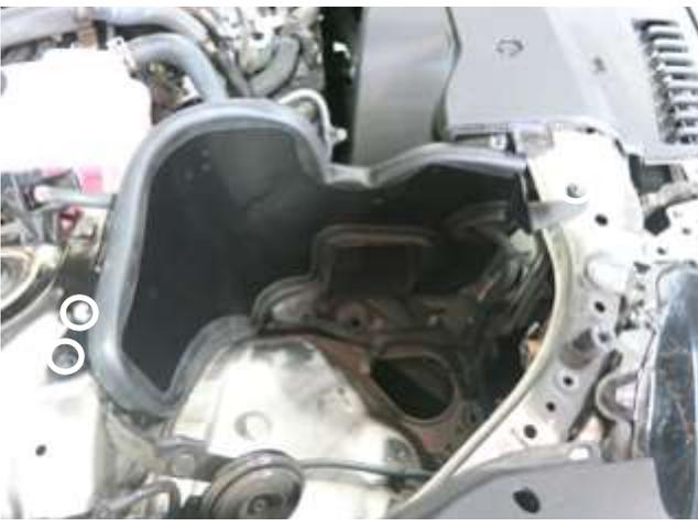
g. Place the heat shield into the engine bay. Make sure the cold air scoop is properly aligned in the heat shield cut-out. Then secure with the supplied M6 bolt and the [2] M6 bolts removed in steps 2i & 2j.
