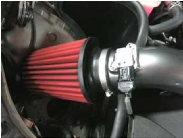
l. Install the AEM filter and tighten the hose clamp on the filter.
