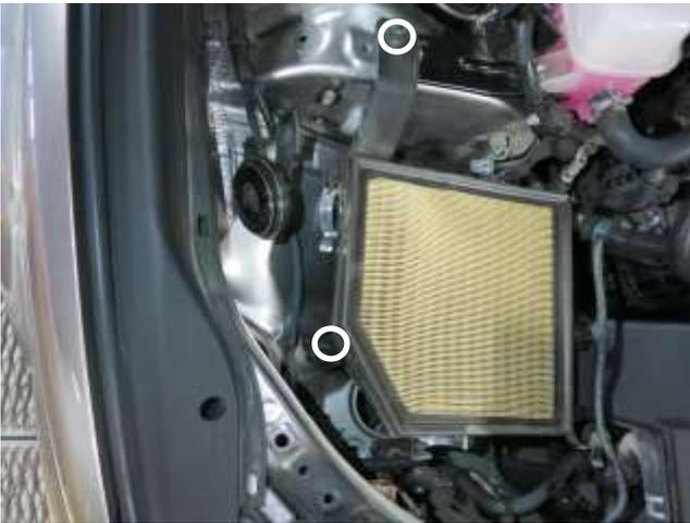
g. Remove the [2] M6 bolts securing the lower airbox.
