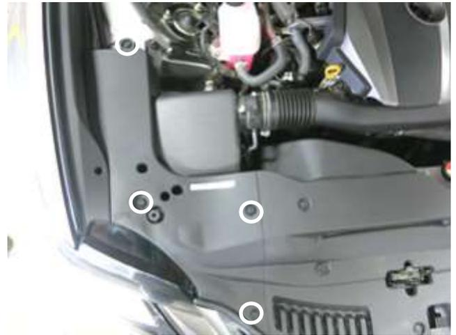
b. Remove the [4] retention clips by depressing the mandrel in the center. Then pull off the plastic shroud.
