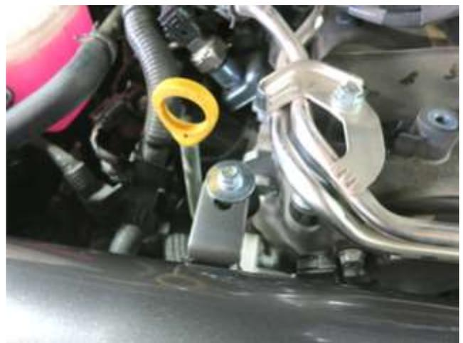
j. Align the mounting bracket to the rubber mount. Position the tube for best fit, then tighten the nut. Also, tighten, the hose clamp left loose in previous step.
