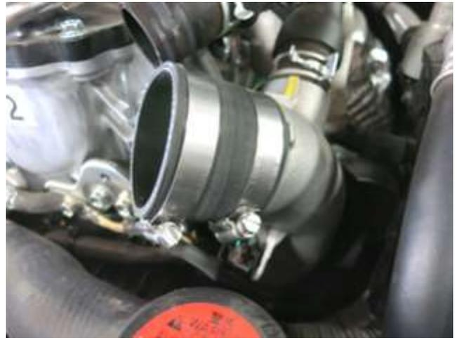
d. Install the coupler with hose clamps onto the turbo inlet pipe. Make sure the smaller end of the coupler is fitted to the turbo inlet side. Tighten the hose clamp on the turbo inlet side at this time.
