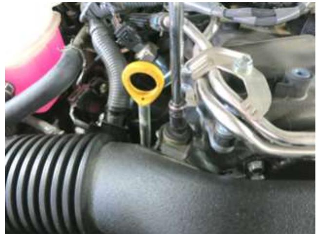
d. Remove the M6 bolt securing the factory intake tube.
