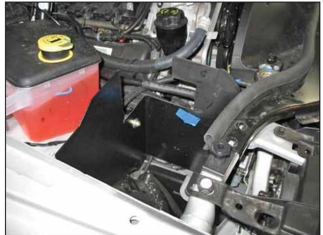
f. Insert heat shield as shown. Align the heat shield mount to the bottom bracket to the heat shield.
