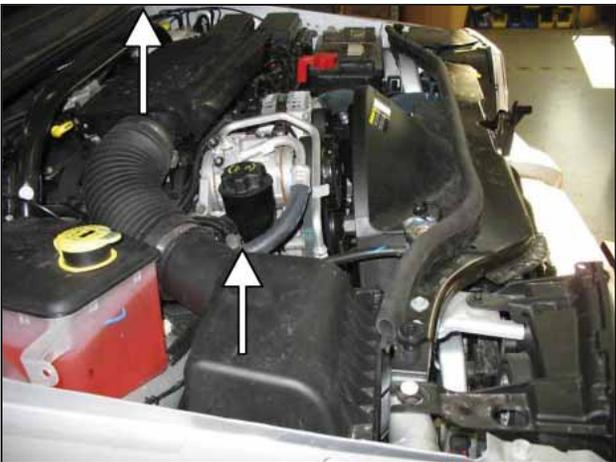
o. Remove the air box assembly.
