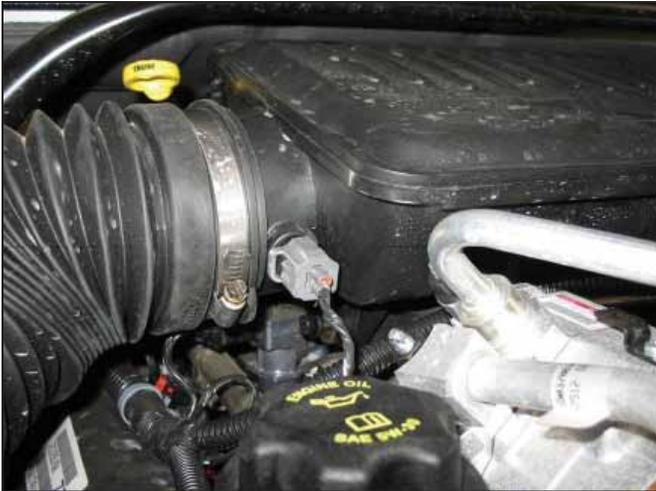
a. Disconnect the Inlet Air Temperature sensor.
