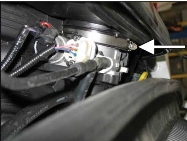
i. Loosen the throttle body hose clamp.
