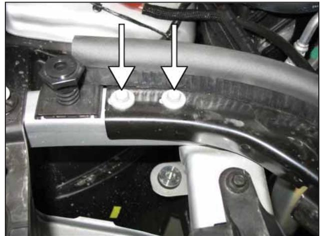
d. Loosen and remove the bolts to the hood latch support bracket. These will be reused.
