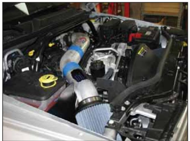
l. Insert the inlet pipe as shown.
