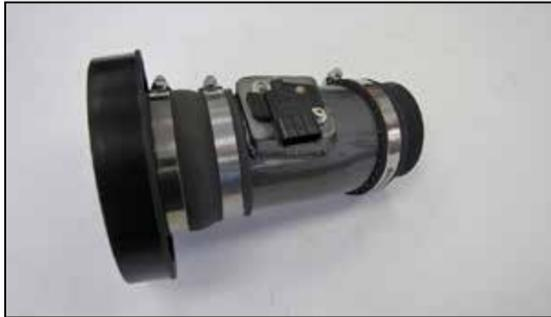
11. Install the filter adapter assembly onto the AEM® intake tube and secure with the provided hose clamp. Install coupler 084034 onto the AEM® intake tube and secure with the provided hose clamp.
