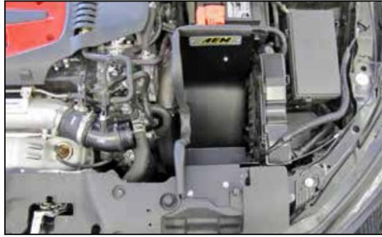
8. Set the heat shield into position on the rubber mounted studs and mounting stud. Secure the heat shield with the provided hardware.
