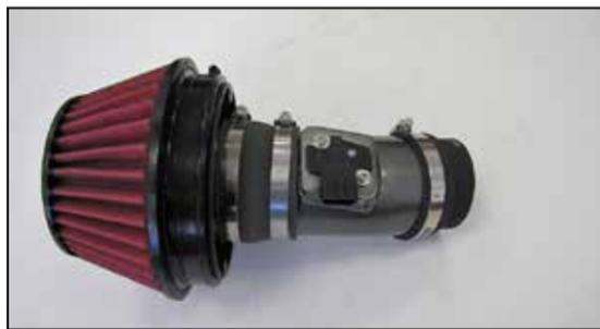
12. Install the AEM® air filter onto the filter adapter and secure with the provided hose clamp.
