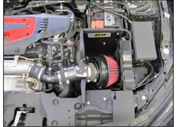
14. Reconnect the mass air sensor electrical connection.
