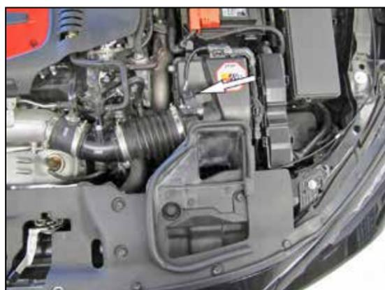
2. Disconnect the mass air sensor electrical connection and unhook the wiring harness from the air filter housing.
