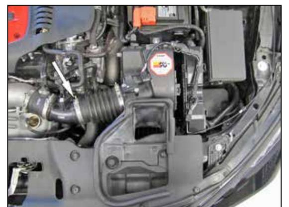
3. Release the clips that secure the upper air filter housing, loosen the hose clamp that secures the intake tube to the turbo inlet and then remove the upper air filter housing and intake tube from the vehicle.
