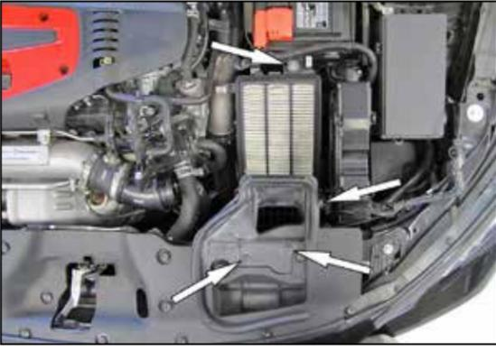
4. Remove the four bolts that secure the lower air filter housing and fresh air scoop to the vehicle and remove the complete assembly from the vehicle.
