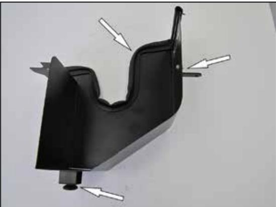
7. Install the factory mounting grommet, mounting bracket (064356) and edge trim onto the heat shield.
