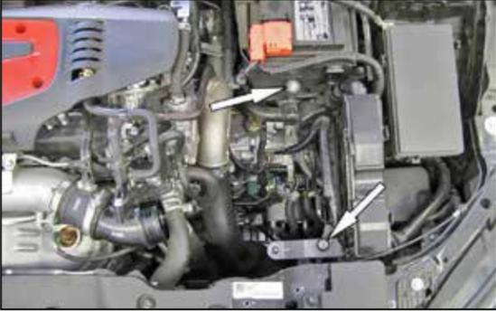
5. Install the two rubber mounted studs to the air filter housing mounting locations. Remove the plastic harness holder from the mass air sensor wiring harness and then install the provided split loom harness cover. Tape the ends of the harness cover with electrical tape.
