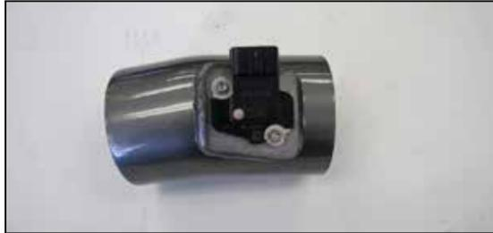
9. Remove the mass air sensor from the factory housing and install into the AEM® intake tube and secure with the provided hardware.
