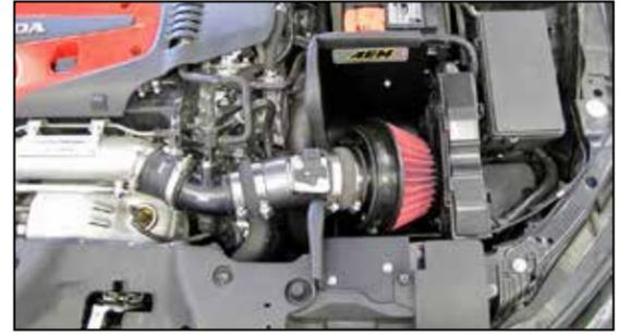
13. Install the intake tube assembly onto the turbo inlet, adjust the assembly for best fit and then secure with the provided hose clamp.
