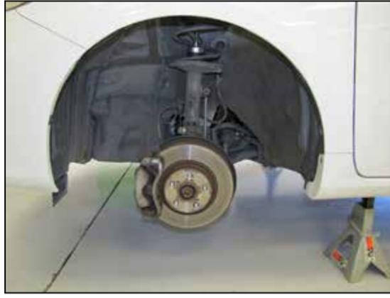
8. Place the vehicle on suitable jack stands and remove the left front tire. Remove the five clips and two bolts that secure the front of the inner fender and flex it back behind the brake assembly to gain access to the intake resonator.
