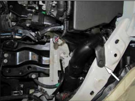
7. Remove the plastic retaining clip that secures the upper fresh air duct and then remove the duct from the vehicle.
