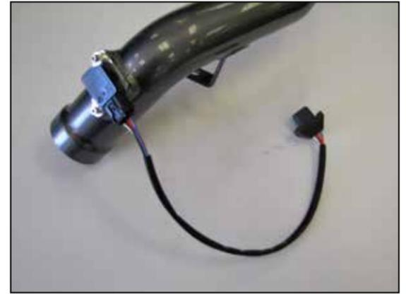
16. Connect the provided harness extension onto the mass air sensor.
