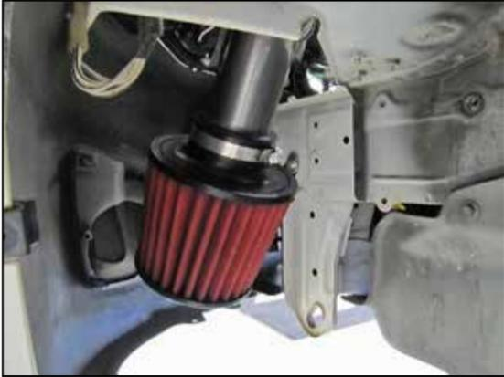
18. Install the AEM® air filter onto the intake tube and secure with the provided hose clamp. Reinstall the inner fender and secure with the factory hardware. Reinstall the tire and secure with the factory lug nuts. Lower the vehicle from the jack stands.
