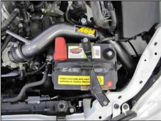
19. Reinstall the battery and hold down assembly, connect the positive battery cable.
