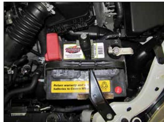
3. Disconnect the negative battery cable first, then remove the battery and hold down assembly from the vehicle.
