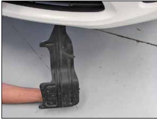
11. Remove the plastic air diverter from behind the bumper cover.
