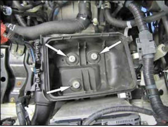
6. Remove the three bolts that secure the lower air filter housing. Disconnect the wiring harness from the mounting bracket. Remove the air filter housing from the vehicle.
