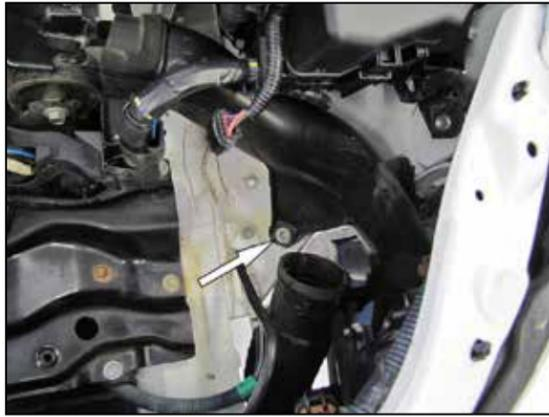
10. Remove the bolt that secures the lower fresh air intake tube and then remove the tube from the vehicle.
