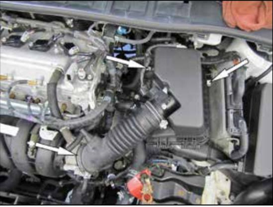
5. Disconnect the mass air sensor electrical connection and unhook the wiring harness from the factory air filter housing. Loosen the hose clamp securing the intake tube to the throttle body and unclip the air filter housing retaining clips. Remove the upper air filter housing and intake tube from the vehicle.
