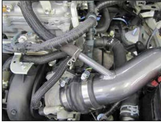
20. Connect the crankcase vent hose and secure with the factory spring clamp.
