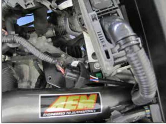
21. Connect the factory mass air harness to the AEM® extension harness and secure with the provided tie wrap.
