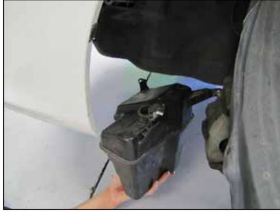
9. Remove the two bolts and one nut which secure the intake resonator to the vehicle and then remove the resonator from the vehicle.
