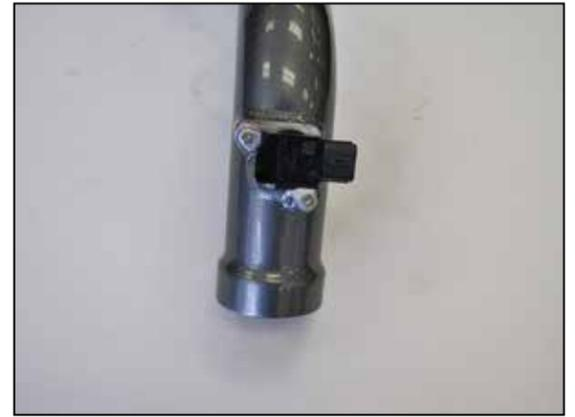
15. Remove the mass air sensor from the factory air filter housing and install into the AEM® intake tube using the provided hardware.
