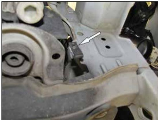
12. Install the provided clipnut onto the core support as shown.
