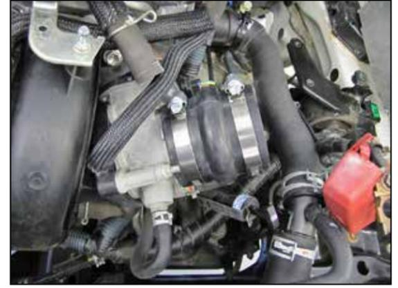
14. Install the provided hump coupler (5-525) onto the throttle body and secure with the provided hose clamp.
