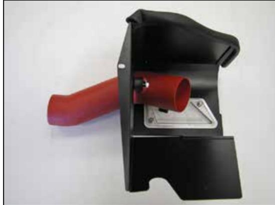
10. Install the intake tube through the heatshield and secure with the provided rubber mounted stud and hardware.
