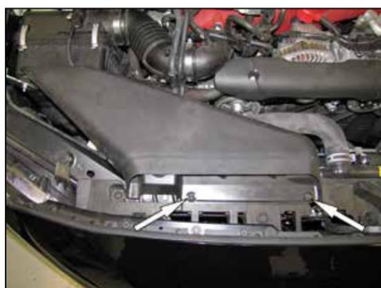
2. Remove the two plastic retaining clips that secure the fresh air duct and then remove the fresh air duct from the vehicle.
