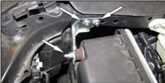
5. Remove the three nuts that secure the air filter housing to the inner fender and then remove the bracket from the vehicle.
