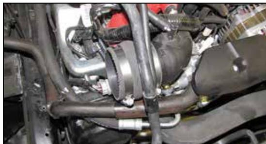
12. Install the provided hump coupler (08185) onto the turbo inlet and secure with the provided hose clamp.
