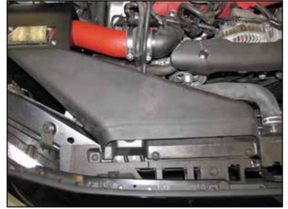
14. Install the fresh air duct and secure with the factory hardware.
