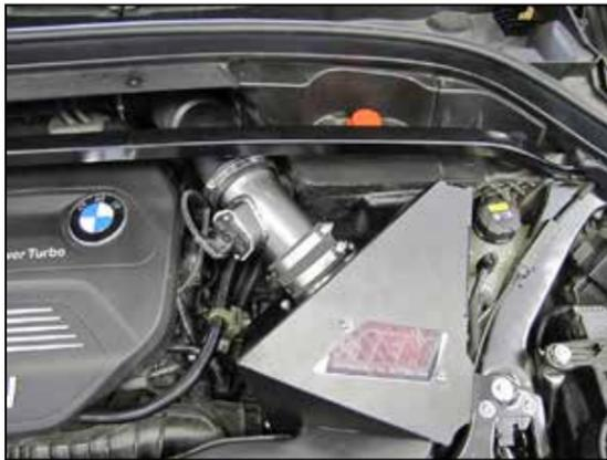
11. Install the provided coupler onto the intake tube but do not secure. Install the intake tube assembly into the factory intake hose and align with the filter adapter, slide the coupler onto the adapter and adjust the assembly for best fit. Secure the intake tube assembly with the provided hose clamps. Reconnect the mass air sensor electrical connection.
