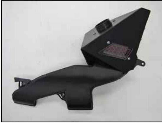
8. Install the AEM® badge into the upper air filter housing and then assemble the two filter housing halves and fresh air scoop and secure with the provided hardware.
