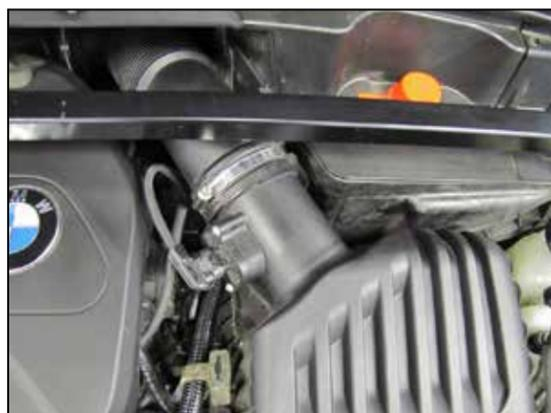
2. Disconnect the mass air sensor electrical connection and disconnect the wiring harness from the air filter housing.
