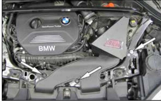
9. Install the air filter assembly into the vehicle and secure with the factory fresh air scoop nuts and the bolt provided.
