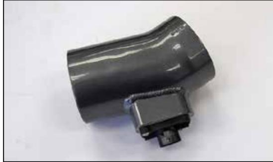
10. Remove the mass air sensor from the factory housing and install it into the AEM® intake tube using the hardware provided.
