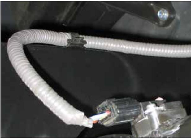
n. Secure the tree mount zip tie into the heat shield's slot as shown. Connect the MAF wiring harness plug to the MAF sensor.
