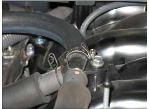
i. Install the provided 5/8" hose onto the breather hose inlet and secure with a hose clamp.
