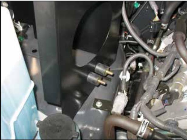
h. Insert the two rubber mounts into the heat shield as shown. Secure the rubber mounts to the inner side of the heat shield with a washer and serrated nut.
