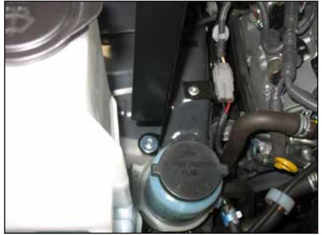
g. Assemble a washer to the long bolt (#1-2075). Guide the bolt through the heat shield tab, spacer, and windshield washer bottle support. Tighten the hardware to secure the heat shield to the vehicle.
