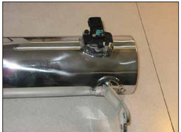
k. Remove the MAF sensor from the stock inlet tube and install it in the AEM® intake pipe. Use the stock screws to secure the MAF sensor to the intake pipe.
