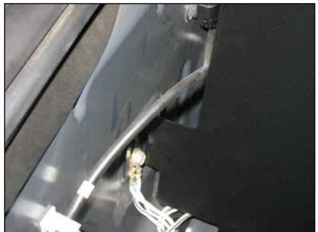
e. Align the third heat shield tab with the bolt hole that was exposed from removing a ground strap in step 2p.
