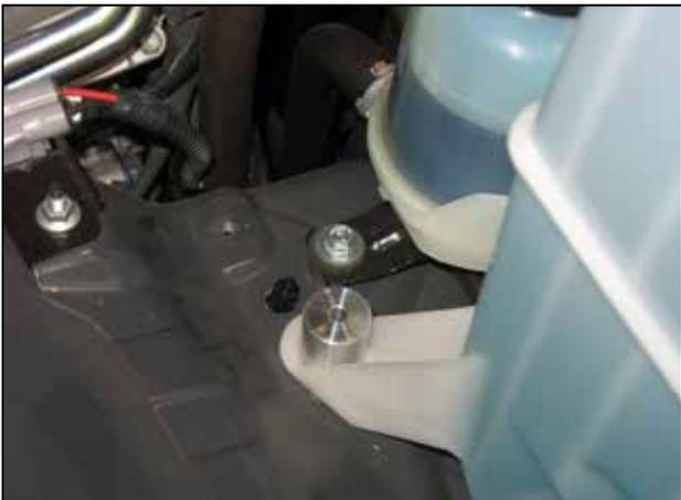
b. Install the supplied spacer over the windshield washer fluid container support.
