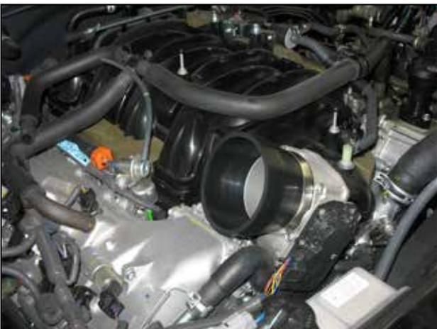
j. Install the reducer coupler onto the throttle body and secure with the provided hose clamp.
