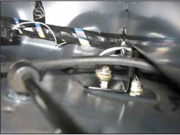
f. Using the bolt removed in step 2p, secure the ground strap and heat shield tab to the inner fender.
