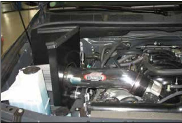
p. Attach the edge trim to the top of the heat shield edges as shown.
