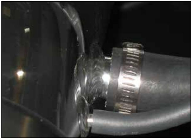
m. Route the open end of the 5/8" breather hose to the intake pipe nipple and secure in place with the supplied hose clamp. Route the stock 5/32" hose to the same location, it should slide snugly over the intake pipe's smaller nipple.
