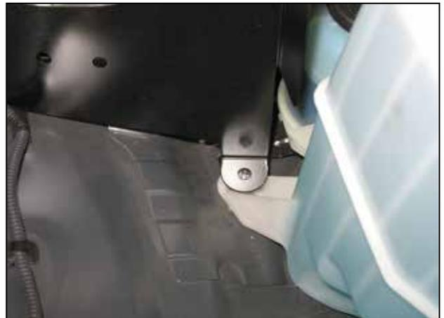
c. Insert the heat shield into the engine bay, aligning the heat shield's tab with the spacer installed in step 3b.
