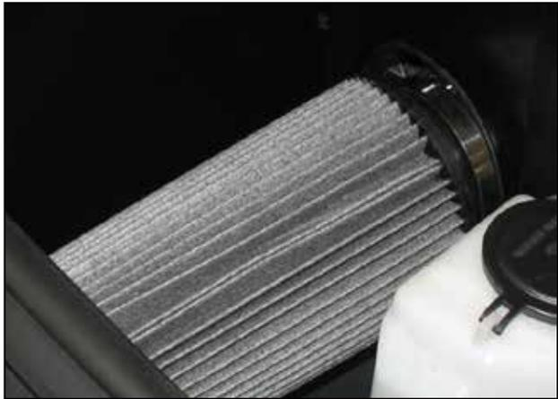
o. Install the supplied edge trim around the heat shield opening. Position the AEM® air filter into the heat shield opening and secure to the intake pipe with a provided hose clamp.
