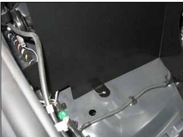
d. Align the second heat shield tab with the fender well hole as shown. Secure the heat shield in place by securing the tab to the fender well with a supplied bolt and washer.
