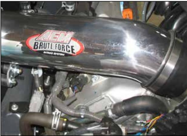
l. Insert the intake pipe into the reducer coupler while also aligning the intake pipe's bracket to the rubber mounts protruding from the heat shield. Secure the intake pipe to the reducer coupler with a provided hose clamp and secure the intake pipe's bracket to the rubber mounts with the provided washers and serrated nuts.
