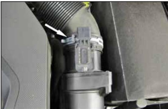
6. Release the spring clamp that secures the factory intake tube to the mass air sensor housing and then disconnect the hose from the sensor.
