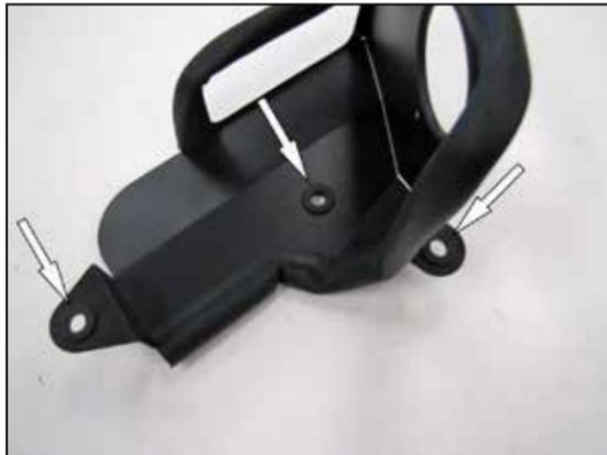
11. Install the three provided mounting grommets into the heat shield where shown.
