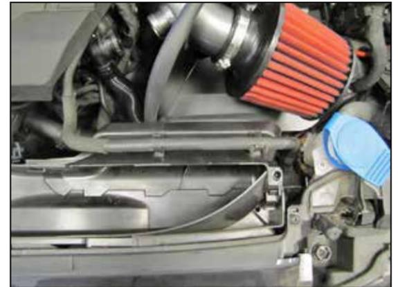
17. Reinstall the lower fresh air duct.
