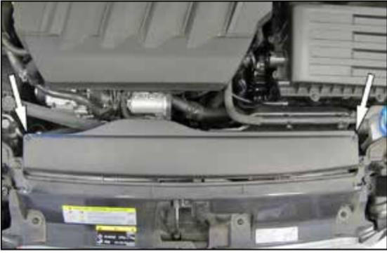
4. Remove the screws that secure the top of the fresh air duct and then remove the top from the vehicle.
