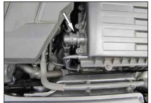
3. Disconnect the air injection hose from the upper air filter housing.
