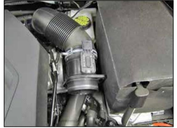
14. Reinstall the factory mass air sensor onto the factory intake tube and secure with the factory spring clamp.
