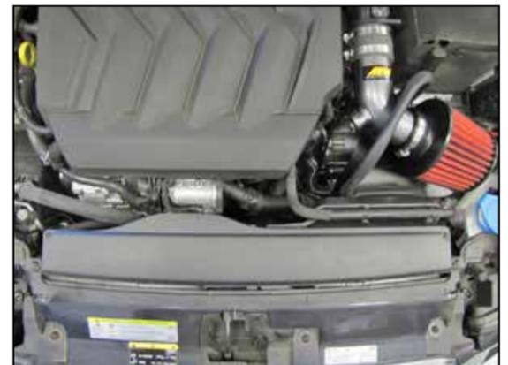
18. Reinstall the upper fresh air duct and secure with the factory hardware.
