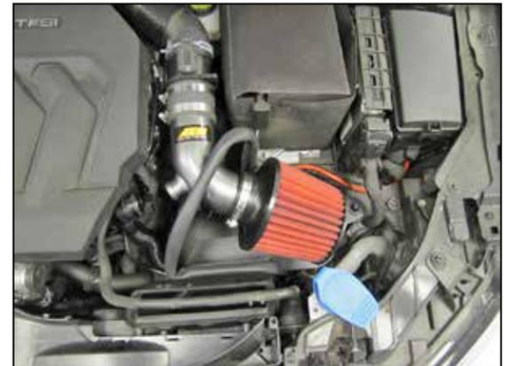
16. Install the AEM® intake kit so the grommets align with the mounting studs, connect the mass air sensor to the intake tube. Adjust the intake tube and filter for best fit and secure with the provided hardware and clamps.
