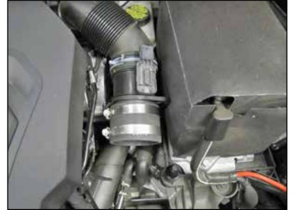
15. Install the provided coupler (08440) onto the mass air sensor and secure with the provided hose clamp.
