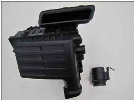
8. Remove the mass air sensor from the factory air filter housing.
