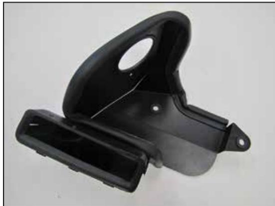
12. Install the factory fresh air duct into the heat shield as shown.
