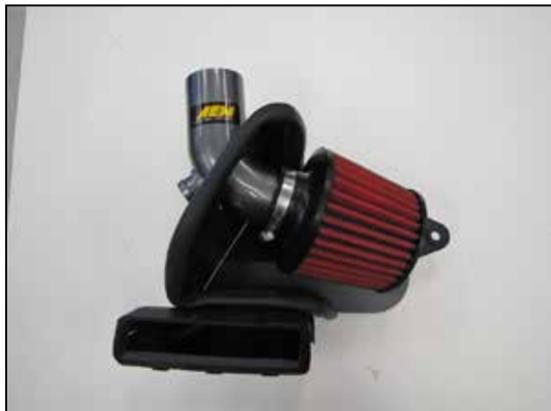
13. Install the rubber mounted stud into the heat shield and secure with the provided hardware. Install the AEM® intake tube into the heat shield and secure to the rubber mounted stud with the provided hardware. Install the AEM® air filter onto the intake tube and secure with the provided hose clamp.
