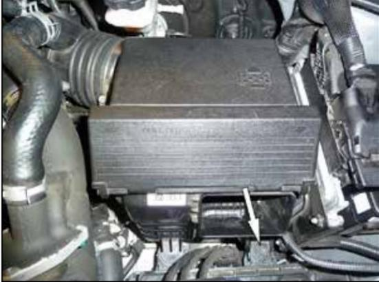
5. Remove the bolt that secures the air filter housing into the vehicle and then remove the air filter housing from the vehicle.
