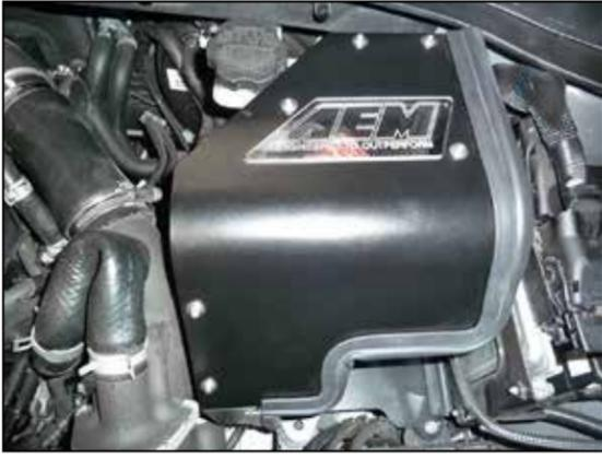
19. Install the AEM® air filter assembly so the mounting studs insert into the mounting grommets and then secure to the rubber mounted stud using the provided hardware.
