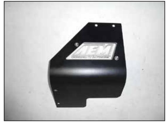
14. Install the provided window logo into the heat shield lid and secure with the provided hardware.
