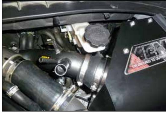
22. Install the AEM® intake tube into the couplers, align the tube for best fit and then secure with the provided hose clamps.
