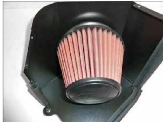
13. Install the air filter onto the adapter and secure with the provided hose clamp.
