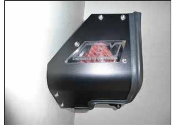
16. Install the lid onto the heat shield and secure with the provided hardware.
