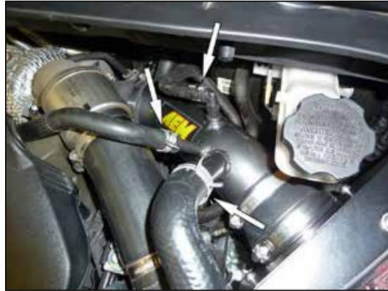
23. Connect the 3 vent lines to the fittings in the intake tube and secure with the factory spring clamps.
