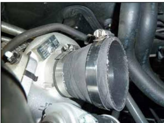
8. Install the provided coupling hose (08188) onto the turbo inlet and secure with the provided hose clamp.
