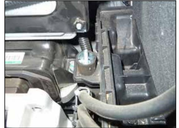
18. Install the provided rubber mounted stud onto the factory air filter housing mounting location as shown.
