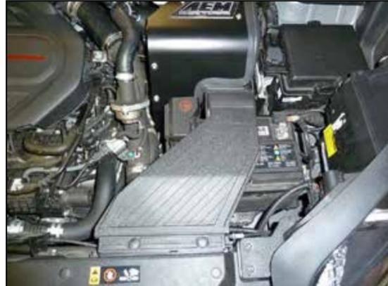
24. Reinstall the fresh air intake duct and secure with the factory retaining pins.
