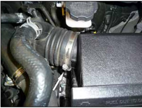
4. Loosen the hose clamp that secures the intake tube to the air filter housing.
