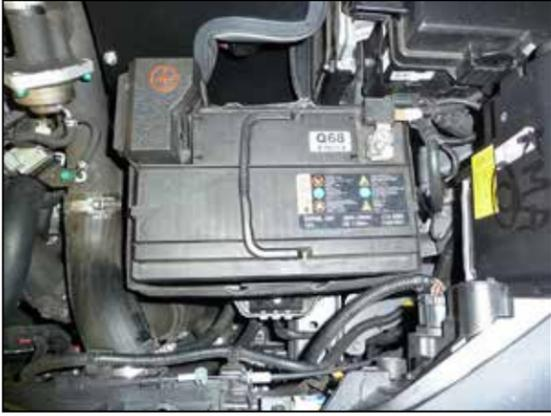
20. Slide the battery back into position and secure with the factory hardware.
