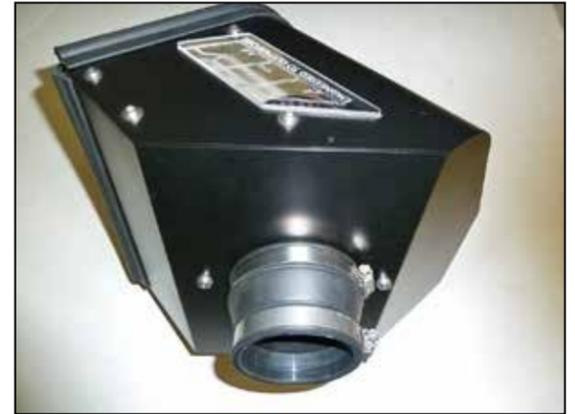
17. Install the provided coupler (084055) onto the filter adapter and secure with the provided hose clamp.
