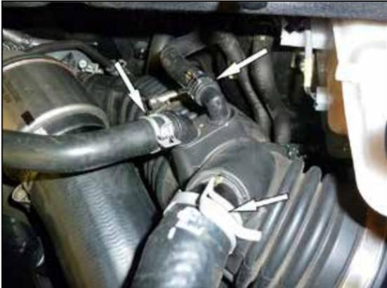
6. Release the spring clamps that secure the vent lines to the factory intake hose and then disconnect the vent lines from the intake hose.
