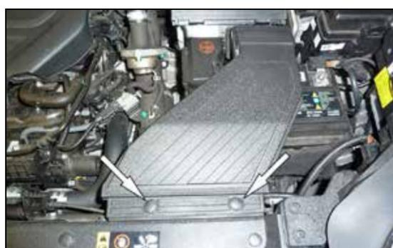
2. Remove the two pins that secure the fresh air intake duct to the core support and then remove the fresh air intake duct from the vehicle.
