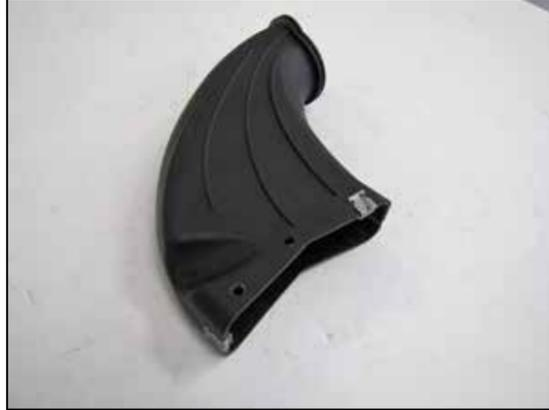
23. Install the two clips from the previous step onto the AEM® fresh air duct in the same position as the factory.
