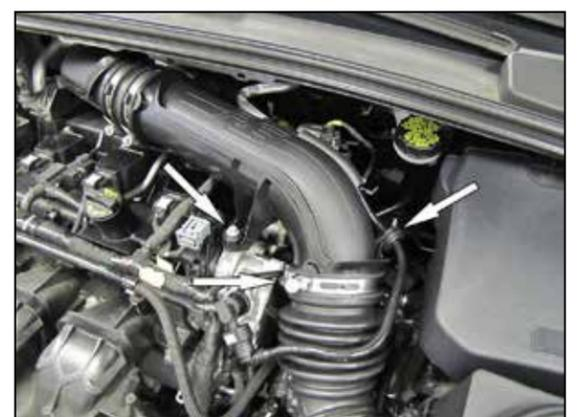
3. Remove the bolt securing the factory intake tube to the engine shown. Next loosen the hose clamps and unhook the vent line from the intake tube and remove the intake tube from the vehicle.
