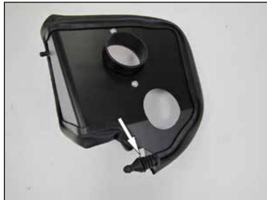
12. Install the mounting post from the previous step onto the AEM® heat shield as shown.
