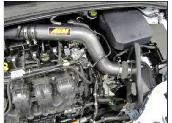
17. Install the AEM® intake tube into the factory coupler and then into the AEM® coupler, adjust the tube for best fit and then secure with the provided hose clamps.
