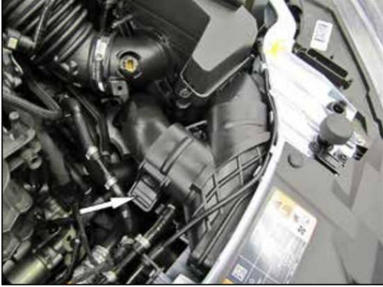
5. Release the inlet air duct from the air box.
