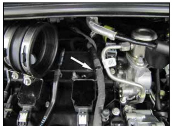
16. Unhook the wiring harness clip from the mounting stud, route the harness next to the coil and fuel line and secure the harness to the fuel line with the provided tie wrap.
