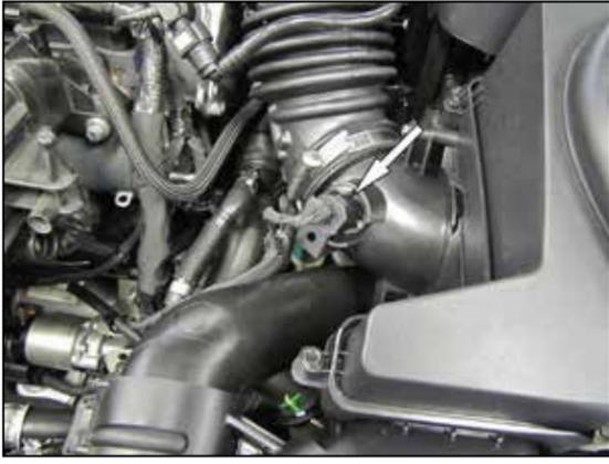
4. Disconnect the inlet air temperature sensor electrical connection.
