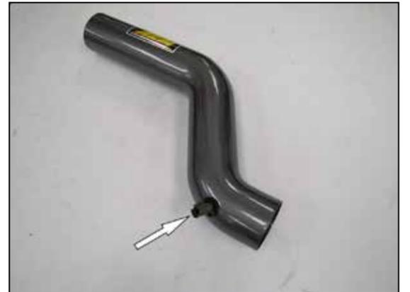
15. Install the grommet provided and the factory inlet air temperature sensor into the AEM® intake tube as shown.
