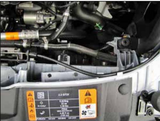
21. Using the Fresh air duct as a guide, mark the two hole locations onto the fresh air duct in the core support. Next remove the AEM® fresh air duct and drill two ¼" id holes into the factory fresh air duct at the marked locations.
