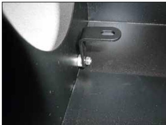
12. Install the provided "L" bracket (070015) onto the heat shield using the provided spacer between the bracket and heat shield and hardware.
