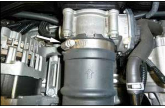
4. Loosen the hose clamp securing the intake hose to the throttle body.
