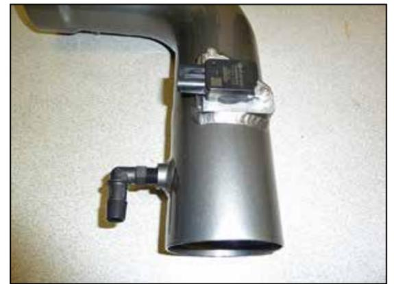
17. Remove the mass air sensor from the factory air filter housing and then install it into the AEM® intake tube using the provided hardware. Install the provided 90° vent fitting into the AEM® intake tube as shown.
