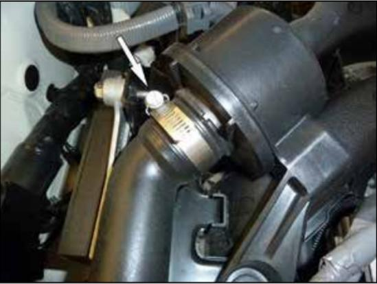
5. Loosen the hose clamp and disconnect the engine sound tube from the engine sound drum.
