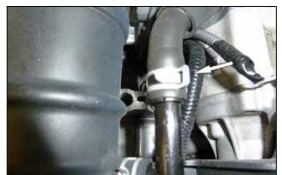
3. Release the spring clamp and then disconnect the crank case vent hose from the fitting.
