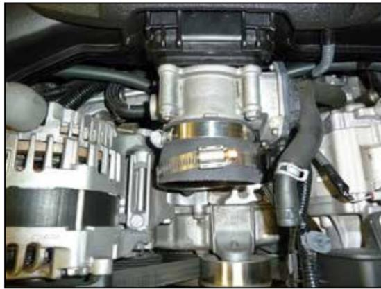
9. Install the provided coupling hose (08186) onto the throttle body and secure with the provided hose clamp.
