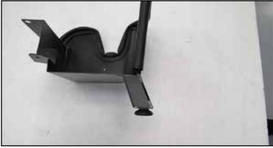
7. Remove the mounting grommet from the factory air filter housing and install it into the AEM® heat shield as shown.
