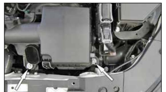
5. Remove the two bolts that secure the air filter housing and then lift up the intake assembly to remove it from the vehicle.
