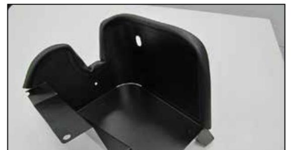
6. Install the provided edge trim onto the heat shield as shown, some trimming of the edge trim will be necessary.
