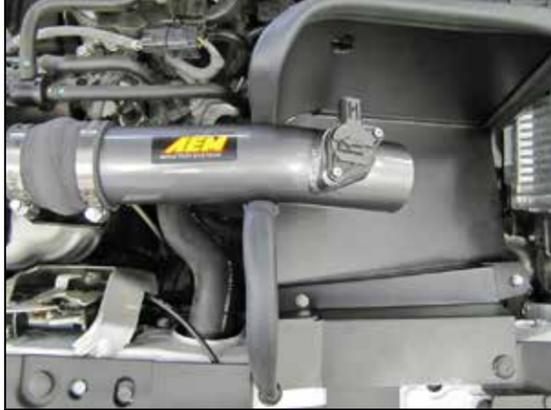
12. Install the AEM® intake tube into the coupler at the turbo inlet and then align the mounting stud with the hole in heat shield. Adjust the intake tube for best fit and then secure with the provided hardware and hose clamp.
