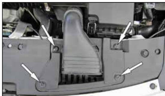
4. Remove the four pins that secure the fresh air intake to the core support.
