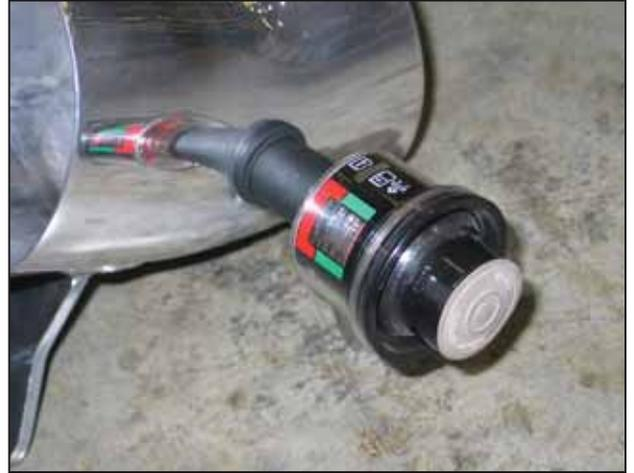
i. Install the previously removed air filter restriction gauge into the rubber adapter in step 3h.
