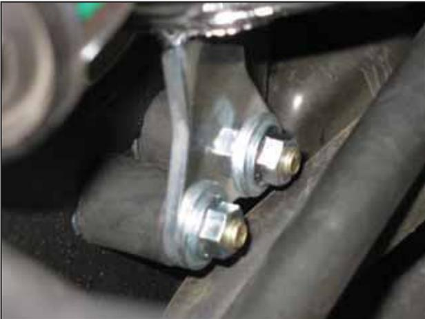
l. Slide the lower intake pipe and reducing coupler down from the upper intake pipe until the mounting bracket face is flush with the rubber mounts. Install the remaining M8 washers and nuts to secure the lower pipe's mounting bracket.
