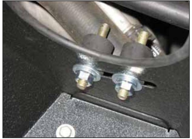
g. Install the two supplied rubber mounts into the slot on the heat shield using two M8 nuts and washers. Secure the mounts with just enough slack for the mounts to slide in the slot.
