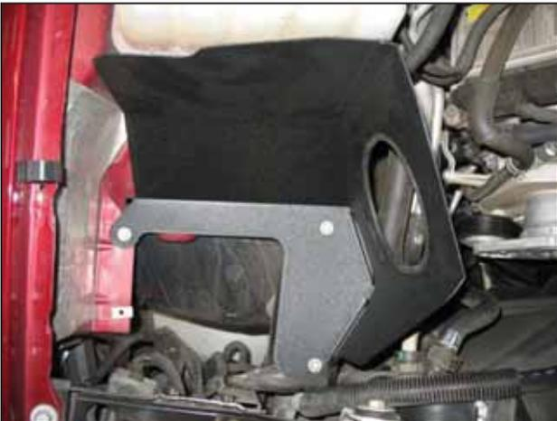
d. Install the heat shield in the engine bay, aligning the holes with the mounting plate bolt locations. Secure it using three of the bolts removed in step 2f.
