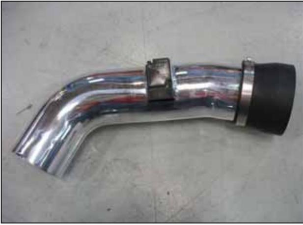
f. Install the reducing coupler onto the upper intake pipe as shown. Slide the coupler all the way onto the intake pipe with a #56 hose clamp; do not tighten the hose clamp.
