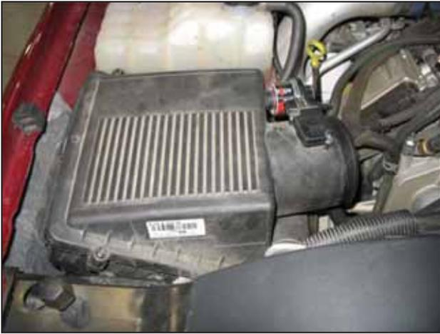
e. The air filter housing is held in place by two grommets on the mounting plate. Gently lift up on the air filter housing and remove it from the engine bay.
