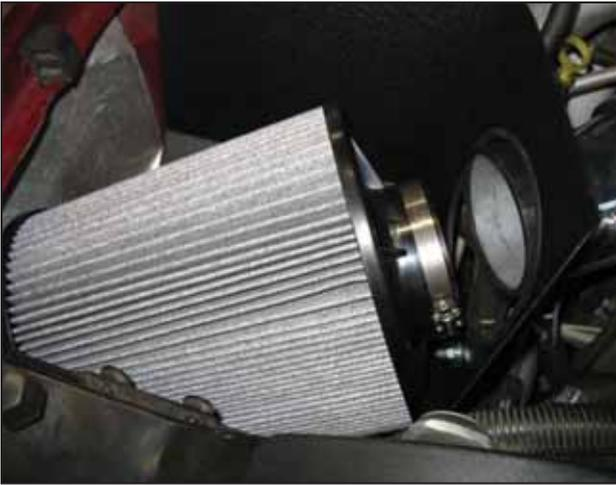
j. Slide the air filter into the heat shield with the filter neck facing the engine. This will ease installation, as the air filter cannot easily be installed if the lower intake pipe is already installed.
