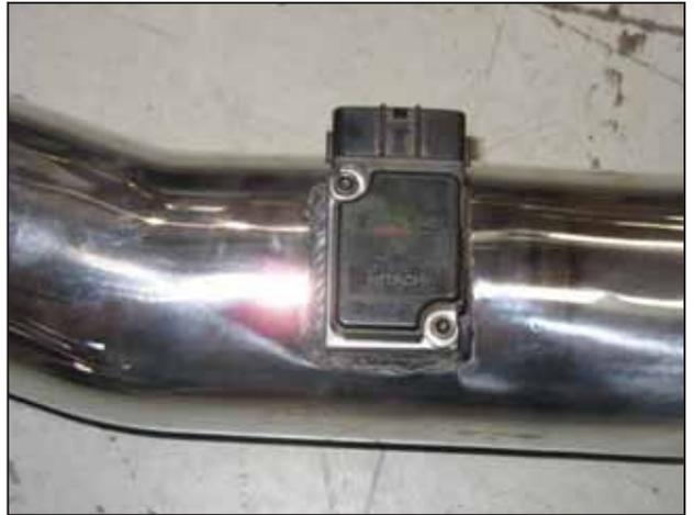
c. Install the previously removed MAF sensor into the upper intake pipe using the two supplied 8-32 bolts.
