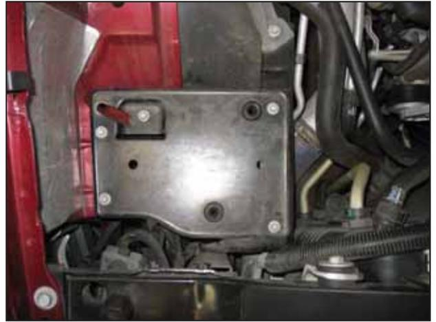
f. Remove the five bolts securing the air filter housing mounting plate to the vehicle chassis.
