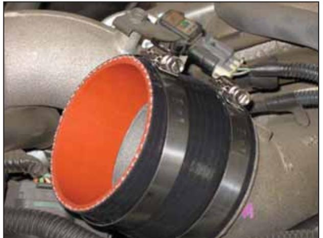
e. Install the 3.50" coupler onto the turbo inlet. Loosely secure the coupler with the supplied #56 hose clamps.
