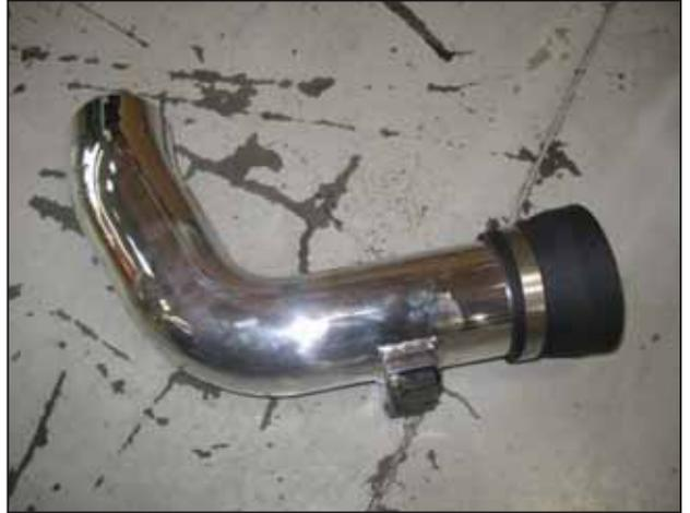
c. Install the previously removed MAF sensor into the upper intake pipe using the two supplied 8-32 bolts. Install the reducing coupler and #56 hose clamp onto the straight side of the upper intake pipe.
