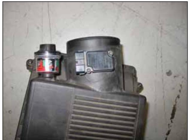
h. Remove the factory air filter restriction gauge from the stock air filter housing.
