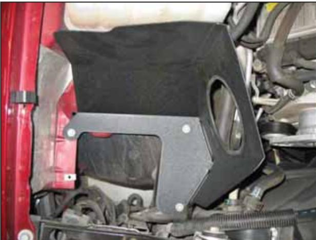
d. Install the heat shield in the engine bay aligning the holes with the mounting plate bolt locations. Secure it using three of the bolts removed during step 2f.
