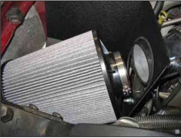
j. Lower the air filter into the heat shield bay with the filter neck facing the engine. This will ease installation, as the air filter cannot easily be installed if the lower intake pipe is already installed.
