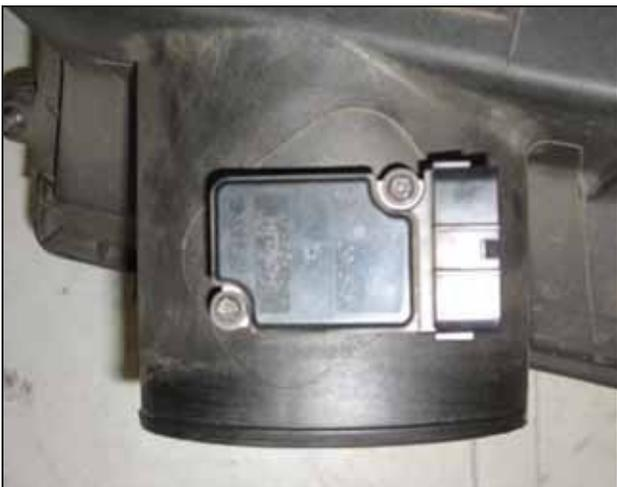
i. Using the supplied tamper-proof torx key, remove the two bolts securing the MAF sensor to the air filter housing. Carefully remove the MAF sensor from the housing.
