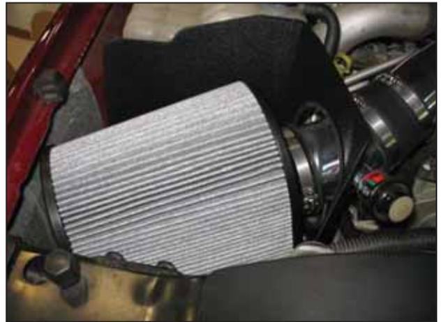
m. Slide the hose clamp onto the air filter's neck and attach the air filter assembly onto the filter adapter. Ensure the air filter is completely seated onto the adapter and the hose clamp is aligned with the filter adapter's lip. Once the hose clamp is properly aligned, secure the hose clamp, ensuring the filter neck's tabs compress and engage the filter adapter. Ensure the air filter does not make contact with any part of the vehicle and has adequate clearance.
