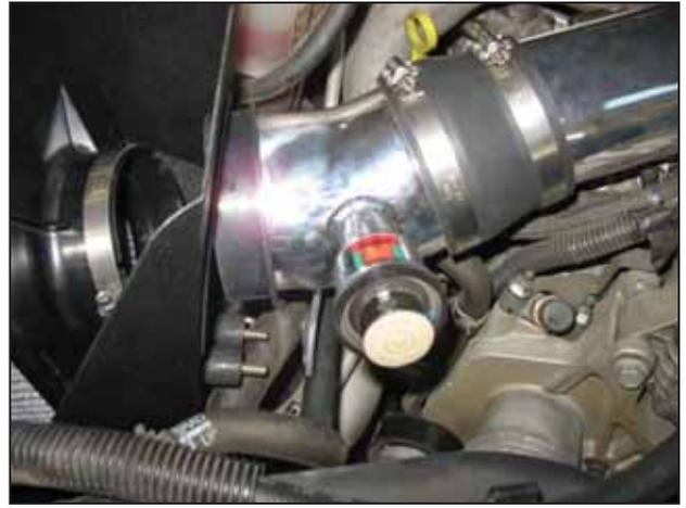
k. Install the lower intake pipe by aligning the two holes in the mounting bracket with the two rubber mounts installed on the heat shield. Slide the reducer coupler over the lower intake pipe and secure using a #64 hose clamp.
