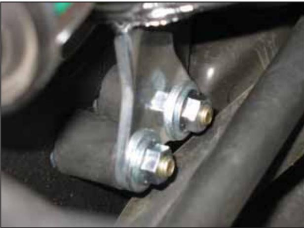
l. Slide the lower pipe and reducing coupler down the upper pipe until mounting bracket face is flush with the rubber mounts. Install the remaining M8 washers and nuts to secure the lower pipe's mounting bracket.
