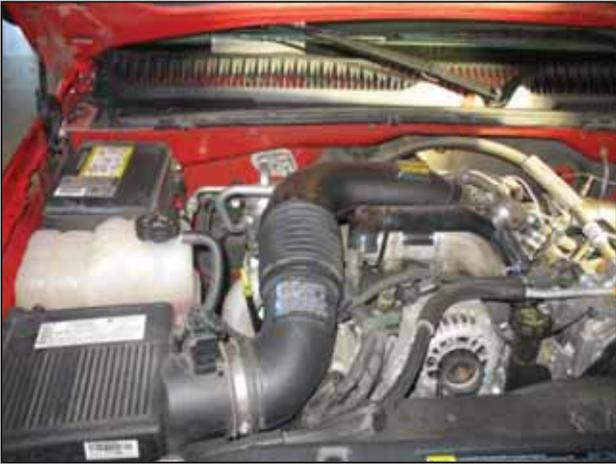
a. Factory air box system installed.
