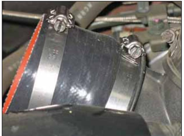
e. Install the straight coupler onto the turbo inlet hose and secure using two supplied #56 hose clamps as shown.
