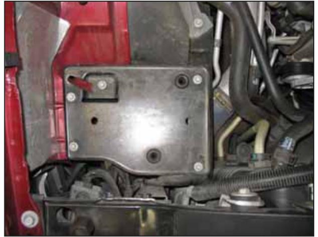
f. Remove the mounting plate for the air filter housing by removing the five bolts that secure it.
