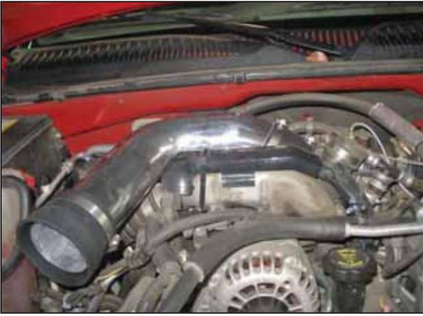
f. Install the upper intake pipe into the coupler on the turbo inlet. Slide the reducing coupler completely onto the intake pipe to allow room for the lower intake pipe to be positioned.
