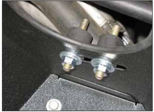
g. Install the two supplied rubber mounts into the slot on the heat shield. Secure each rubber mount with a washer and M8 nut. Secure the mounts with just enough slack for the mounts to slide in the slot.
