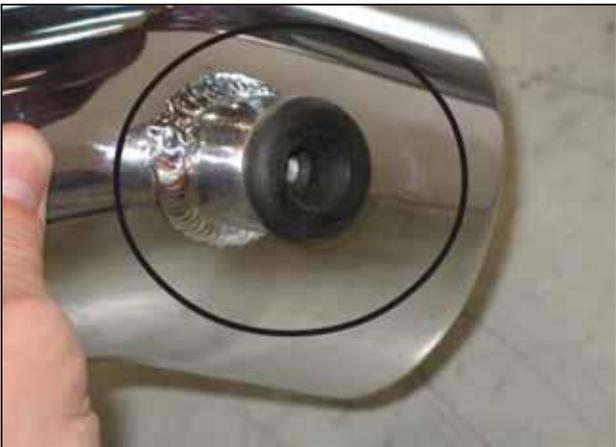
h. Install the rubber grommet into the nipple on the lower intake pipe as shown.
