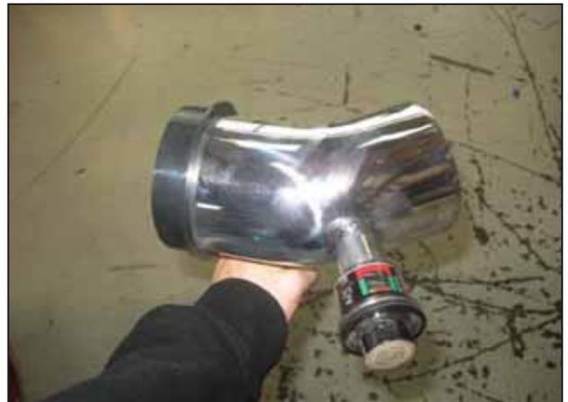
i. Install the previously removed air filter restriction gauge into the grommet installed in previous step. Also install the rubber filter adapter onto the filter end of the lower intake pipe.
