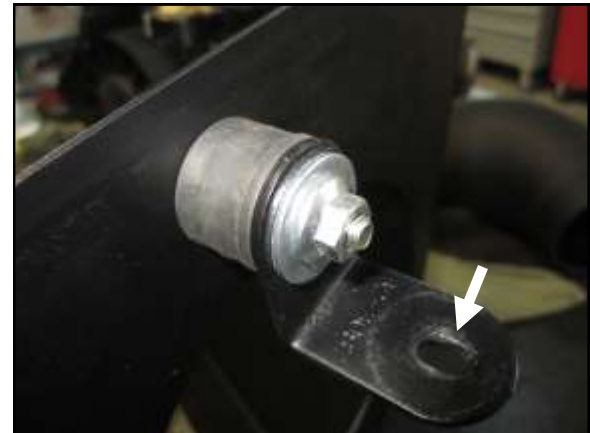
H. Install the "L" mounting bracket (R) onto the end of the rubber isolator mount using another flat washer (X) and M6 nut (U). Note that the slotted hole in the bracket is facing down. Leave the M6 nut loose for Step M.
