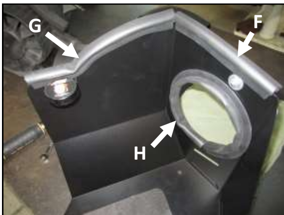
I. Install the longer bulb seal molding (H) around the inside of the large outlet hole in the heat shield. Trim any excess bulb seal. Then install the two shorter bulb seal moldings (F and G) along the top edge of the heat shield as shown.
