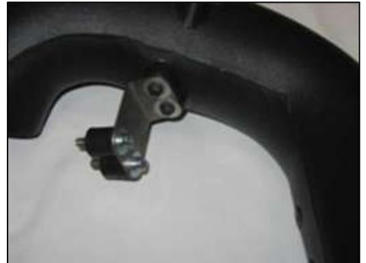
c. Install the intake tube bracket and rubber mounts onto the intake tube using the included bolts and washers. Do not over tighten.
