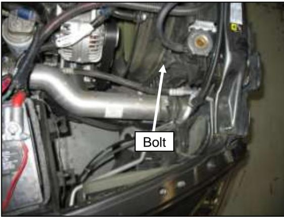
e. Remove the indicated bolt from the radiator fan shroud.
