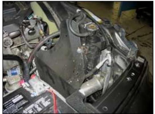
e. Install the heat shield into the engine bay, aligning the heat shield bracket with the exposed bolt hole on the radiator fan shroud. Secure the bracket with the factory bolt removed in step 2e. Secure the heat shield tab to the radiator support with the factory bolt removed in step 2d.
