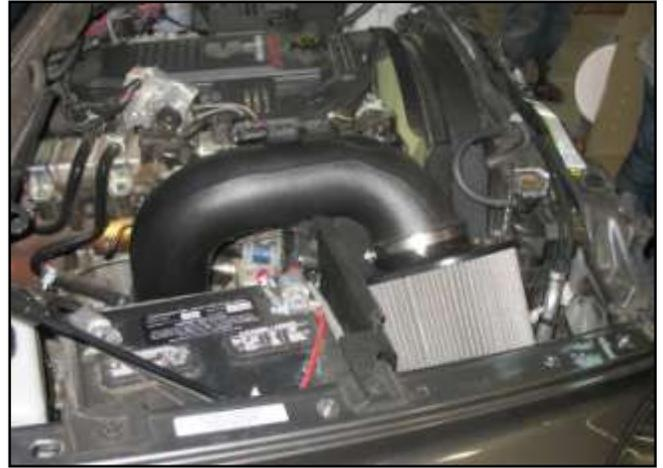
AEM® intake system installed
