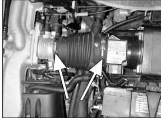
b. Loosen the hose clamps at both ends of the rubber intake tube. Remove the three vacuum lines from the rubber intake tube. When removing the vacuum lines, make sure the plastic nipples remain in each breather hose and not in the rubber intake tube. These components will be re-used with the AEM® intake system.
