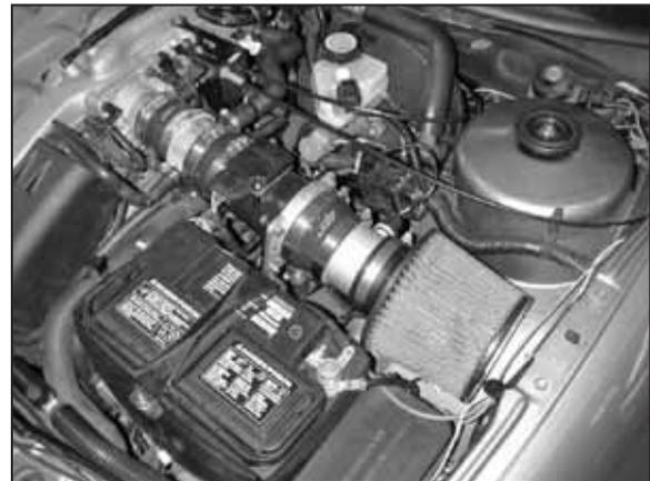
g. Install the AEM® air filter onto the end of the assembly. Position the inlet pipe for best fitment. Plug in the MAF sensor connector. Be sure that the pipe or any other components do not contact any part of the vehicle. Tighten the hose clamps and bracket bolt.
