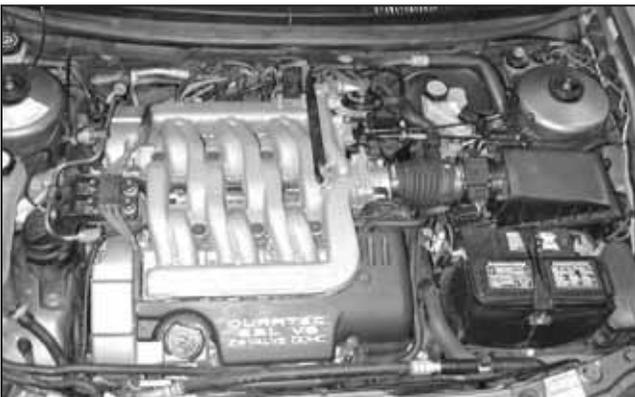
Stock air box system installed
