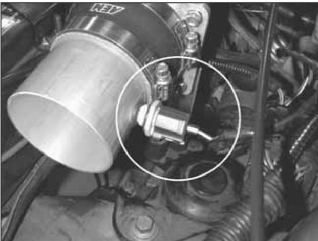
f. Insert the IAT sensor in the IAT grommet at the back of the AEM® inlet pipe '9.' Insert the sensor up to the barbs. Attempting to force the barbs past the grommet will cause the grommet to fall out of the pipe.
