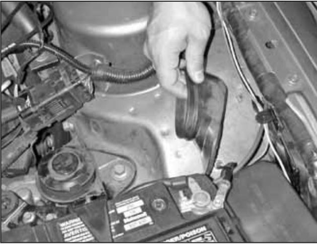
e. Remove rubber boot from the inner fender in front of the shock tower.
