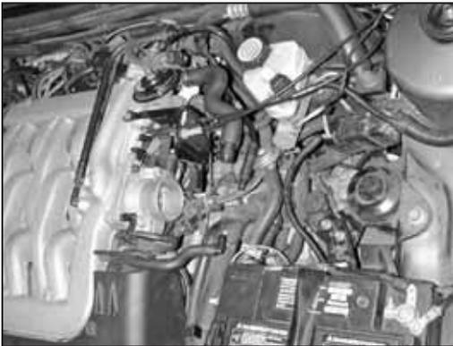
c. Remove the air box, MAF sensor, and rubber intake tube assembly from the vehicle.
