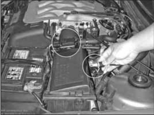
a. Twist the inlet air temperature (IAT) sensor and remove it from the back side of the air box. Unplug the mass air flow (MAF) sensor connector.
