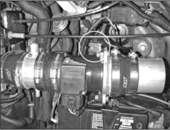
d. Place the AEM® intake assembly in the engine bay. The 2.50" coupler and hose clamp should be affixed to the throttle body. The bracket on the MAF sensor will line up with the rear-most rubber mount where the air box mounting bracket used to be attached. Use one of the stock bolts to attach the bracket to this mount.
