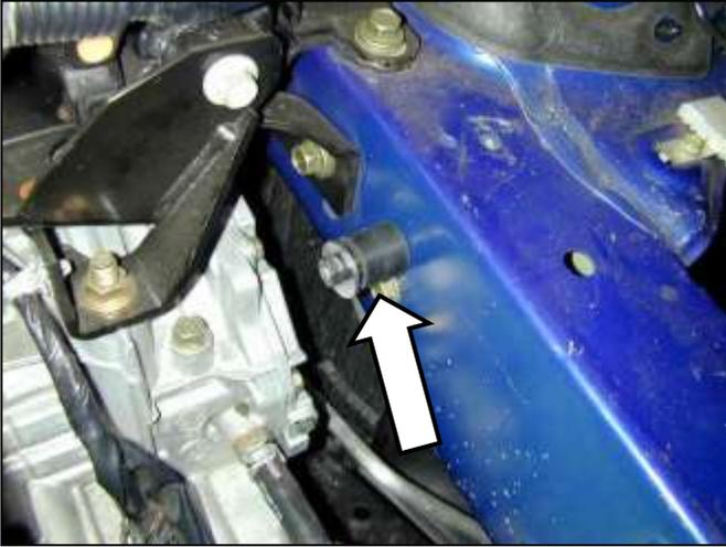
h. Install supplied rubber mount as shown.
