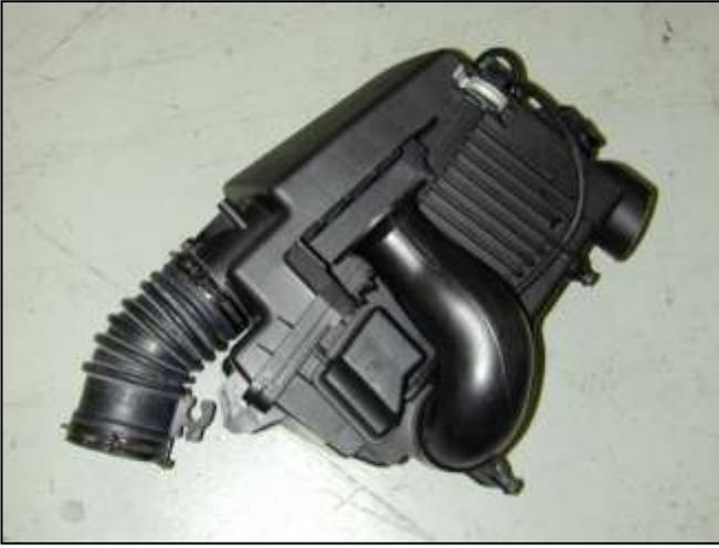
g. Pull the air box up and out of the engine bay.
