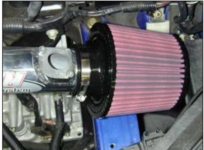
l. Install the air filter onto the end of the pipe.
