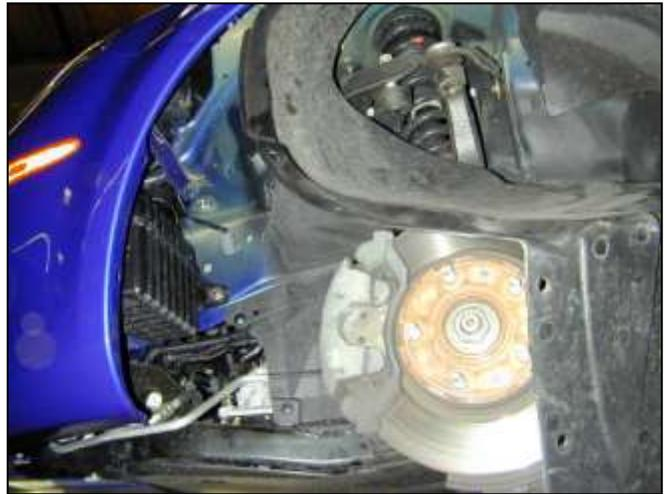
l. Place the fender liner as shown.
