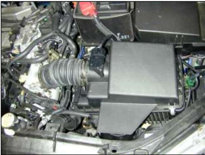
a. Stock air box system installed.
