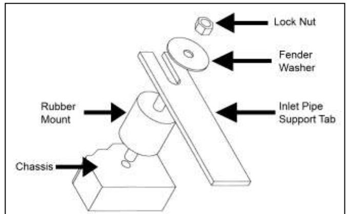
Proper installation of rubber mount assembly.
