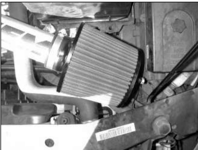
h. Ensure there is enough clearance around the air filter. Once proper fitment is achieved secure the air filter. Secure the intake bracket to the rubber mount installed in step 3c with a washer and nyloc nut. Refer to diagram for proper installation of rubber mount assembly.
