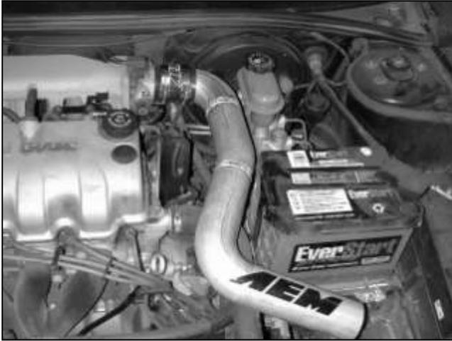
b. Insert intake pipe with provided coupler and hose clamps.
