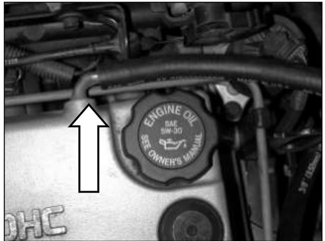
e. Attach breather hose to crank case with provided clamp.
