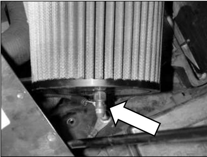
f. Attach the air filter element to the end of the inlet pipe. Insert the IAT into the air filter. Make sure the sensor is snug.
