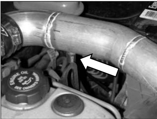
d. Attach breather hose to inlet pipe with provided clamp.
