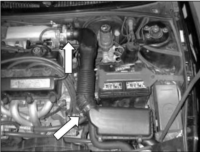
a. Snap open the clips on the throttle body and the air box. They should lock open.
