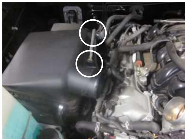
d. Disconnect the mass air flow sensor connector and the retaining clip from the air box.
