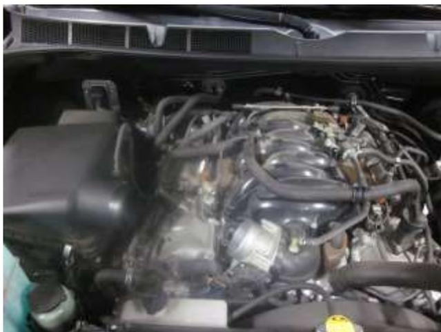
c. Remove the stock intake tube. **Note:** Do not discard your stock equipment.
