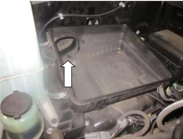
c. Install the lower air box into the vehicle by squeezing the air accelerator and inserting it into the fender opening in the vehicle. **Note:** it 's easier to have the air box lid and base separated to perform this step.
