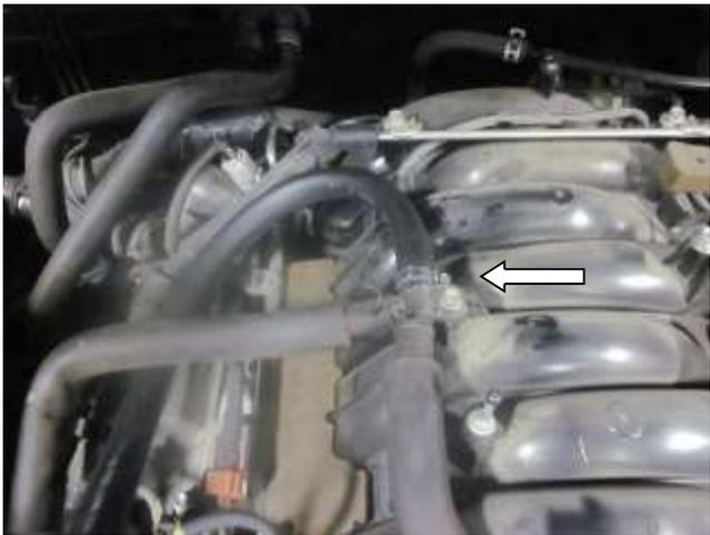
h. Route the hose (5-7022) as shown and install on the "T" fitting and tighten provided hose clamp (08411).
