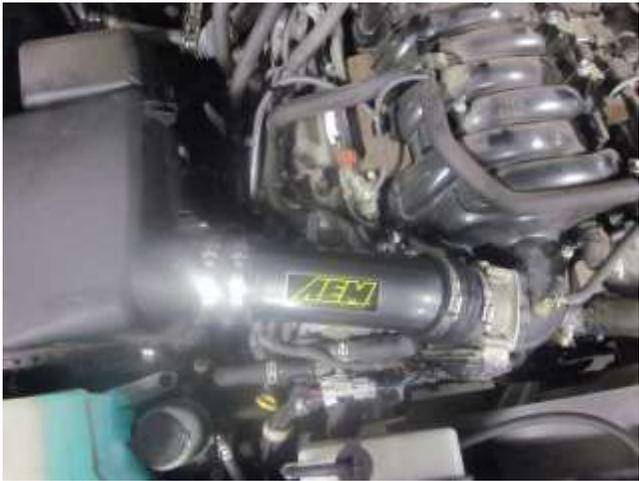
f. Lift the air box slightly and slide the AEM intake into the throttle body hose, then the air box hose while lowering the air box over the mount installed in 3b. Tighten all four hose clamps at this point.
