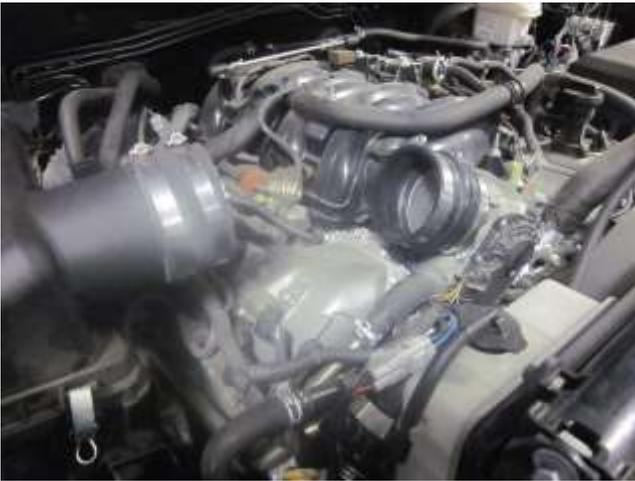
e. Slide the provided hose (5-1086) with the hose clamps (9456) onto the air box. Slide the provided hump hose (08657) with the hose clamps (9456 & 9452) over the throttle body.
