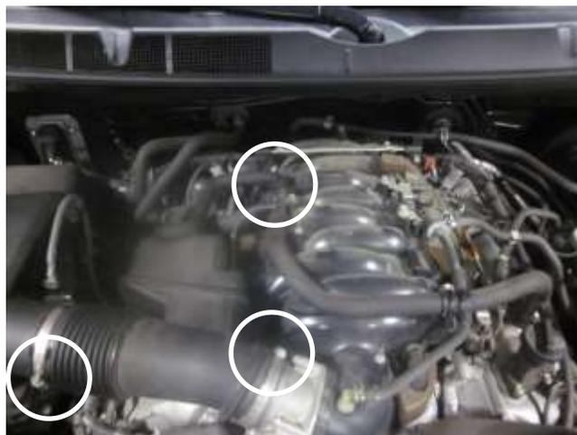
b. Loosen the hose clamp at the throttle body and the air box. Disconnect the small vacuum line on the intake resonator and the large vacuum line at the "T" above the intake manifold.
