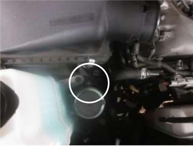
e. Loosen and remove the M6 bolts securing the air box to the vehicle. **Note:** One of the bolts is on the backside of the air box (not shown). One of the bolts will be re-used.
