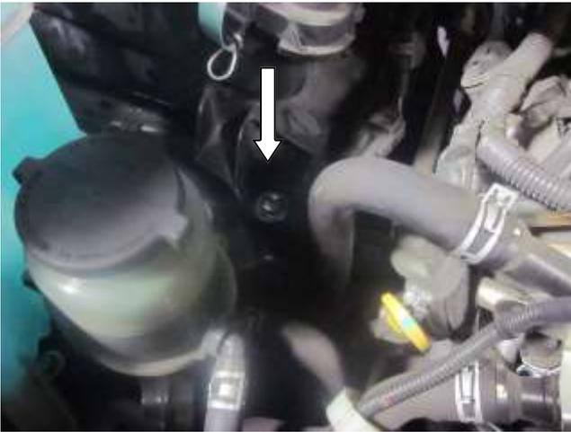
i. Make sure air box is sitting on the previously installed mount and install the washer (559960) and nut (444.460.04) and tighten. Also re-install and tighten the backside bolt that was removed in step 2e.
