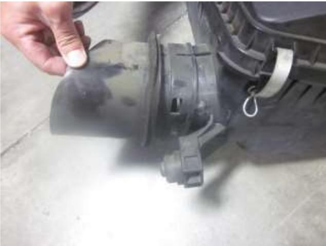
g. Disconnect the stock air inlet from the air box.
