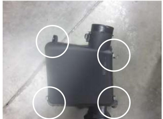
h. Unlatch the 4 clips holding the upper air box to the lower air box and remove the stock filter.
