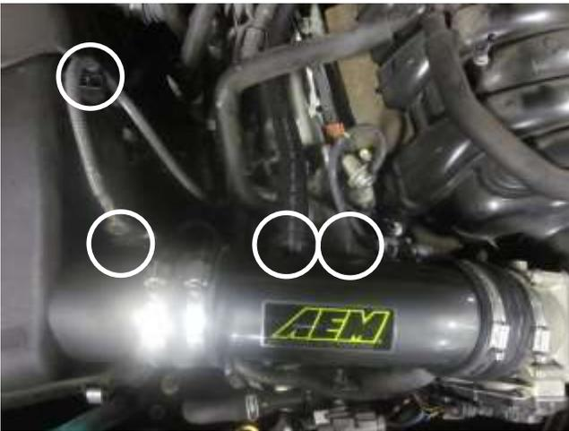
g. Re-clip the mass air flow sensor harness to the sensor. Re-attach the small vacuum line back onto the AEM intake tube. Install the provided hose (5-7022) onto the AEM intake tube.
