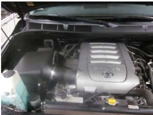
a. Remove the engine cover by pulling up and out.
