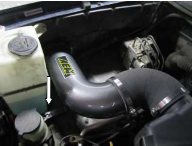
g. Install the intake tube into the accelerator first then, slide the coupler over the air box inlet. The bracket should line up to the rubber mount as well.
