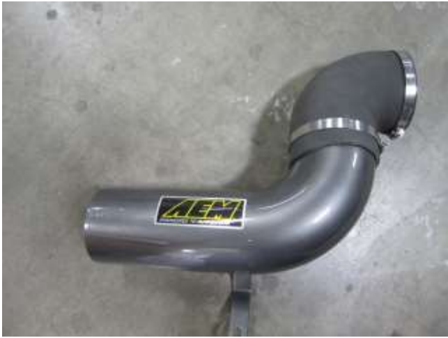
f. Install the 90 degree coupler onto the intake tube with the supplied hose clamps. Do not tighten at this time.
