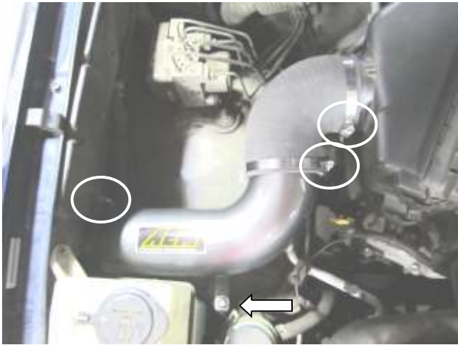
h. Install the M8 washer and nut onto the rubber mount securing the tube. After proper tube orientation has been achieved tighten all three hose clamps.
