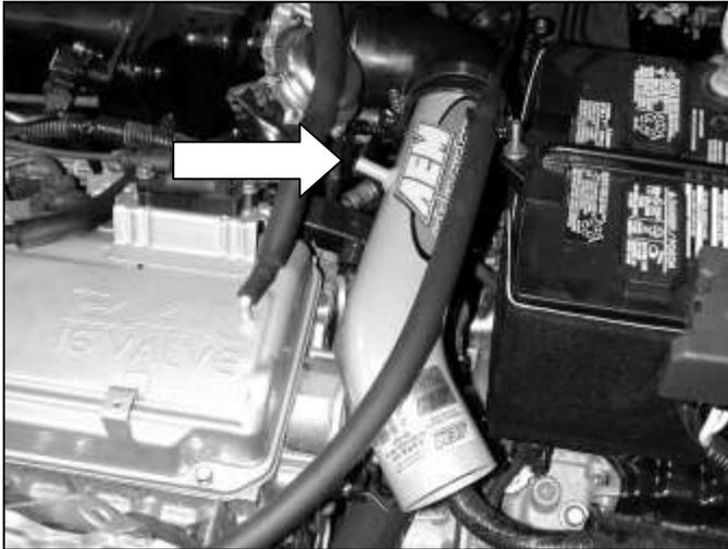
e. Insert the upper AEM® intake pipe into the rubber elbow. Ensure that the nipple of the intake pipe is facing the valve cover.
