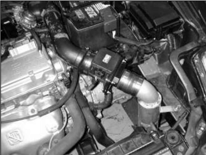
k. Install the air filter onto the lower end of the intake pipe. Once proper fitment and clearance is achieved secure the air filter with the supplied hose clamp.
