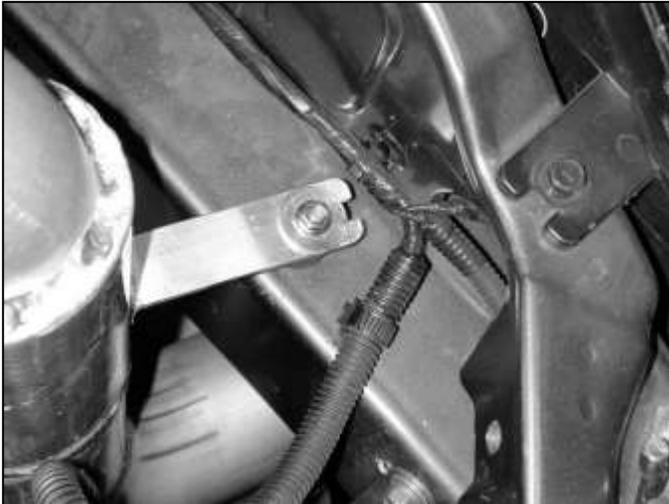
i. Install the rubber mount into the frame of the vehicle as shown. Align the lower intake pipe's bracket with the rubber mount and secure with a washer and lock nut. Do not completely tighten the lock nut. Refer to the diagram below to reference the proper installation of the rubber mount assembly.
