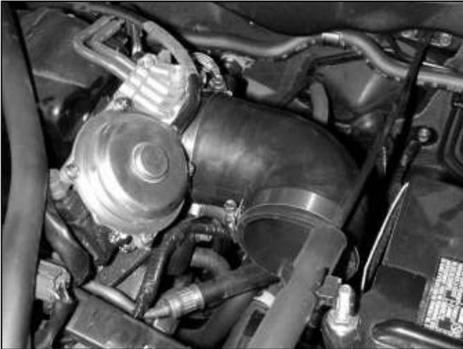
d. Place the rubber elbow with two hose clamps onto the throttle body. The longer end attaches to the throttle body.
