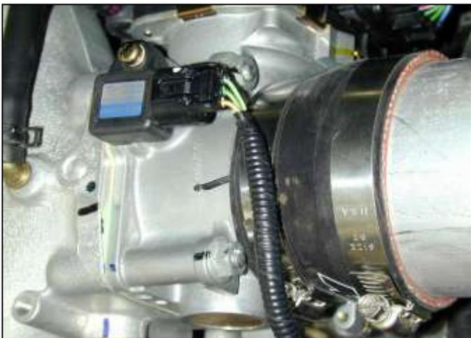
f. Install the silicone coupler over the throttle body and hose clamps but do not tighten hose clamps.
