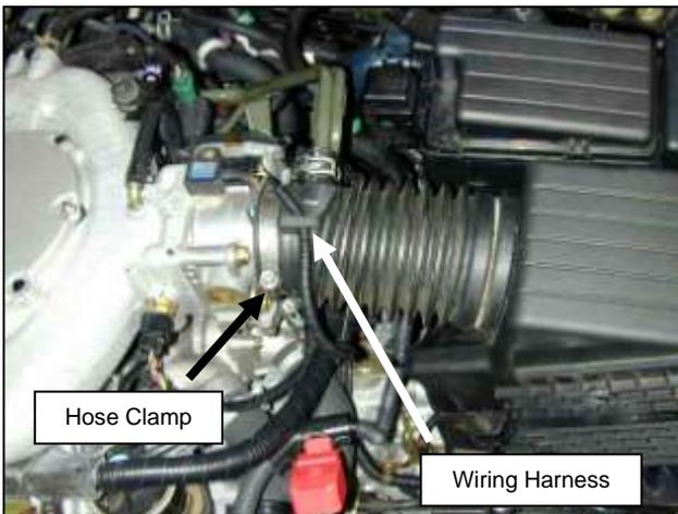
e. Loosen the hose clamp on the throttle body and unhook the wiring harness.
