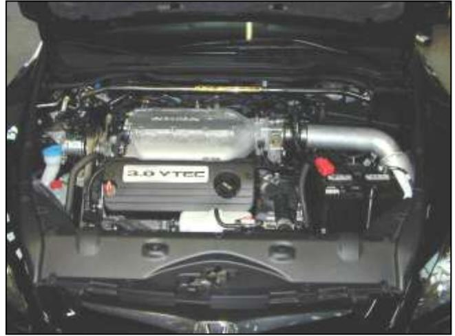
k. Check that the filter is not touching any part of the vehicle. Position the AEM® intake for best fitment. Be sure that the pipe or any other component is not in contact with any part of the vehicle. Tighten the hose clamps at the throttle body and silicone coupling. Tighten the nut on the mounting bracket. Re-adjust pipe if necessary.
