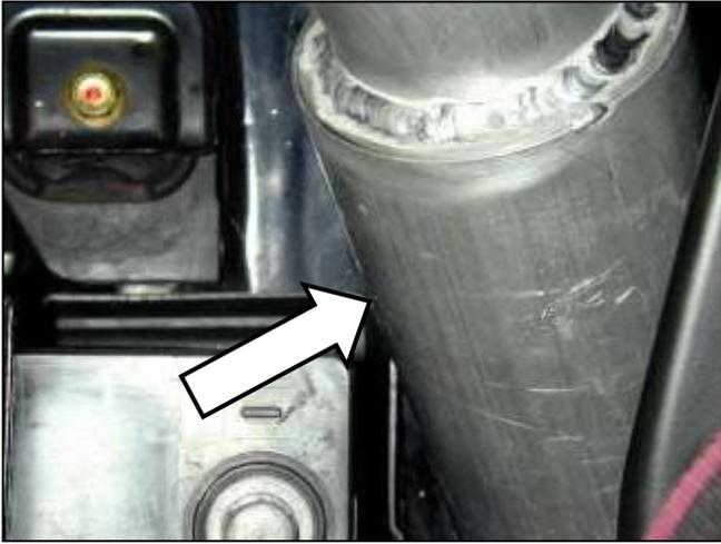
j. Reinstall the plastic battery under-tray, the battery, and the battery tie down bracket. Do not install the plastic battery cover. Check for proper clearance between the battery and the intake pipe. Use the supplied zip-ties to make sure no wires are in contact with the intake system.
