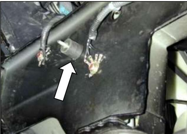
d. Install the rubber mount where the factory ground block was removed.
