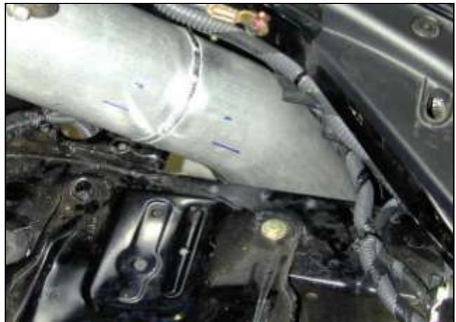
e. Install the AEM® intake pipe by routing the filter (large) end of the pipe through the opening in the engine bay between the battery location and the fender. Be sure to have the mounting bracket on the intake facing the front of the car and use rags to prevent the pipe from being scratched.
