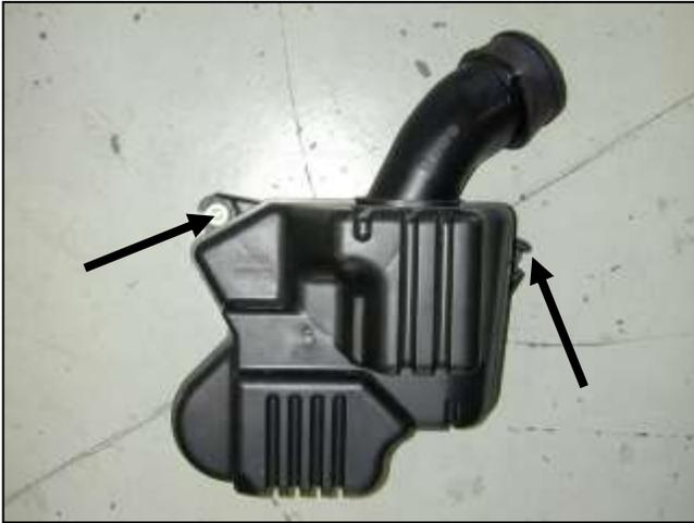
k. On automatic transmission equipped cars the stock intake resonator looks like the one pictured above. Remove the two bolts holding it in place. **NOTE: The second bolt is located on the top front side of the resonator.**
