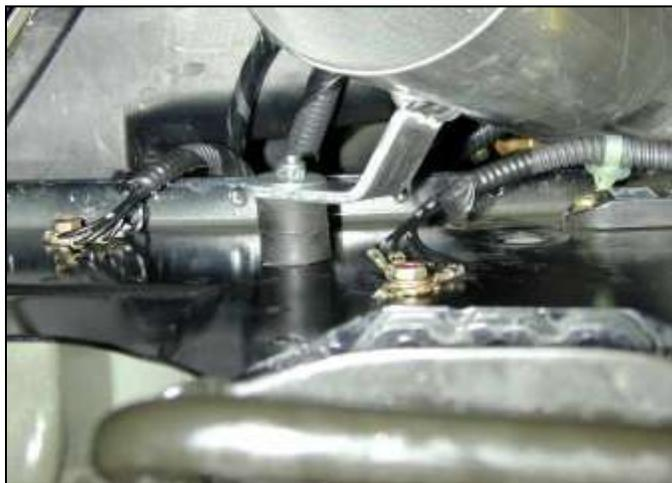
g. Guide the bracket on the intake pipe over the stud on the rubber mount. Once aligned, install the supplied washer and nut onto the stud. Do not tighten until fitment is complete.
