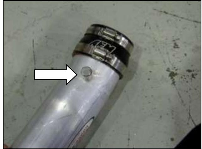
c. Check to see that the inside of the AEM® inlet pipe and air filter are clean and free from any foreign objects and/or obstructions. Install the 3" silicone coupler over the throttle body end of the intake pipe using the #48 hose clamps. Install the hex head plug and o-ring into the threaded nipple as shown.
