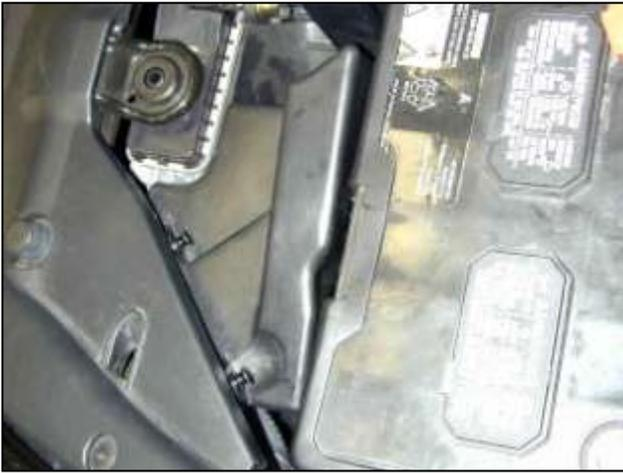
c. Remove the plastic shielding in front of the battery by pulling the two plastic snaps out and lifting straight up on the shield.
