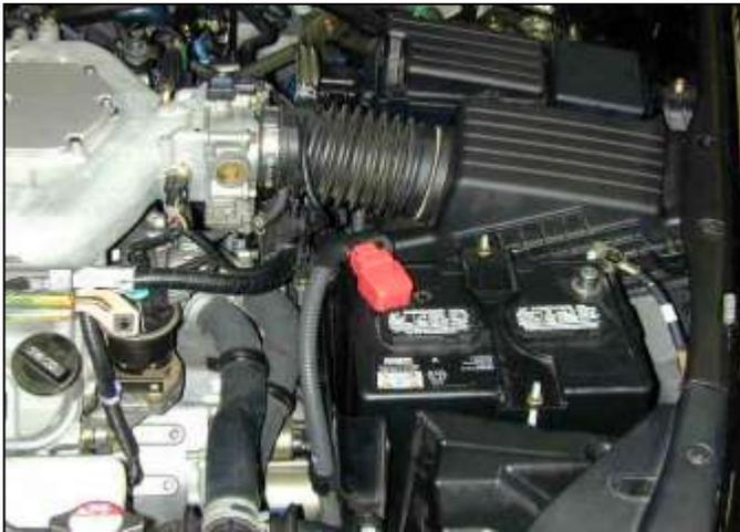
Factory air box system installed
